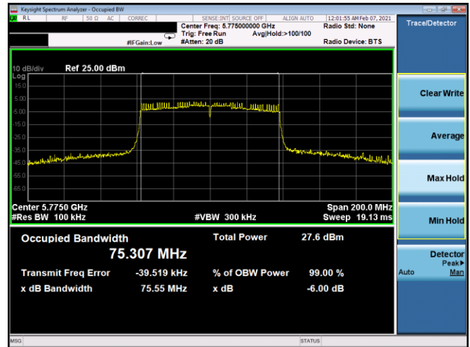
Plot 7-131. 6dB BW & 99% OBW Antenna 4b (80MHz BW 802.11ac – Ch. 155, MCS0)
