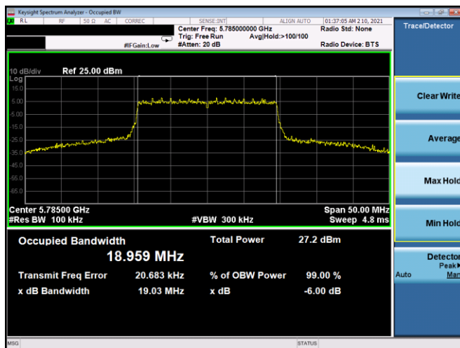
Plot 7-134. 6dB BW & 99% OBW Antenna 5b (20MHz BW 802.11ax(SU) – Ch. 157, MCS3)
