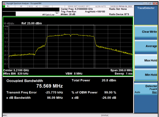
Plot 7-77. 26dB BW & 99% OBW Antenna 4b (80MHz BW 802.11ac – Ch. 42, MCS3)
