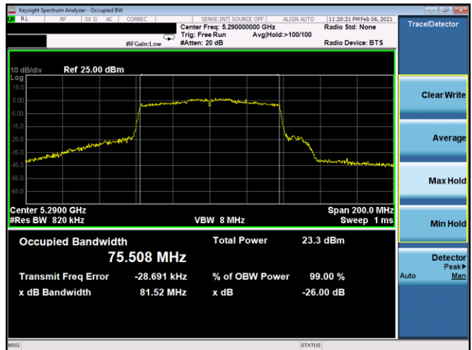
Plot 7-83. 26dB BW & 99% OBW Antenna 4b (80MHz BW 802.11ac – Ch. 58, MCS3)
