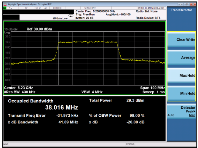
Plot 7-58. 26dB BW & 99% OBW Antenna 4b (40MHz BW 802.11ax(SU) – Ch. 46, MCS0)
