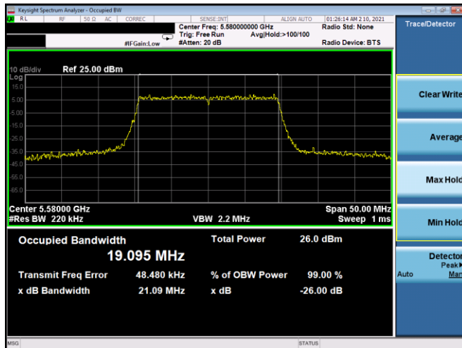
Plot 7-68. 26dB BW & 99% OBW Antenna 4b (20MHz BW 802.11ax(SU) – Ch. 116, MCS0)
