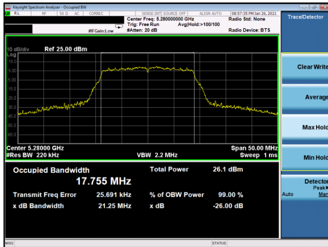
Plot 7-7. 26dB BW & 99% OBW Antenna 5b (20MHz BW 802.11n – Ch. 56, MCS0)
