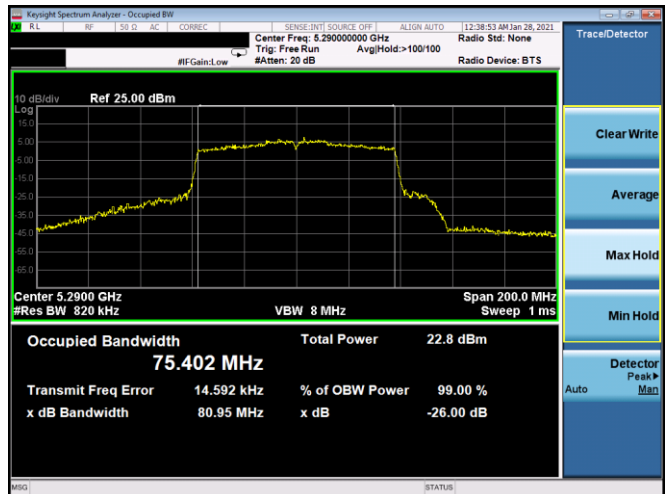
Plot 7-29. 26dB BW & 99% OBW Antenna 5b (80MHz BW 802.11ac – Ch. 58, MCS3)
