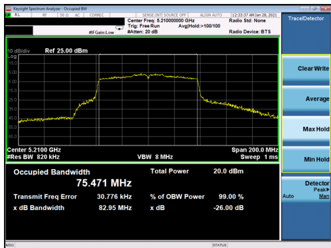
Plot 7-5. 26dB BW & 99% OBW Antenna 5b (80MHz BW 802.11ac - Ch. 42, MCS0)
