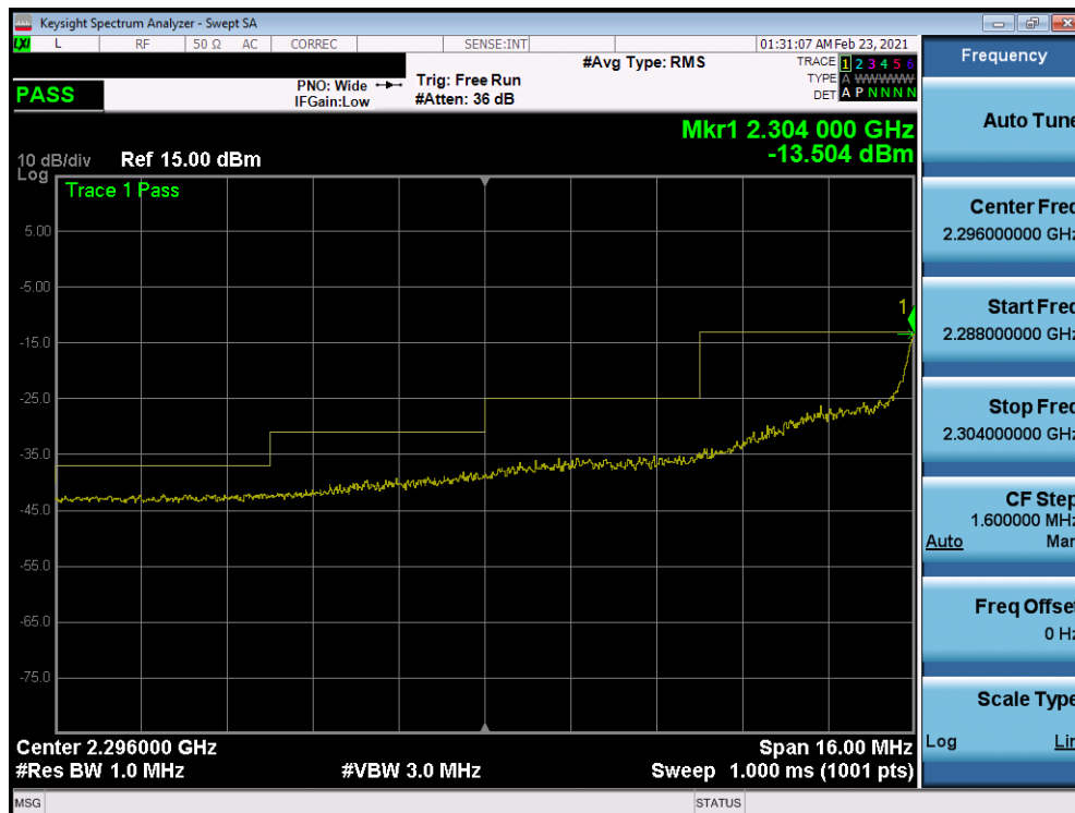
Plot 7-175. Lower Extended Band Edge Plot (Band 30 - 5.0MHz QPSK - Full RB Configuration)
