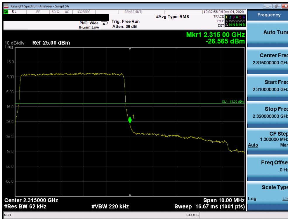
Plot 7-176. Upper Band Edge Plot (Band 30 - 5.0MHz QPSK - Full RB Configuration)
