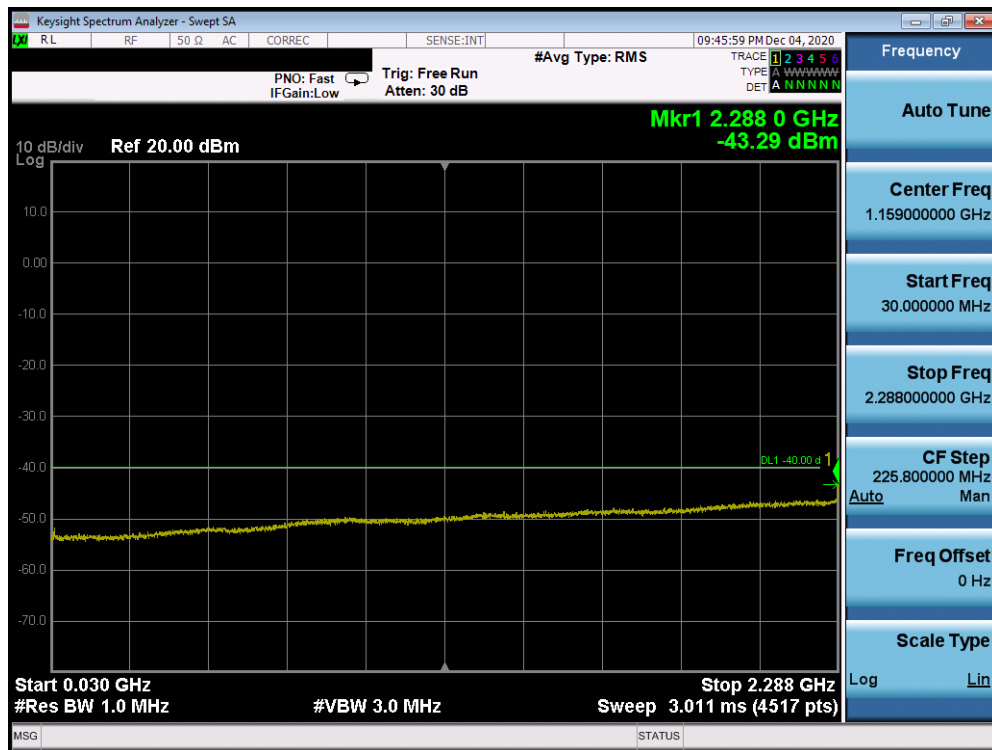
Plot 7-122. CSE (Band 30 - 10.0MHz QPSK - RB Size 1, RB Offset 0 - Mid Channel)
