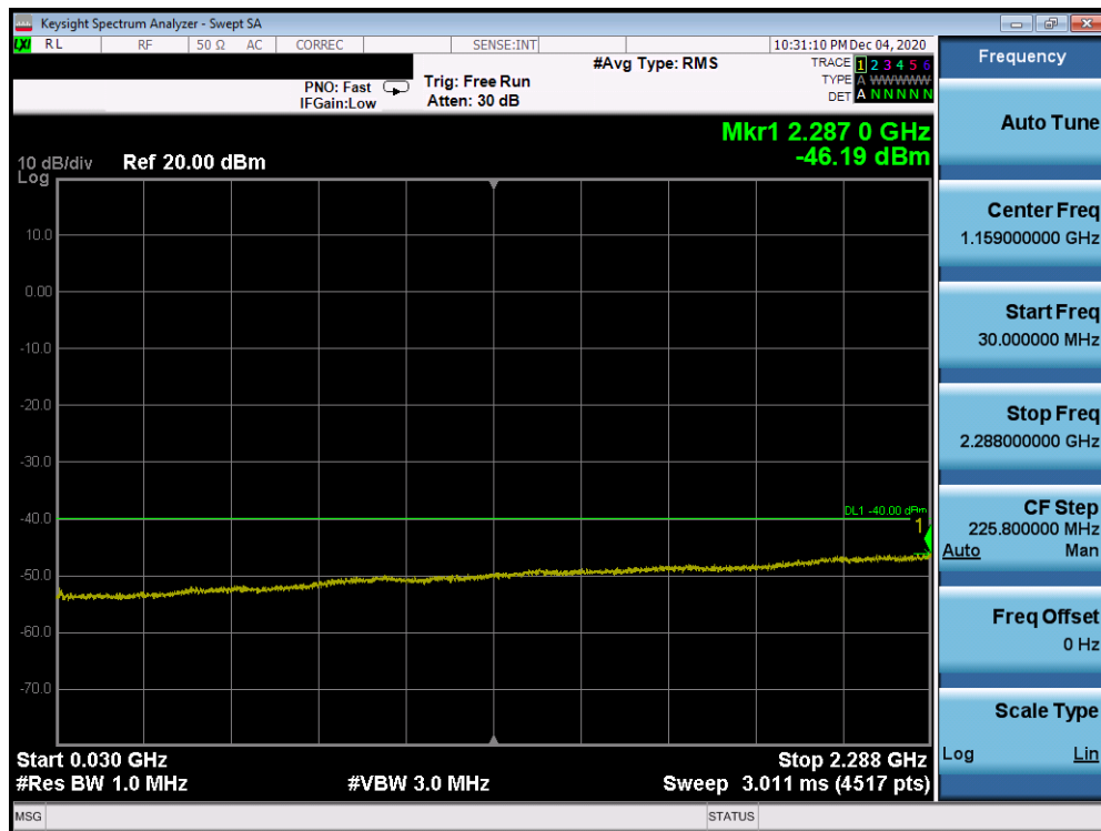
Plot 7-125. CSE (Band 30 - 5.0MHz QPSK - RB Size 1, RB Offset 0 - High Channel)
