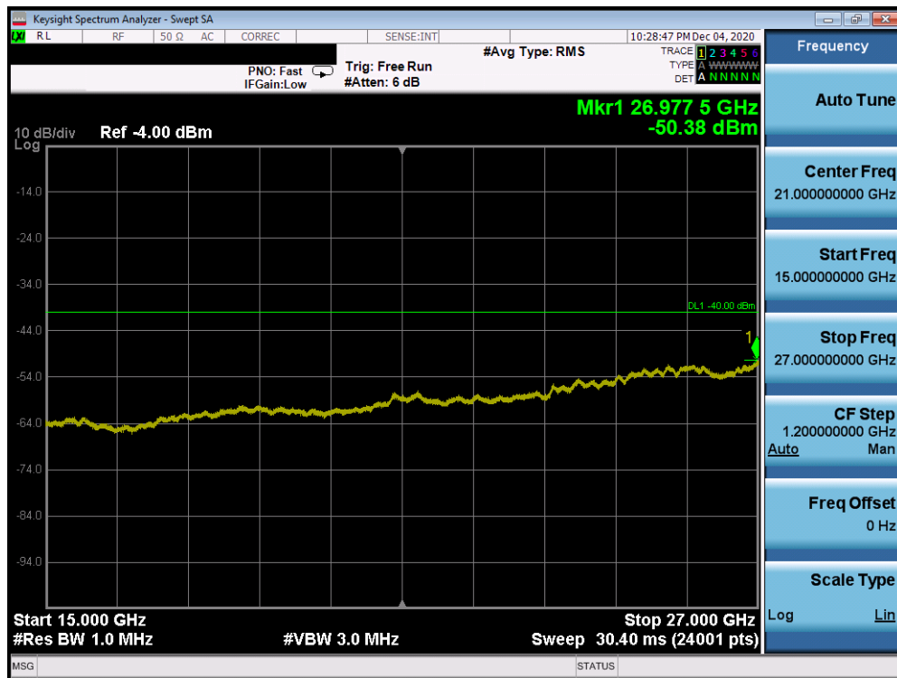
Plot 7-121. CSE (Band 30 - 5.0MHz QPSK - RB Size 1, RB Offset 0 - Low Channel)
