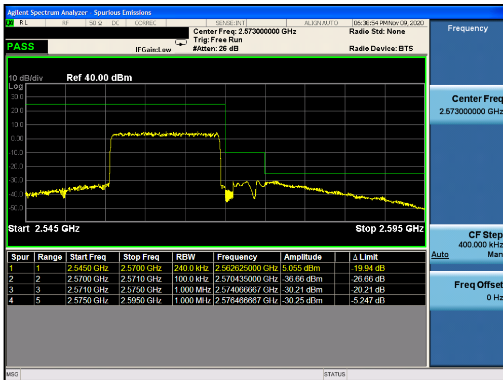
Plot 7-181. Upper ACP Plot (LTE Band 7 - 15MHz QPSK – Full RB Configuration)
