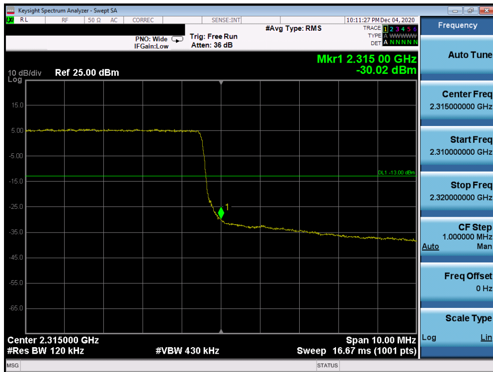
Plot 7-172. Upper Band Edge Plot (Band 30 - 10.0MHz QPSK - Full RB Configuration)
