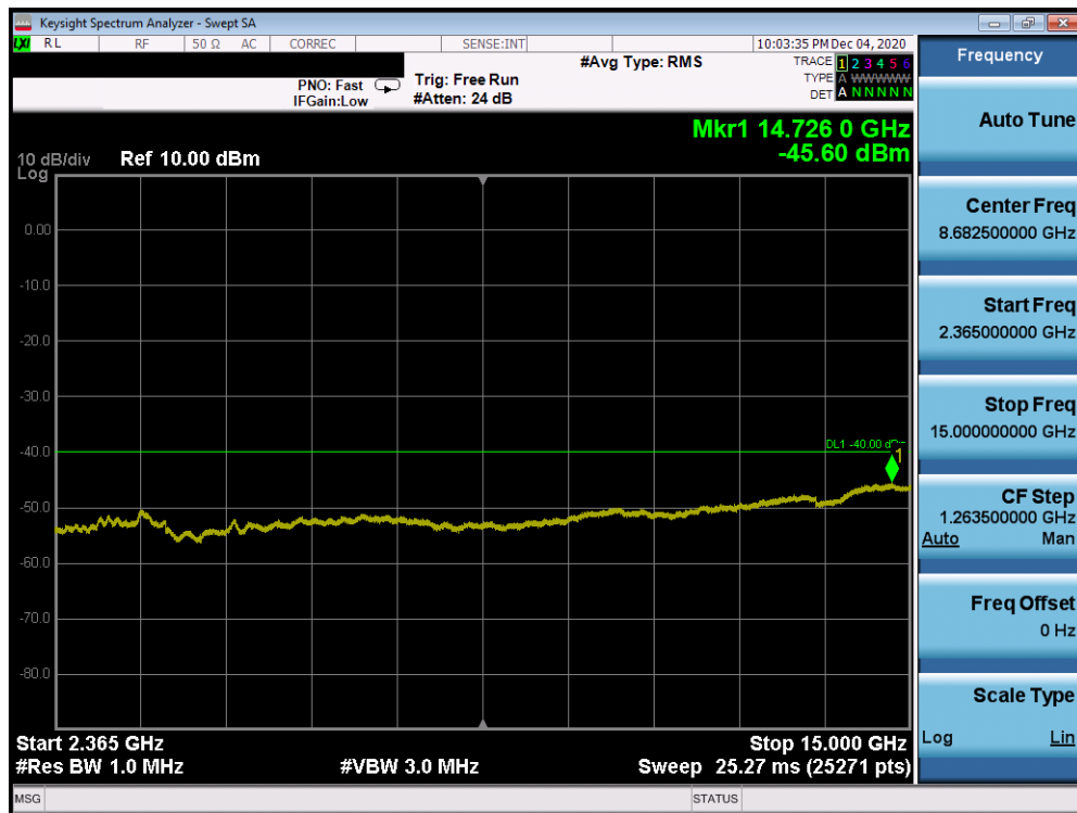
Plot 7-123. CSE (Band 30 - 10.0MHz QPSK - RB Size 1, RB Offset 0 - Mid Channel)
