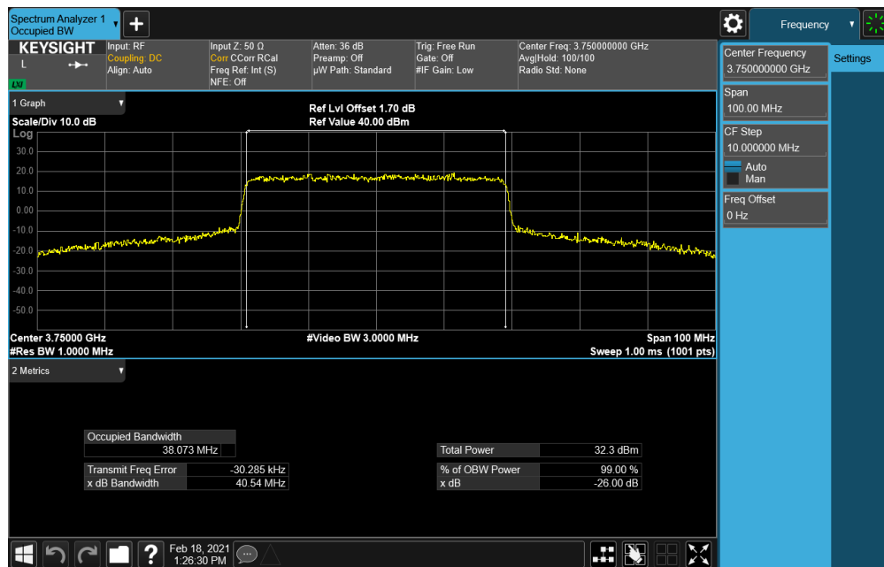
Plot 7-103. Occupied Bandwidth Plot (NR Band n77 - 40MHz CP-OFDM 16-QAM - Full RB Configuration)
