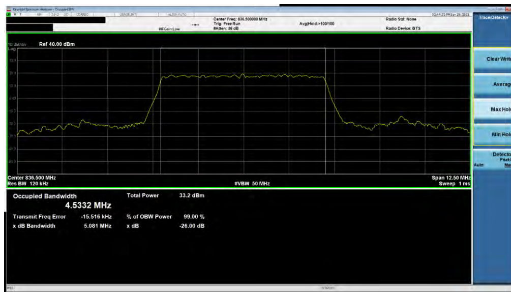
Plot 7-32. Occupied Bandwidth Plot (NR Band n5 - 5MHz DFT-s-OFDM \pi/2 BPSK - Full RB Configuration)
