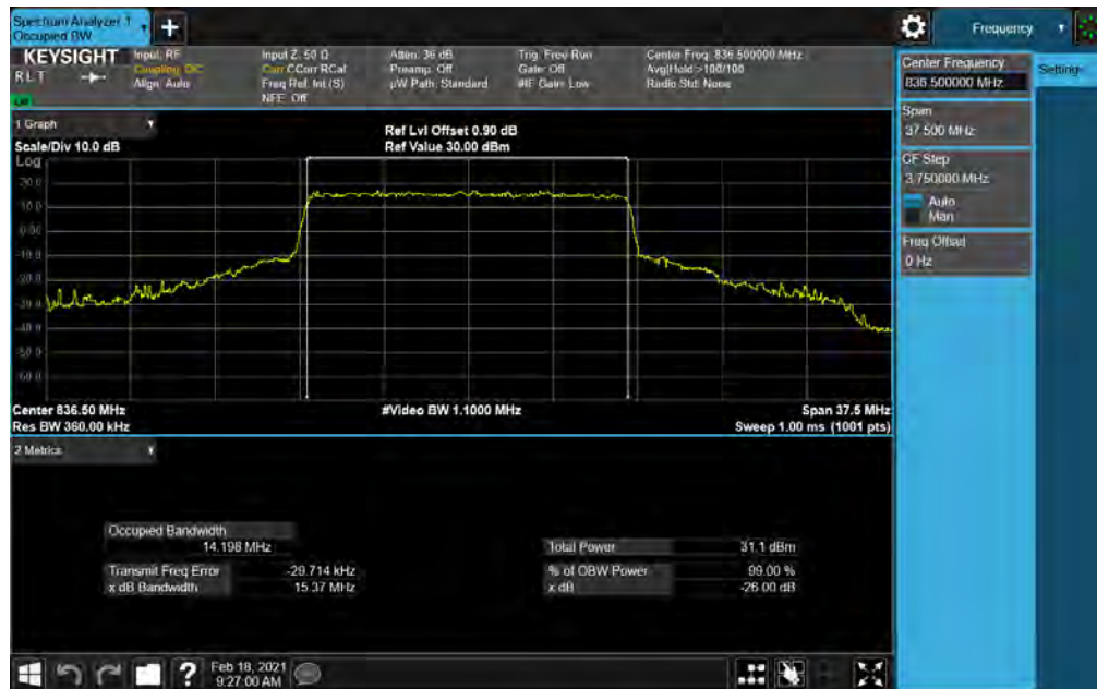
Plot 7-23. Occupied Bandwidth Plot (NR Band n5 - 15MHz CP-OFDM QPSK - Full RB Configuration)
