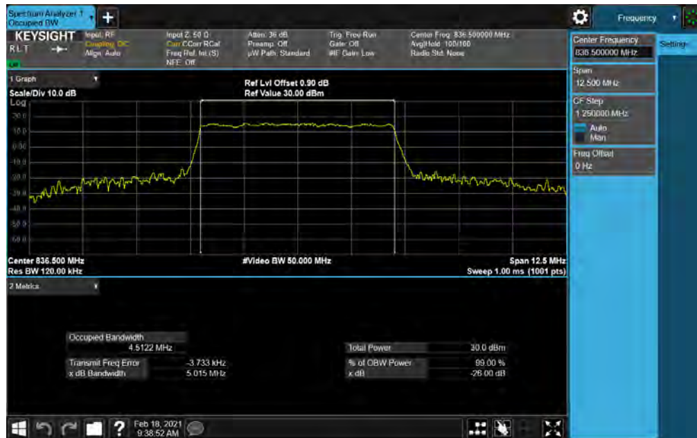
Plot 7-35. Occupied Bandwidth Plot (NR Band n5 - 5MHz CP-OFDM 64-QAM - Full RB Configuration)
