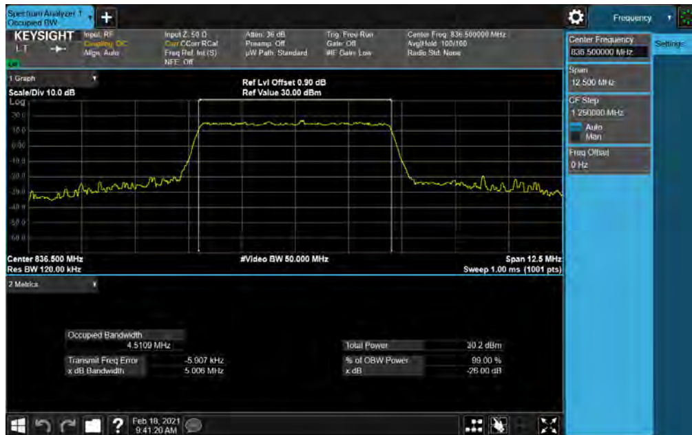
Plot 7-33. Occupied Bandwidth Plot (NR Band n5 - 5MHz CP-OFDM QPSK - Full RB Configuration)
