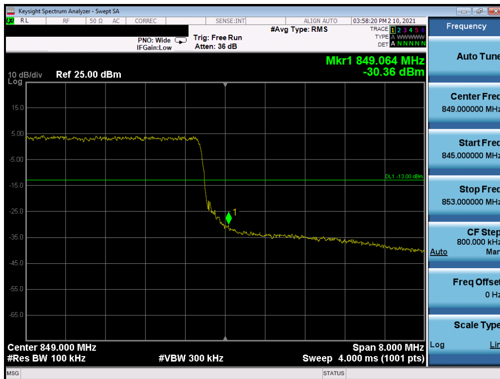
Plot 7-111. Upper BE Plot (ULCA LTE Band 5 - (10 + 10)MHz QPSK – Full RB Configuration)
