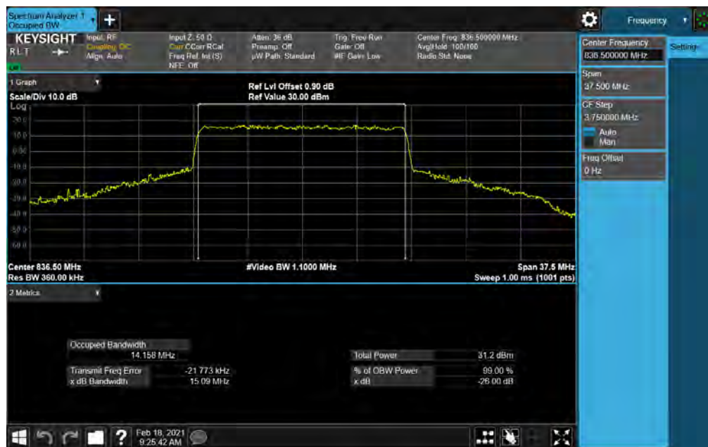
Plot 7-24. Occupied Bandwidth Plot (NR Band n5 - 15MHz CP-OFDM 16-QAM - Full RB Configuration)
