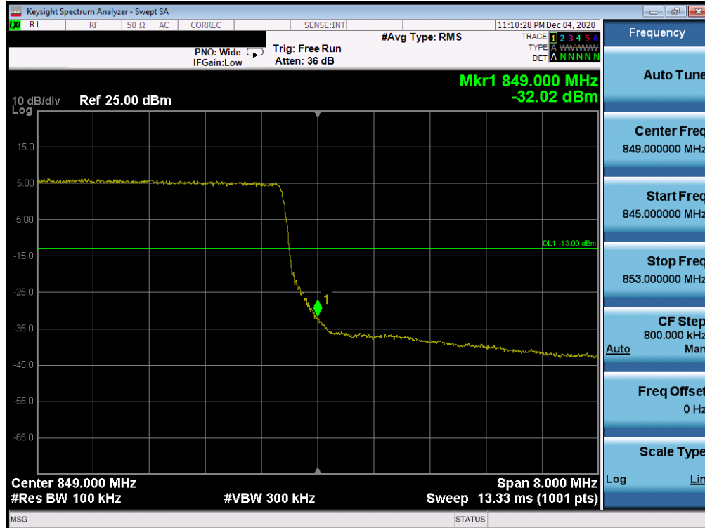
Plot 7-95. Upper Band Edge Plot (LTE Band 26/5 - 10MHz QPSK – Full RB Configuration)
