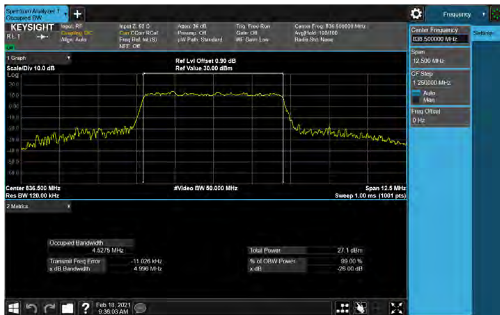
Plot 7-36. Occupied Bandwidth Plot (NR Band n5 - 5MHz CP-OFDM 256-QAM - Full RB Configuration)
