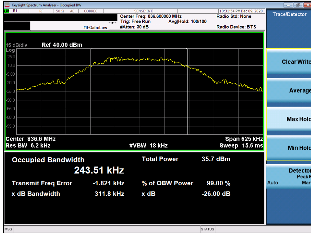
Plot 7-42. Occupied Bandwidth Plot (EDGE, Ch. 190)
