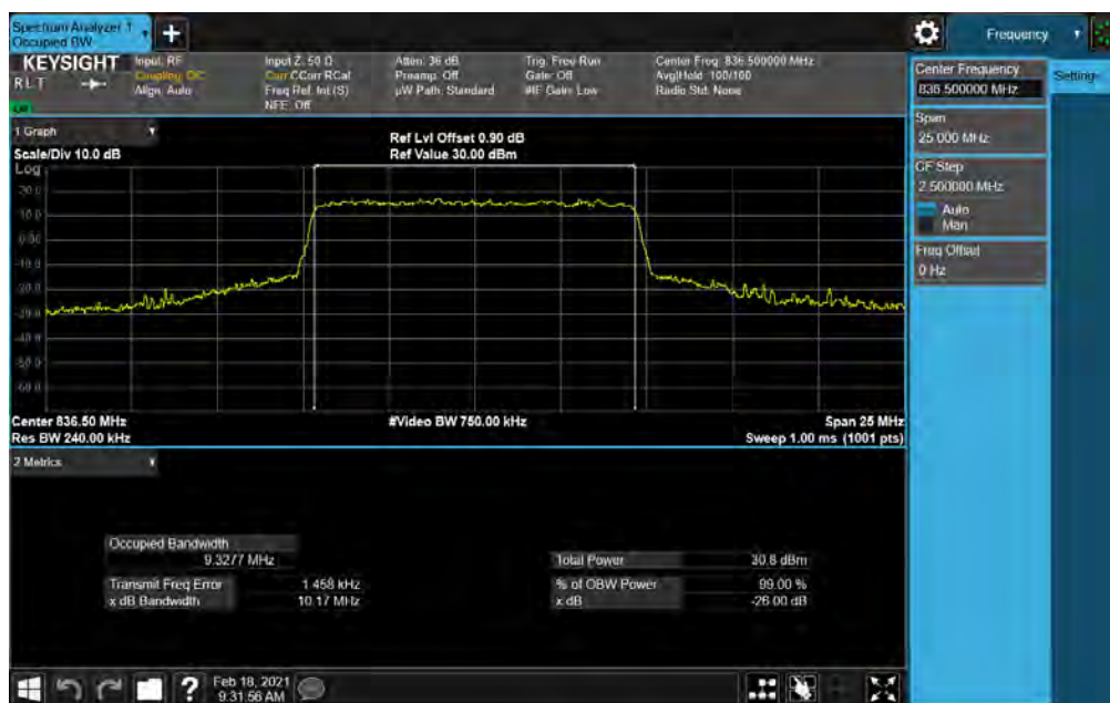
Plot 7-28. Occupied Bandwidth Plot (NR Band n5 - 10MHz CP-OFDM QPSK - Full RB Configuration)
