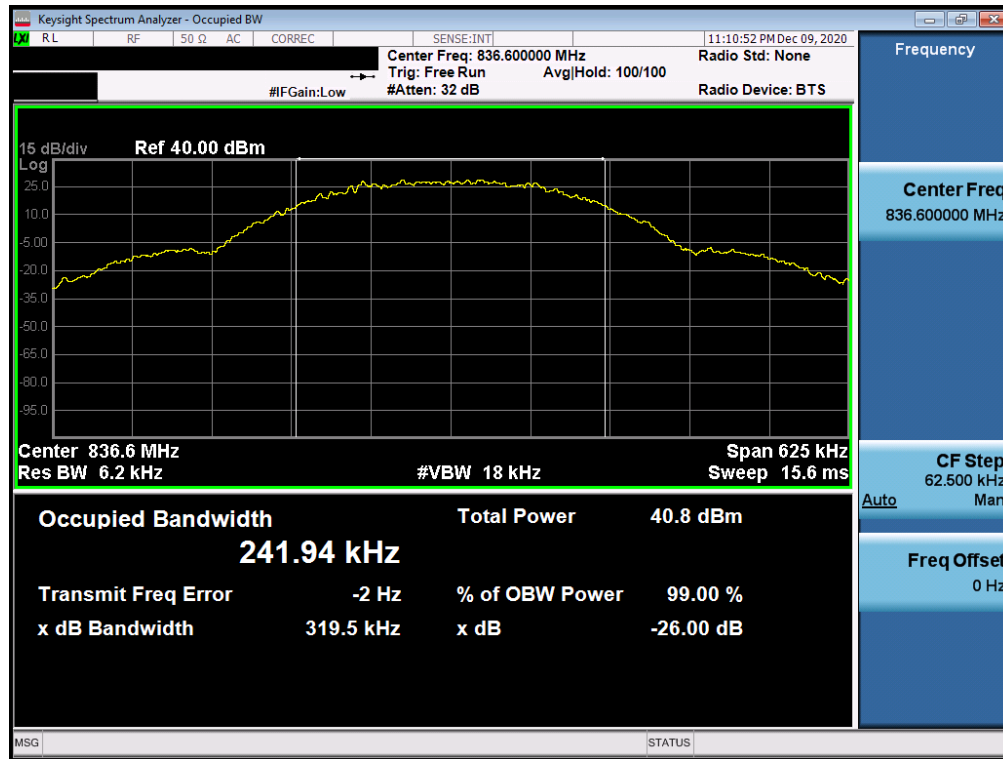
Plot 7-41. Occupied Bandwidth Plot (GPRS, Ch. 190)
