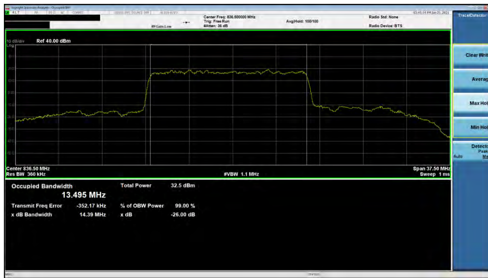
Plot 7-22. Occupied Bandwidth Plot (NR Band n5 - 15MHz DFT-s-OFDM \pi/2 BPSK - Full RB Configuration)
