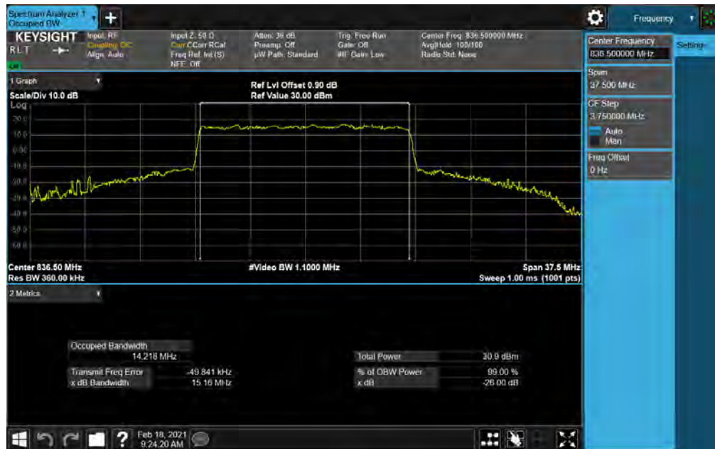
Plot 7-25. Occupied Bandwidth Plot (NR Band n5 - 15MHz CP-OFDM 64-QAM - Full RB Configuration)
