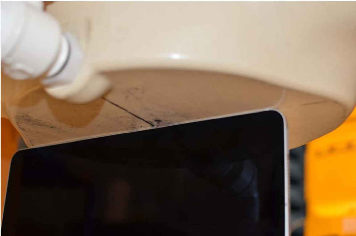
Test Setup Photo 9 – Right Edge Antenna 1, 2a, and 2b SAR at 0 mm
