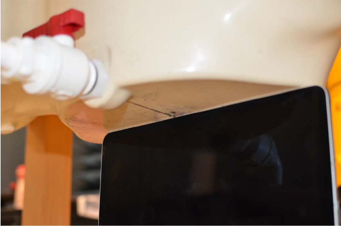
Test Setup Photo 10 – Left Edge Antenna 1, 2a, and 2b SAR at 0 mm
