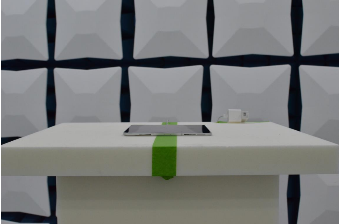
Figure 1: 1-18GHz Test Setup (Front View)
