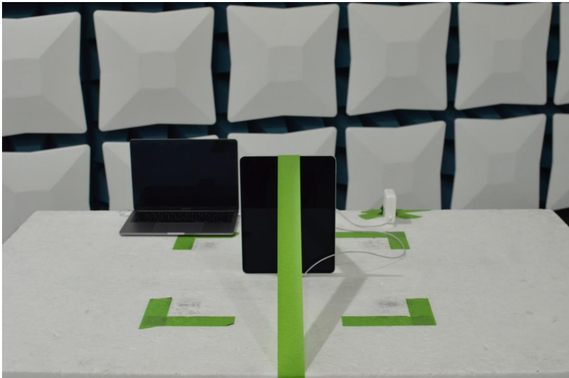
Figure 17: 30MHz-1GHz Test Setup (Front View)
