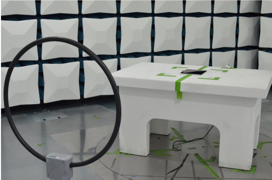
Figure 19: 9kHz-30MHz Test Setup (Front View)
