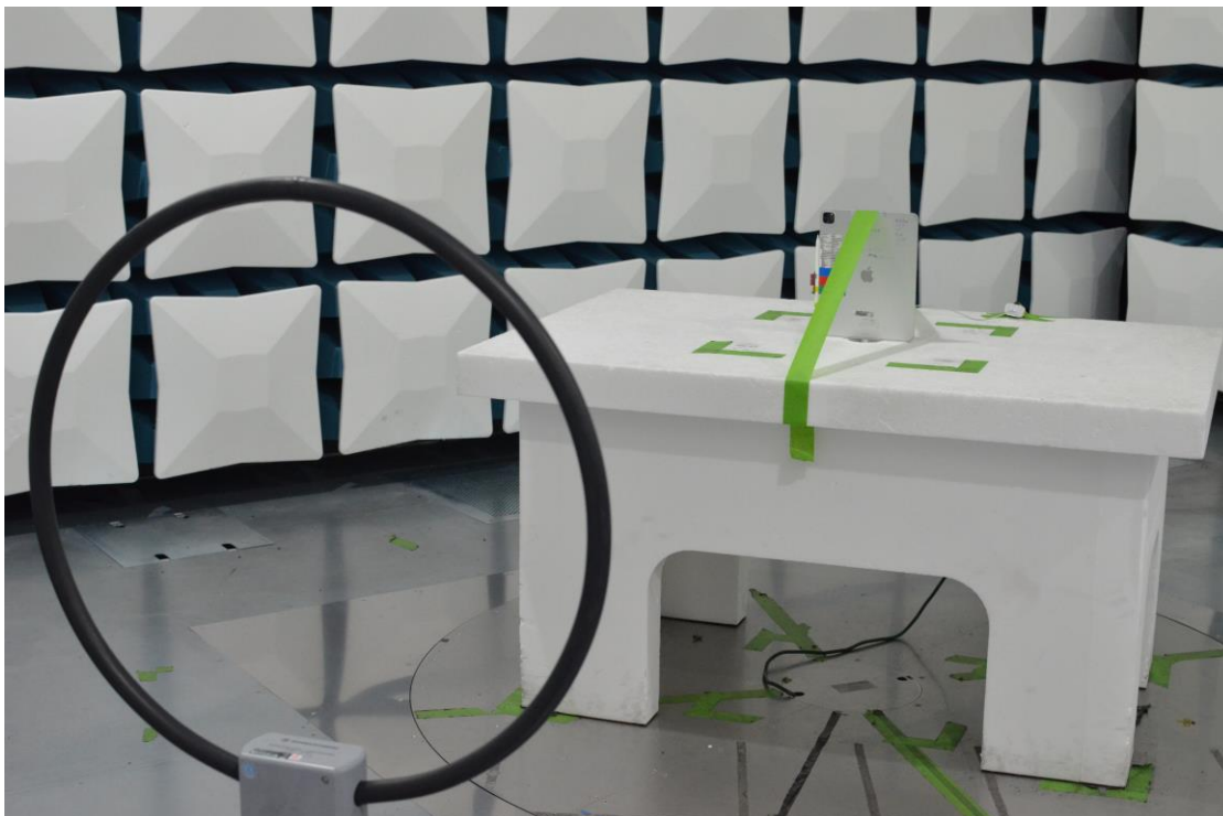
Figure 21: 9kHz-30MHz Test Setup (Front View)
