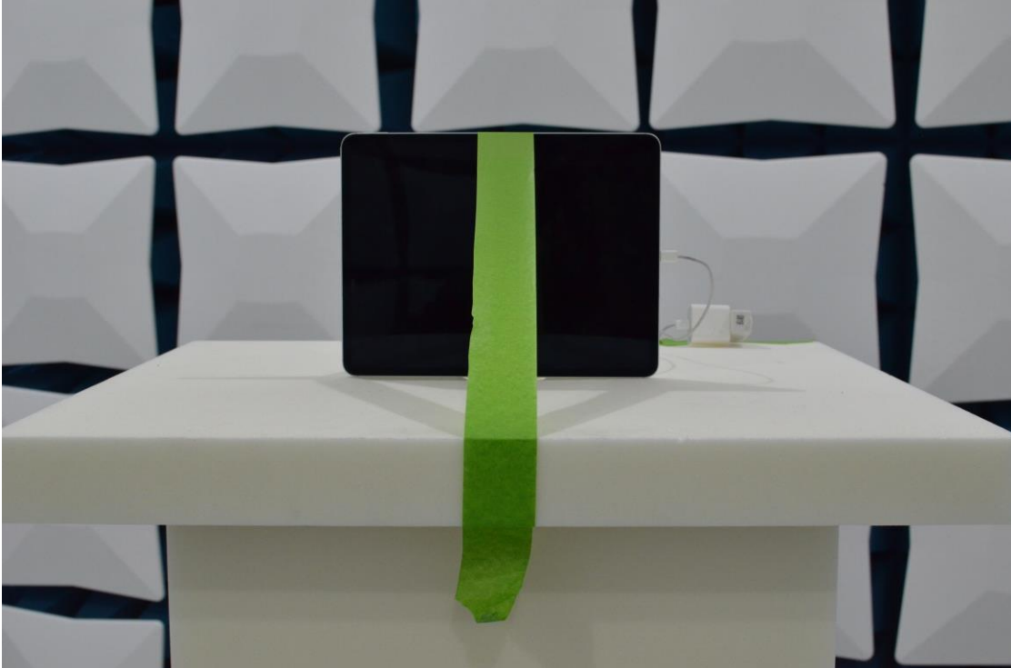
Figure 3: 1-18GHz Test Setup (Front View)
