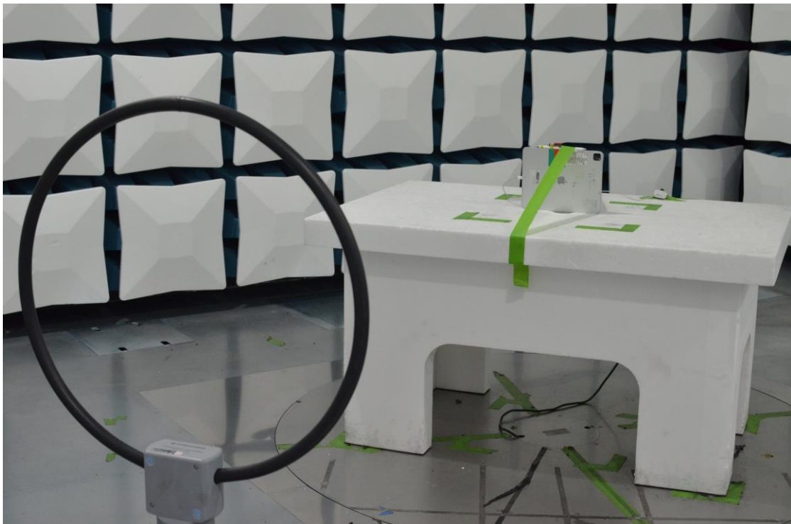
Figure 20: 9kHz-30MHz Test Setup (Front View)
