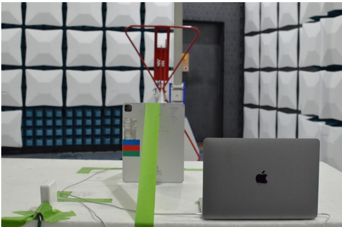
Figure 18: 30MHz-1GHz Test Setup (Rear View)
