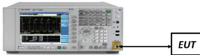
Figure 7-4. Test Instrument & Measurement Setup
