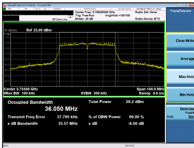
Plot 7-129. 6dB BW & 99% OBW Antenna 5B (40MHz BW 802.11n – Ch. 151, MCS0)
