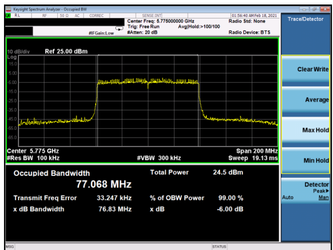
Plot 7-114. 6dB BW & 99% OBW Antenna 5T (80MHz BW 802.11ax(SU) - Ch. 155, MCS0)
