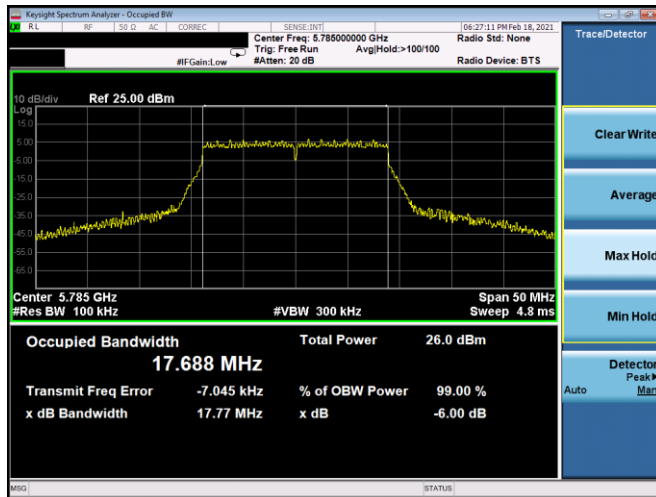
Plot 7-139. 6dB BW & 99% OBW Antenna 5B (20MHz BW 802.11n – Ch. 157, MCS5)
