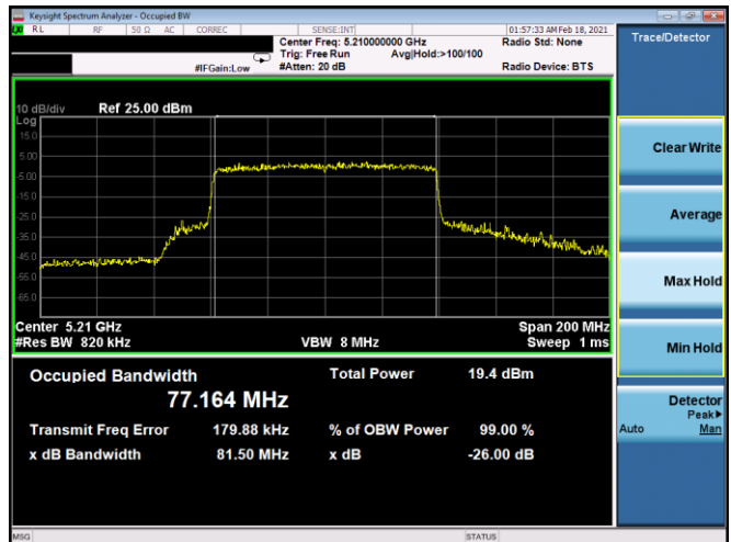
Plot 7-24. 26dB BW & 99% OBW Antenna 5T (80MHz BW 802.11ax(SU) – Ch. 42, MCS3)
