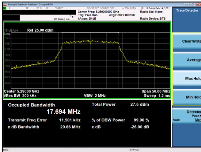
Plot 7-25. 26dB BW & 99% OBW Antenna 5T (20MHz BW 802.11n – Ch. 56, MCS3)
