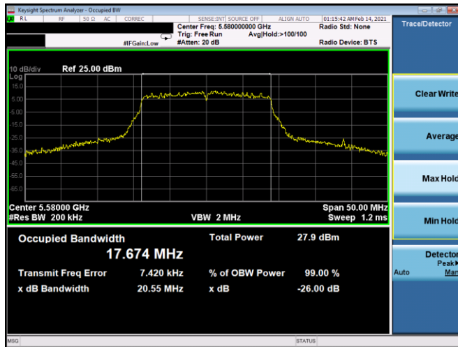
Plot 7-31. 26dB BW & 99% OBW Antenna 5T (20MHz BW 802.11n – Ch. 116, MCS3)
