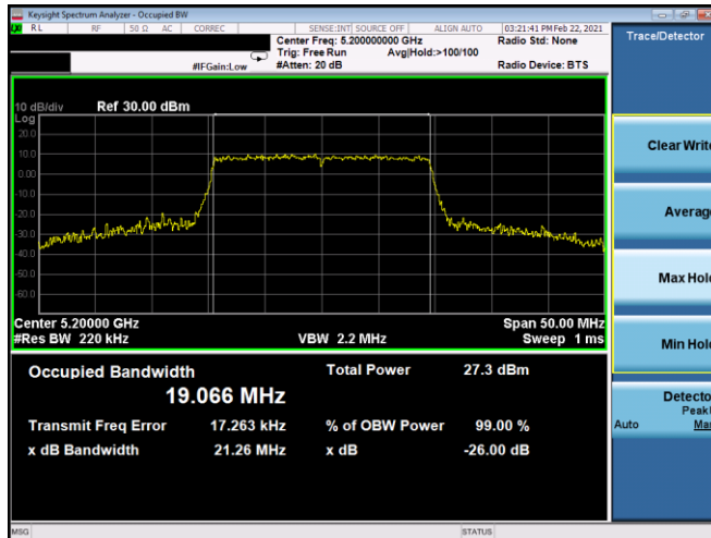
Plot 7-38. 26dB BW & 99% OBW Antenna 5T (20MHz BW 802.11ax(SU) – Ch. 40, MCS11)
