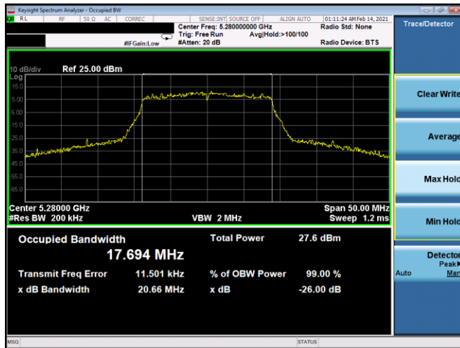
Plot 7-43. 26dB BW & 99% OBW Antenna 5T (20MHz BW 802.11n – Ch. 56, MCS5)
