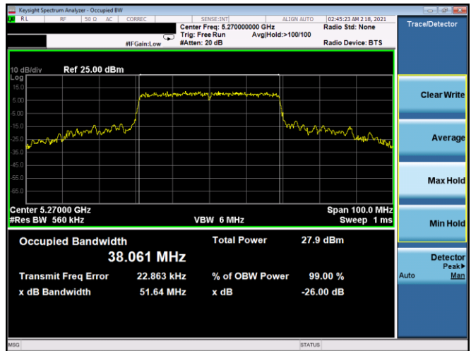
Plot 7-46. 26dB BW & 99% OBW Antenna 5T (40MHz BW 802.11ax(SU) – Ch. 54, MCS11)
