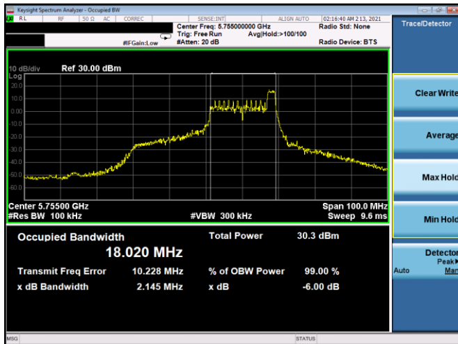
Plot 7-91. 6dB BW & 99% OBW Antenna 5B (40MHz BW 11ax Index 17 – RU26 – Ch.151)
