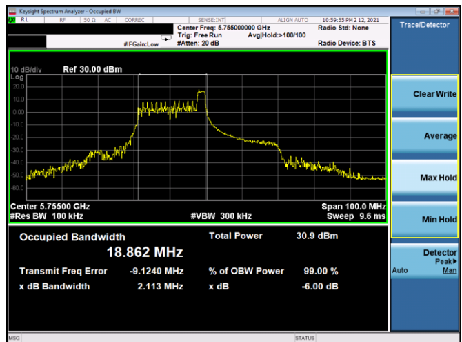
Plot 7-78. 6dB BW & 99% OBW Antenna 5T (40MHz BW 11ax Index 8 – RU26 – Ch.151)
