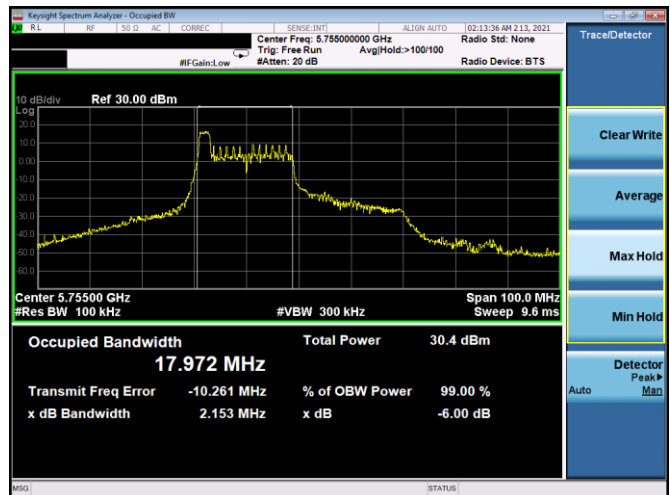
Plot 7-89. 6dB BW & 99% OBW Antenna 5B (40MHz BW 11ax Index 0 – RU26 – Ch.151)
