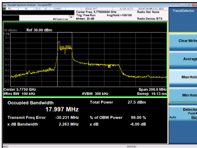
Plot 7-93. 6dB BW & 99% OBW Antenna 5B (80MHz BW 11ax Index 0 – RU26 – Ch.155)
