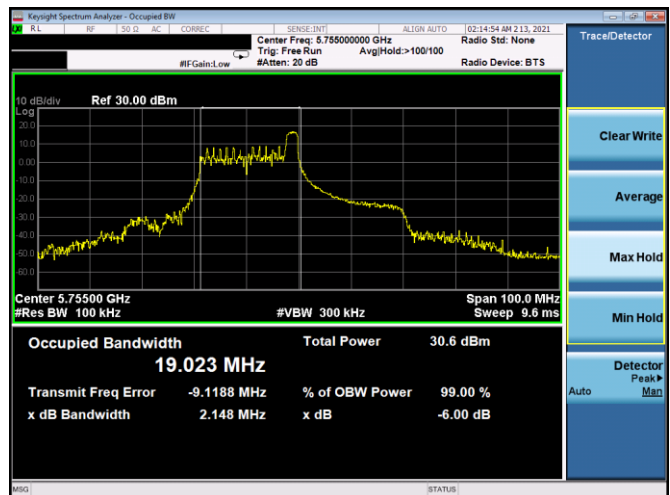
Plot 7-90. 6dB BW & 99% OBW Antenna 5B (40MHz BW 11ax Index 8 – RU26 – Ch.151)
