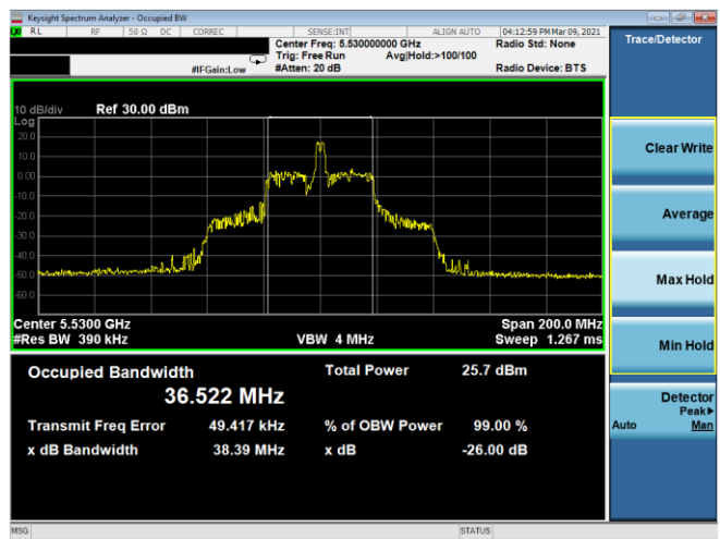
Plot 7-70. 26dB BW & 99% OBW Antenna 5B (80MHz BW 11ax Index 18 - RU26 - Ch.106)
