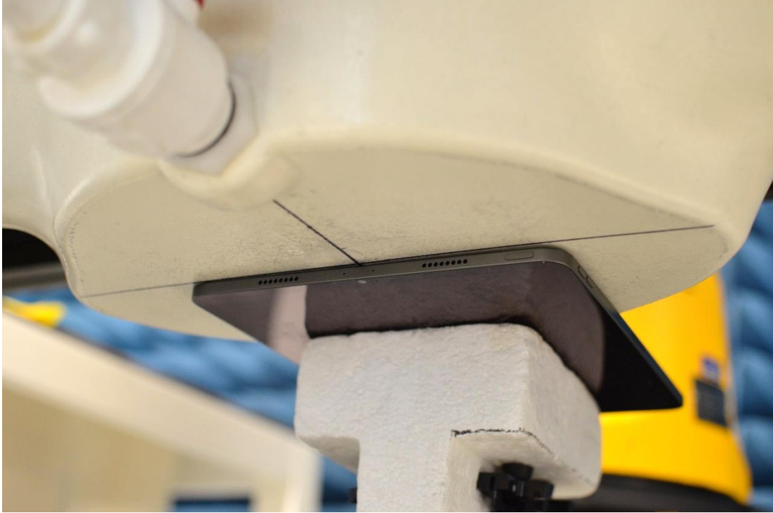
SAR Test Setup Photo 1: Back Side at 0mm – Ant WF8/7
