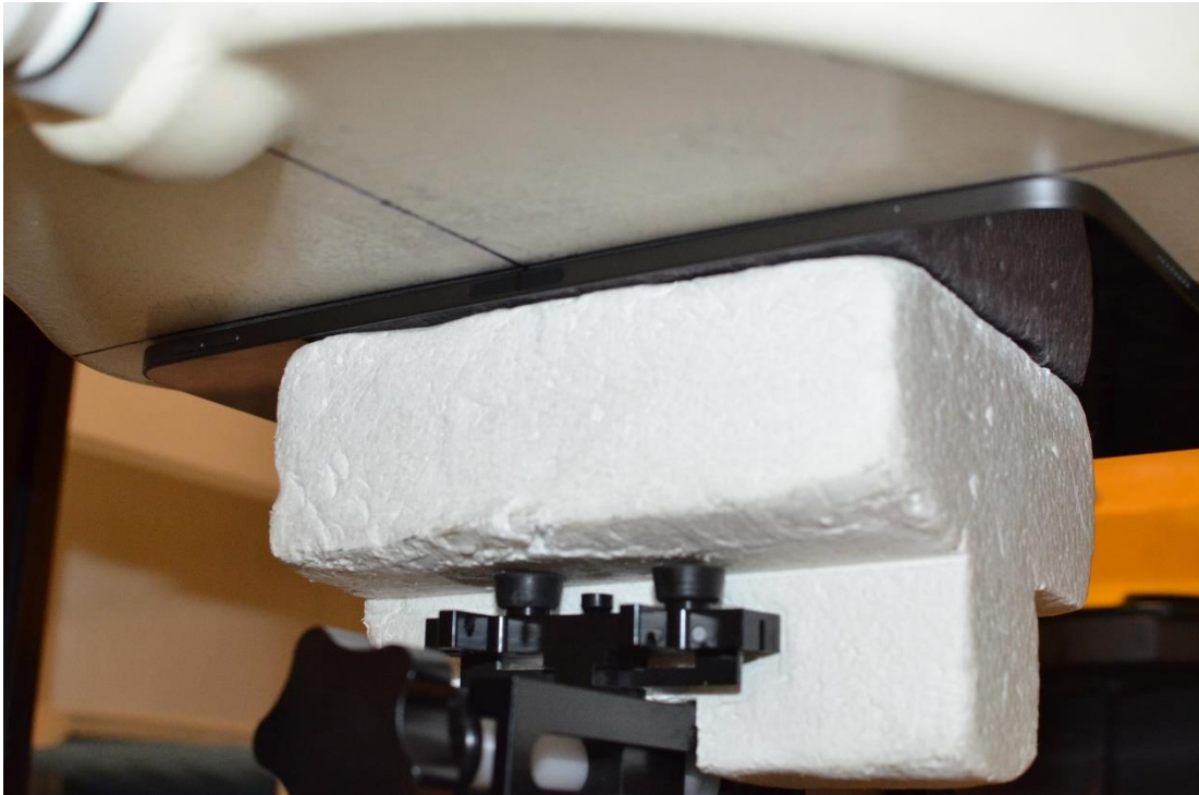
SAR Test Setup Photo 2: Back Side at 0mm – Ant 5T/5B
