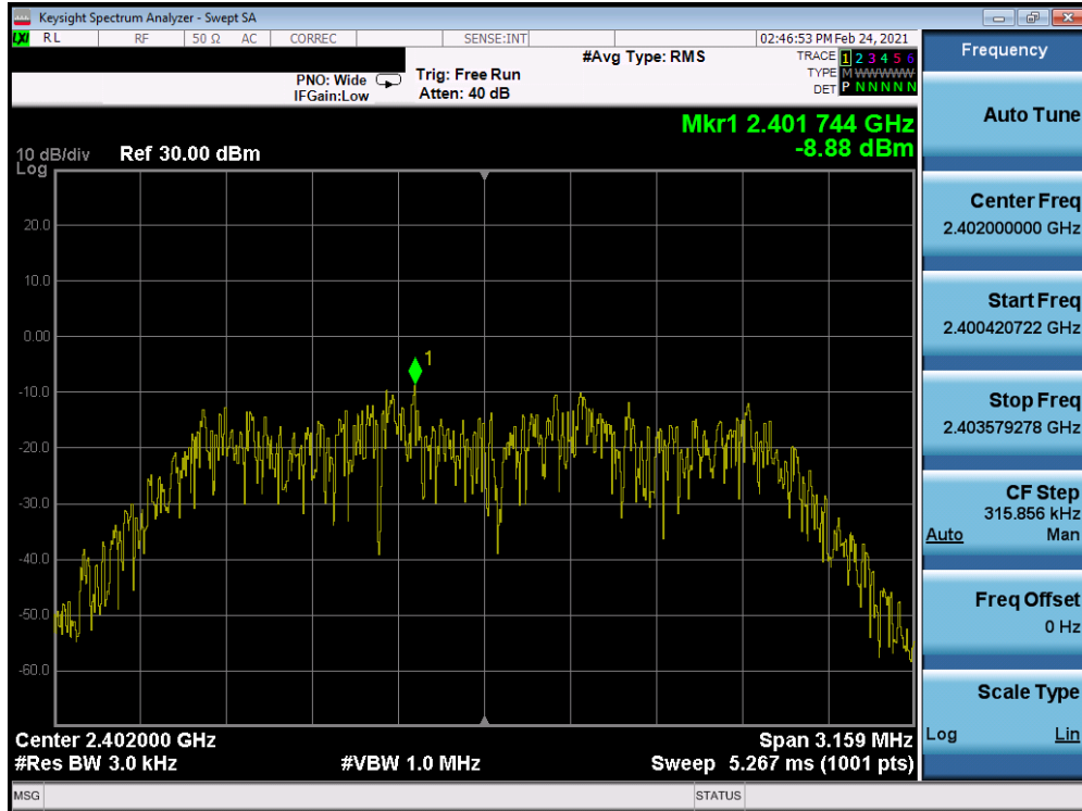
Plot 7-43. Power Spectral Density Plot TxBF Antenna WF8 (Bluetooth (HDR4), 4Mbps, iPA – Ch. 1)
