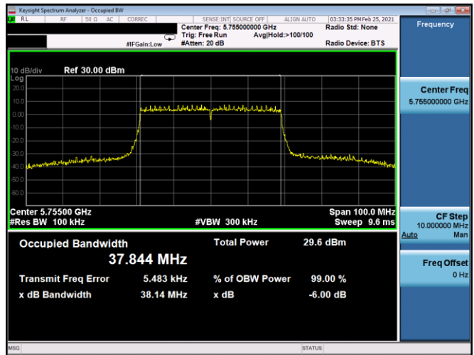
Plot 7-112. 6dB BW & 99% OBW Antenna 5T (40MHz BW 802.11ax(SU) – Ch. 151, MCS0)
