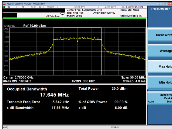
Plot 7-133. 6dB BW & 99% OBW Antenna 5B (20MHz BW 802.11n – Ch. 157, MCS3)
