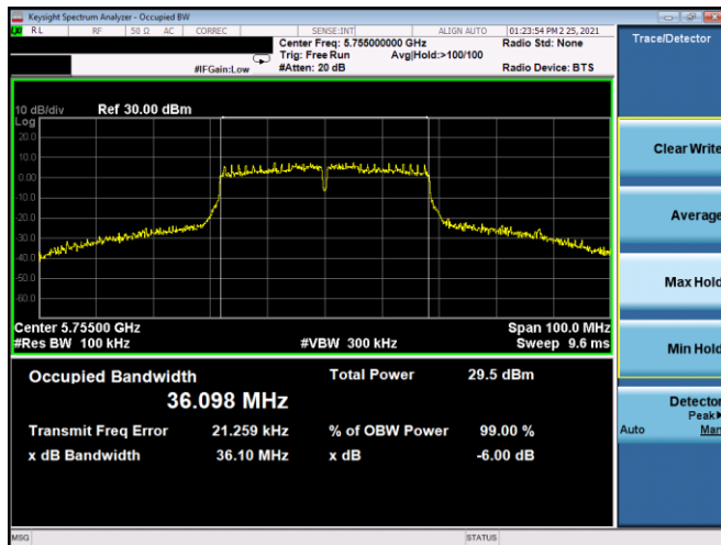
Plot 7-135. 6dB BW & 99% OBW Antenna 5B (40MHz BW 802.11n – Ch. 151, MCS3)
