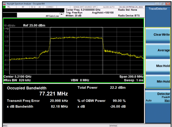
Plot 7-78. 26dB BW & 99% OBW Antenna 5B (80MHz BW 802.11ax(SU) – Ch. 42, MCS3)
