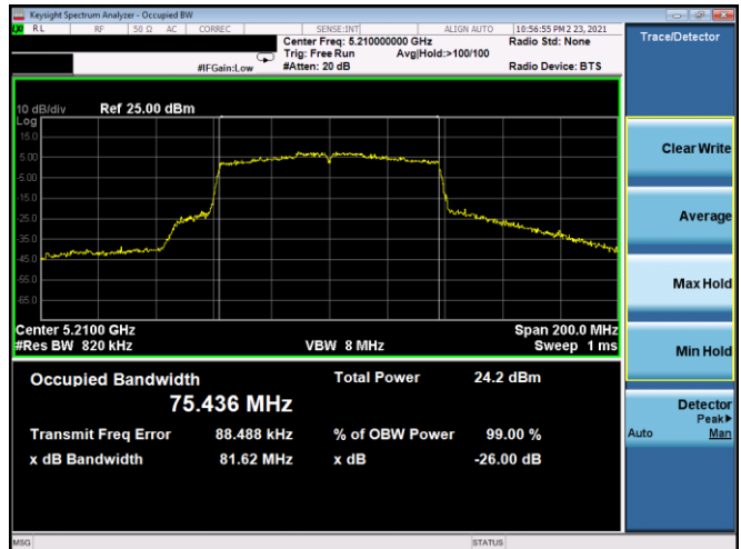
Plot 7-23. 26dB BW & 99% OBW Antenna 5T (80MHz BW 802.11ac – Ch. 42, MCS3)
