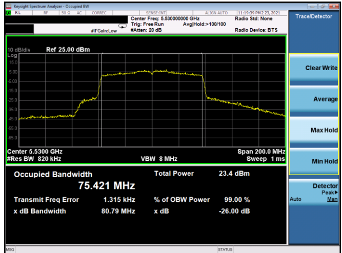
Plot 7-35. 26dB BW & 99% OBW Antenna 5T (80MHz BW 802.11ac – Ch. 106, MCS3)
