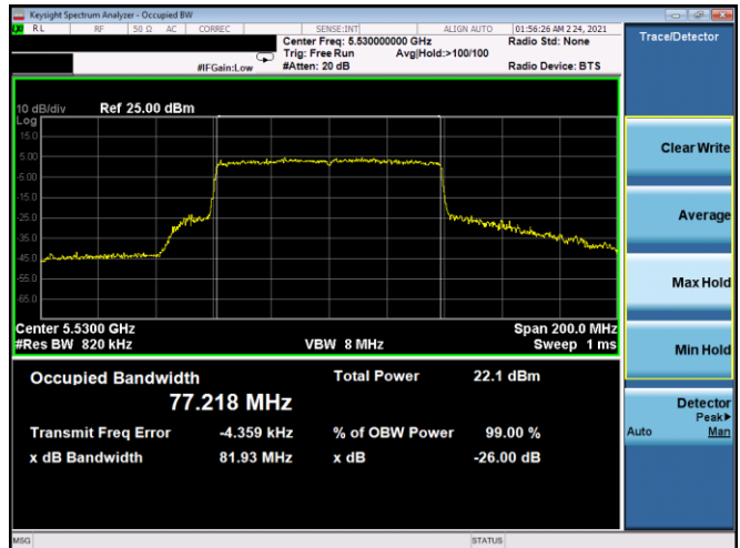
Plot 7-36. 26dB BW & 99% OBW Antenna 5T (80MHz BW 802.11ax(SU) – Ch. 106, MCS3)
