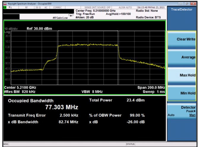
Plot 7-6. 26dB BW & 99% OBW Antenna 5T (80MHz BW 802.11ax(SU) – Ch. 42, MCS0)
