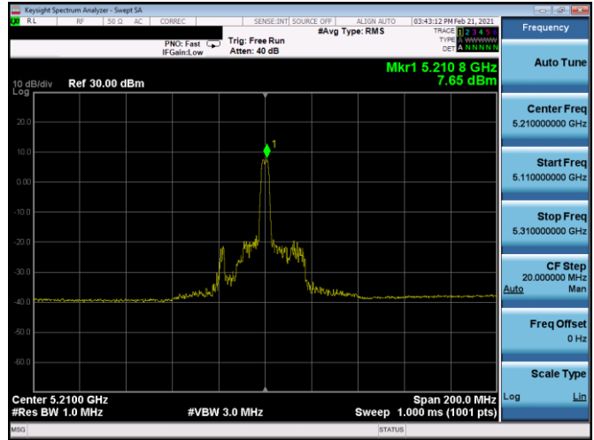
Plot 7-106. PSD Antenna 5T (80MHz BW 11ax Index 18 – RU26 – Ch.42)
