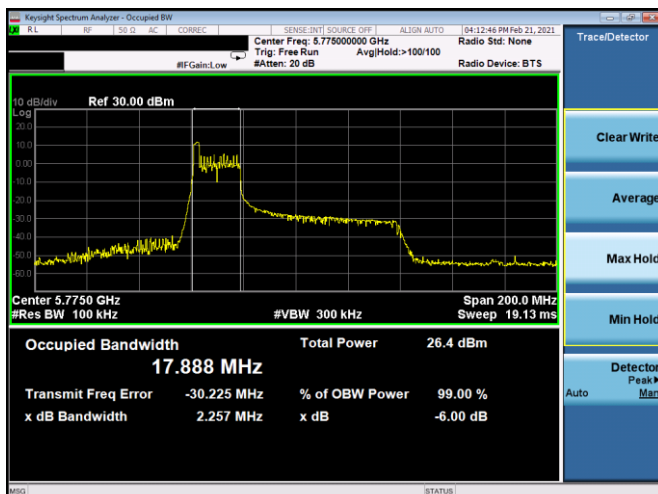
Plot 7-81. 6dB BW & 99% OBW Antenna 5T (80MHz BW 11ax Index 0 – RU26 – Ch.155)
