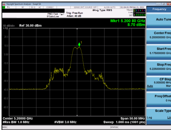
Plot 7-98. PSD Antenna 5T (20MHz BW 11ax Index 4 – RU26 – Ch.40)
