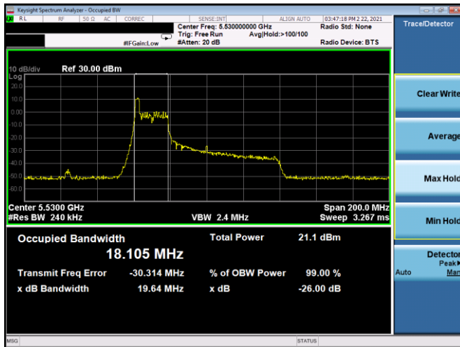
Plot 7-69. 26dB BW & 99% OBW Antenna 5B (80MHz BW 11ax Index 0 – RU26 – Ch.106)
