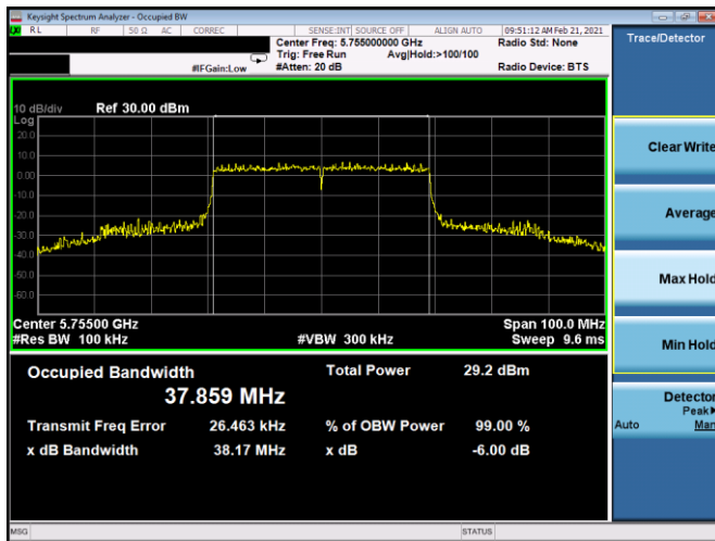
Plot 7-92. 6dB BW & 99% OBW Antenna 5B (40MHz BW 11ax – RU484 – Ch.151)
