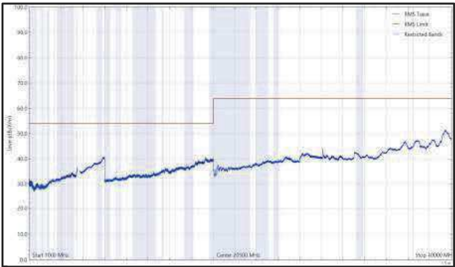
Figure 938 - U-NII-2C - 5500 MHz (CH100), HT20, CDD, Core 0 + Core 1, 1 GHz to 40 GHz, Horizontal (RMS)
