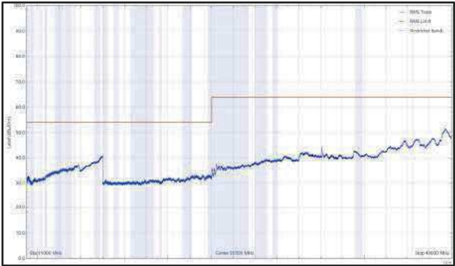
Figure 967 - 5825 MHz (CH165), HE20, RU26-0, Core 0 + Core 1, 1 GHz to 40 GHz, Horizontal (RMS)
