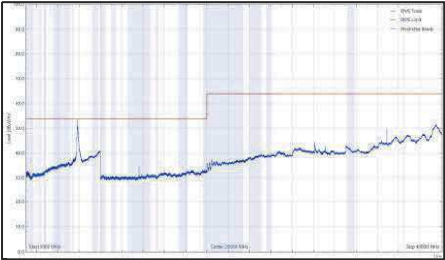
Figure 970 - 5825 MHz (CH165), HE20, RU26-0, Core 0 + Core 1, 1 GHz to 40 GHz, Vertical (RMS)
