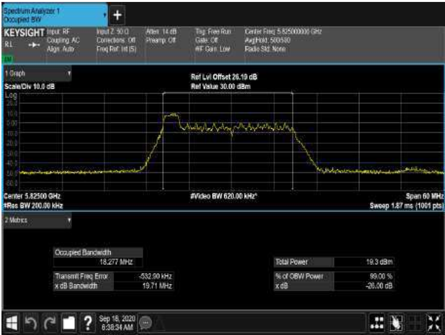
Figure 531 - 5825 MHz - 99% Occupied Bandwidth
