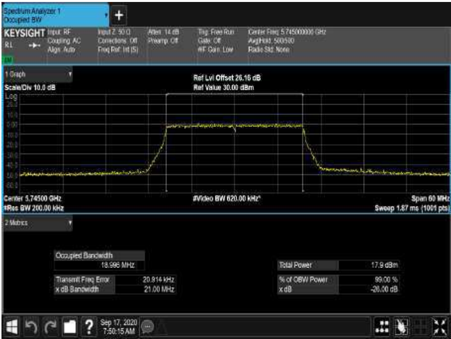
Figure 516 - 5745 MHz - 99% Occupied Bandwidth
