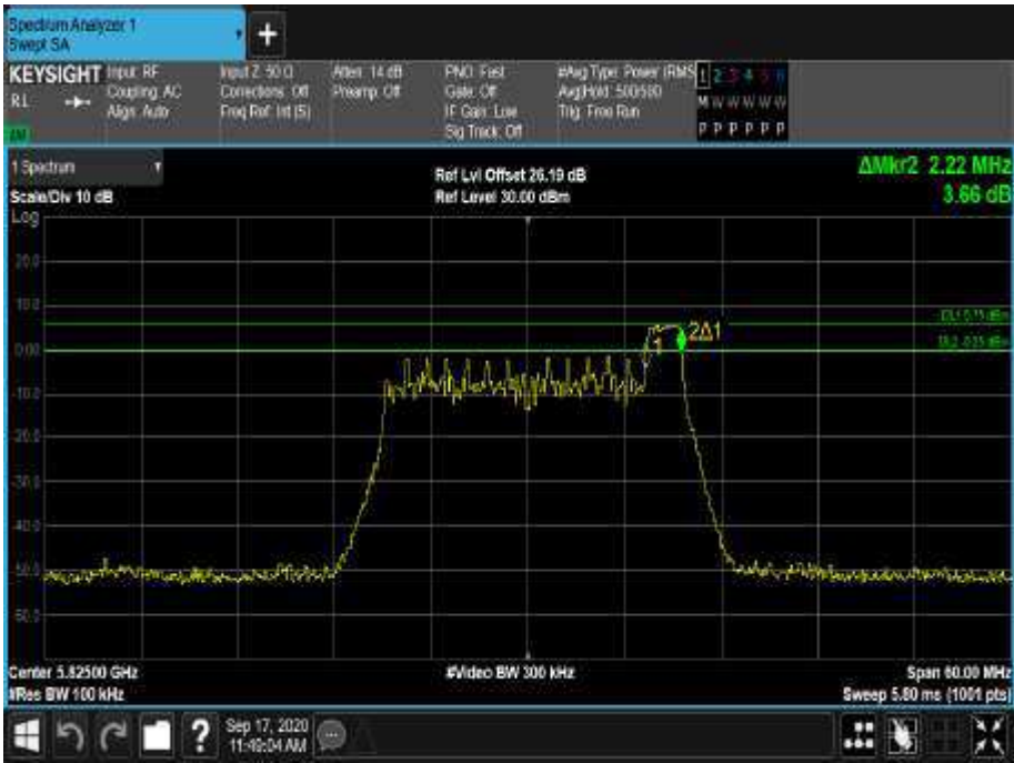
Figure 508 - 5825 MHz - 6 dB DTS Bandwidth
