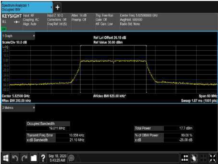
Figure 522 - 5825 MHz - 99% Occupied Bandwidth
