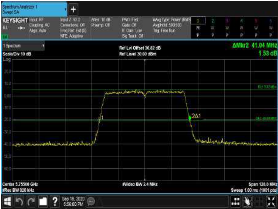
Figure 602 - 5755 MHz - 26 dB Emission Bandwidth
