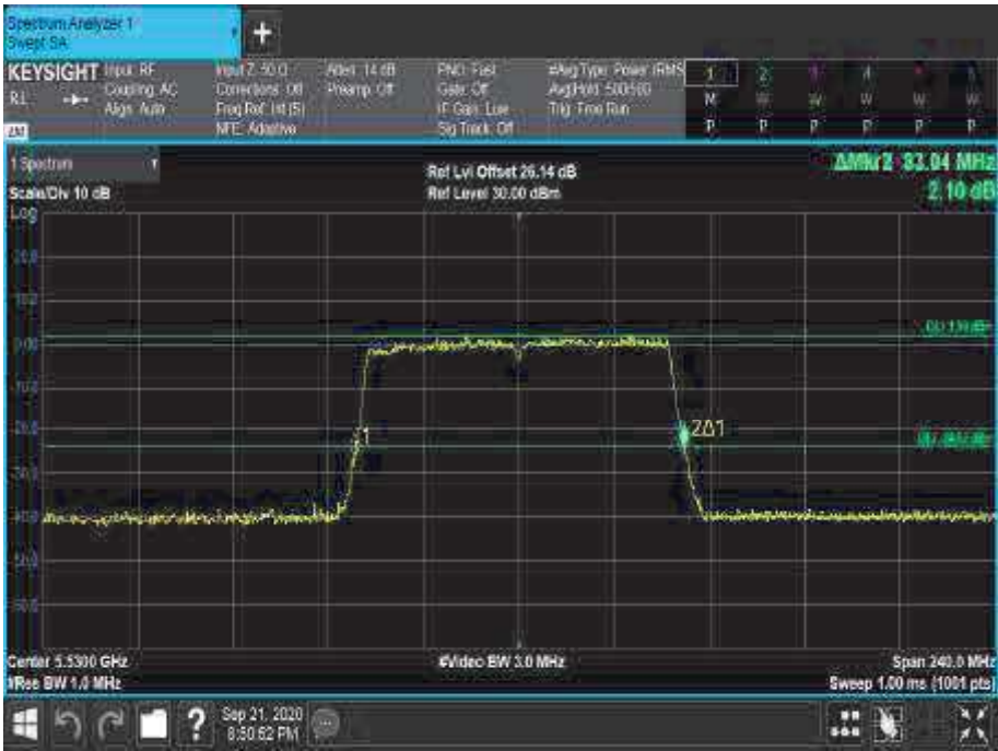
Figure 397 - 5530 MHz - 26 dB Emission Bandwidth
