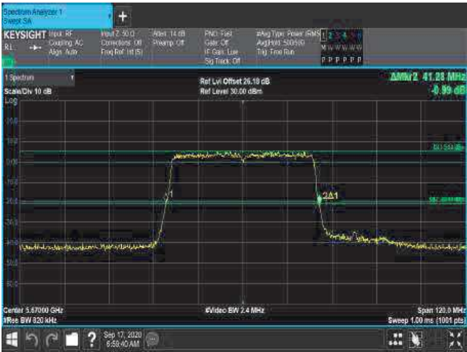
Figure 387 - 5670 MHz - 26 dB Emission Bandwidth
