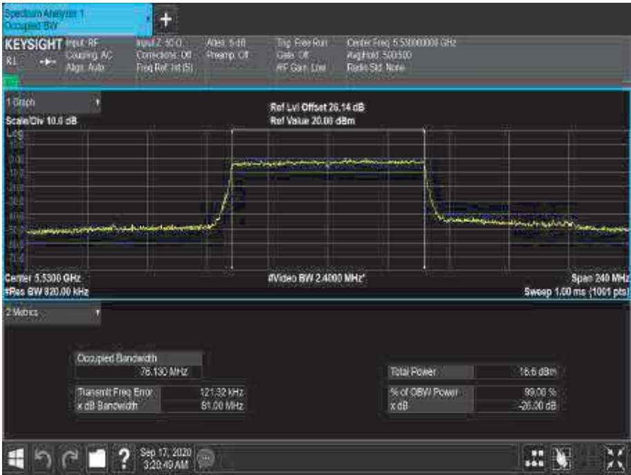
Figure 398 - 5530 MHz - 99% Occupied Bandwidth
