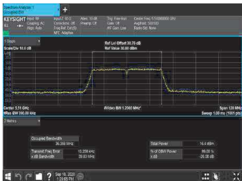
Figure 360 - 5510 MHz - 99% Occupied Bandwidth
