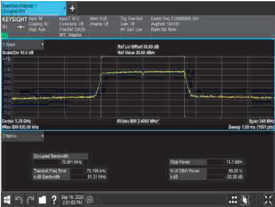
Figure 264 - 5290 MHz - 99% Occupied Bandwidth
