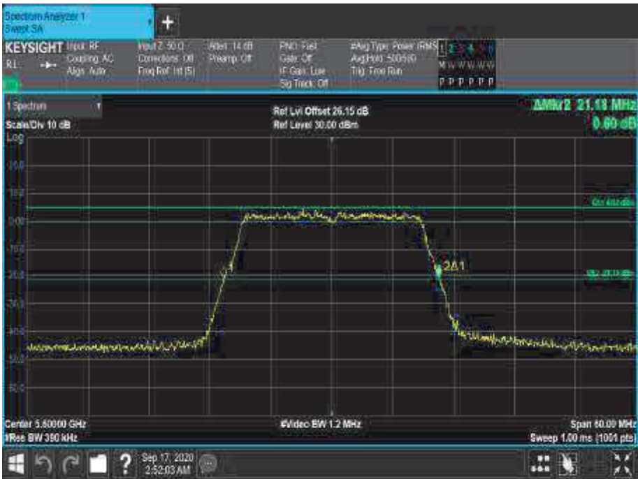
Figure 281 - 5600 MHz - 26 dB Emission Bandwidth
