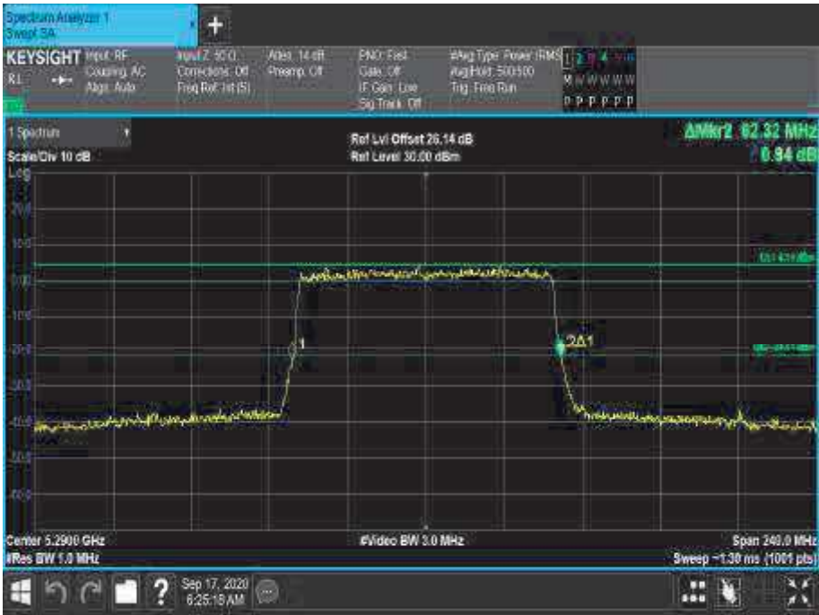
Figure 265 - 5290 MHz - 26 dB Emission Bandwidth
