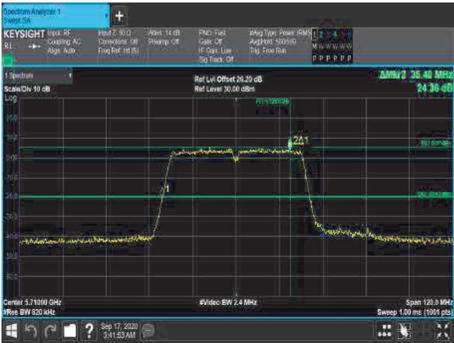
Figure 341 - 5710 MHz - 26 dB Emission Bandwidth
