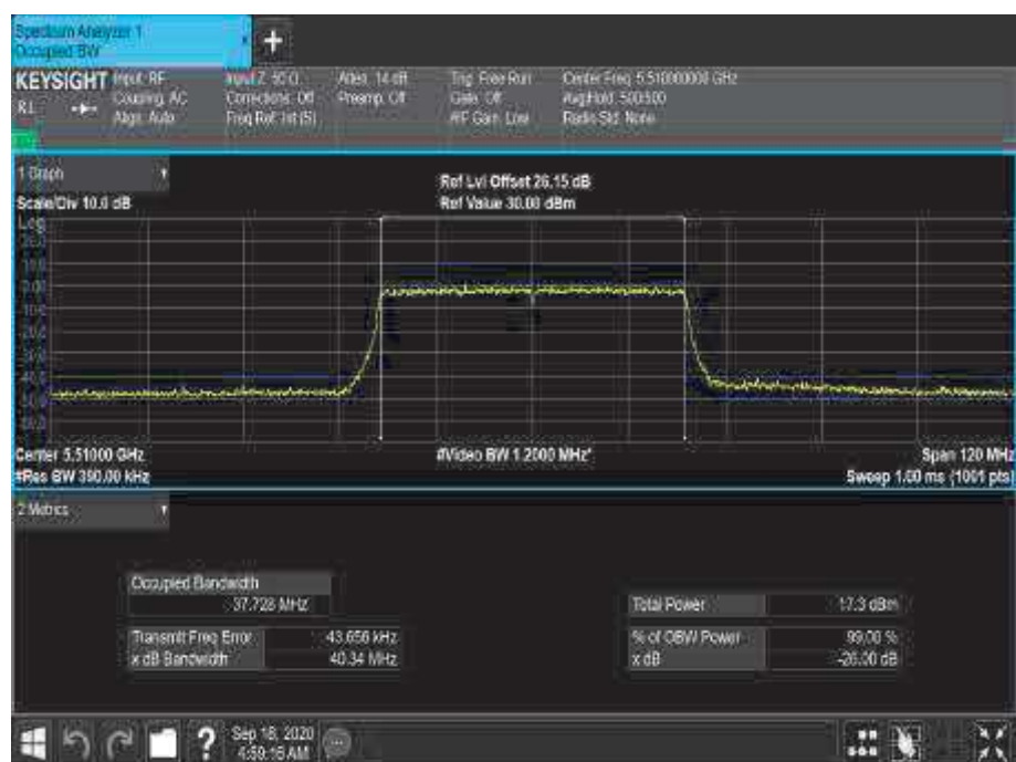
Figure 376 - 5510 MHz - 99% Occupied Bandwidth
