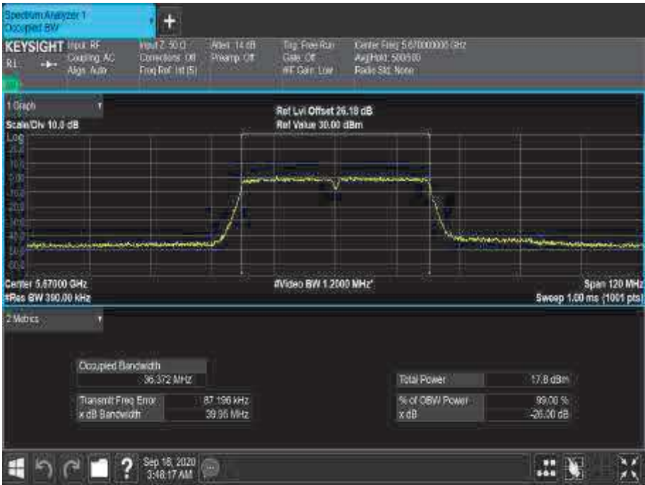
Figure 348 - 5670 MHz - 99% Occupied Bandwidth
