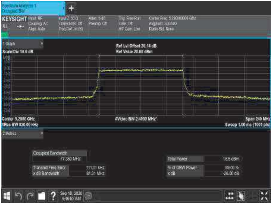
Figure 268 - 5290 MHz - 99% Occupied Bandwidth
