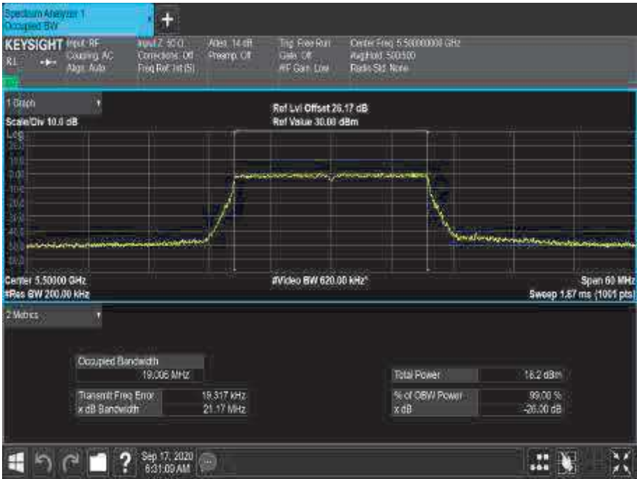
Figure 312 - 5500 MHz - 99% Occupied Bandwidth
