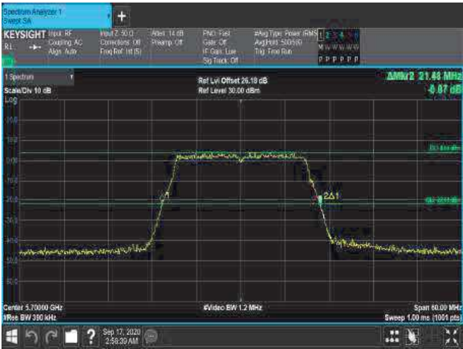
Figure 283 - 5700 MHz - 26 dB Emission Bandwidth
