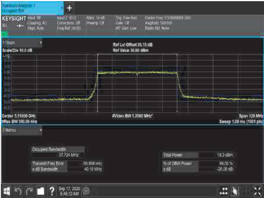
Figure 368 - 5510 MHz - 99% Occupied Bandwidth
