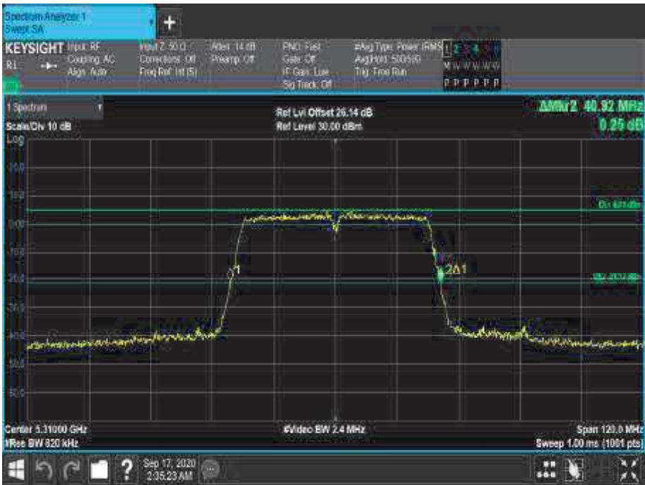
Figure 235 - 5310 MHz - 26 dB Emission Bandwidth
