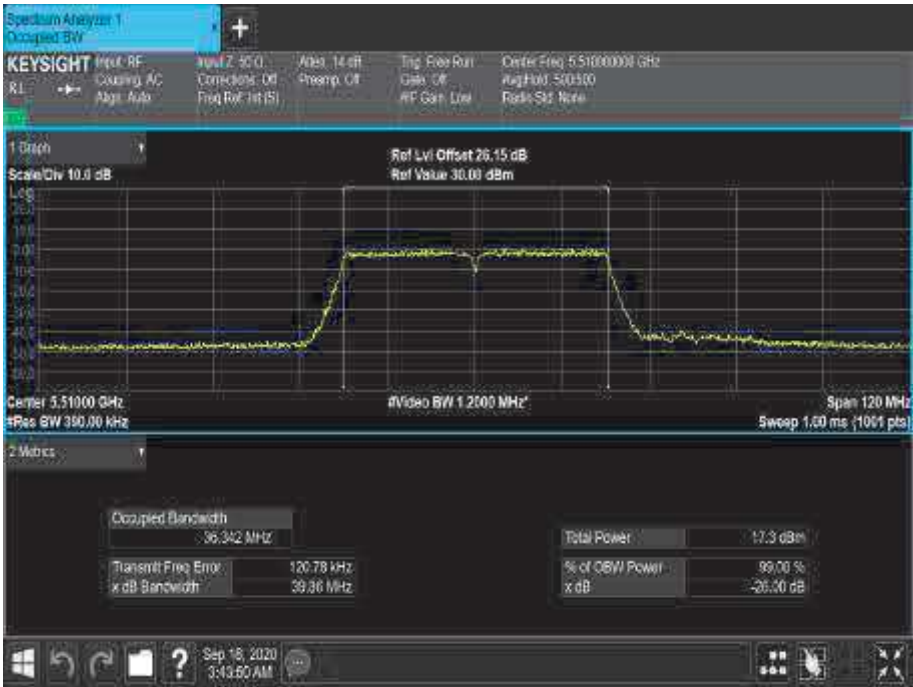
Figure 352 - 5510 MHz - 99% Occupied Bandwidth
