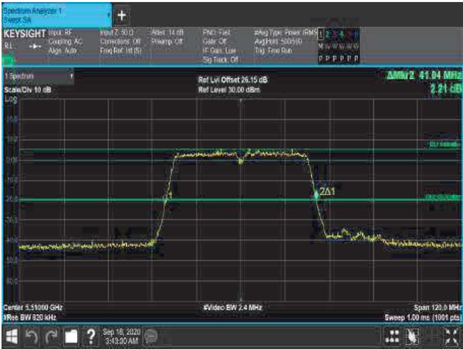
Figure 351 - 5510 MHz - 26 dB Emission Bandwidth
