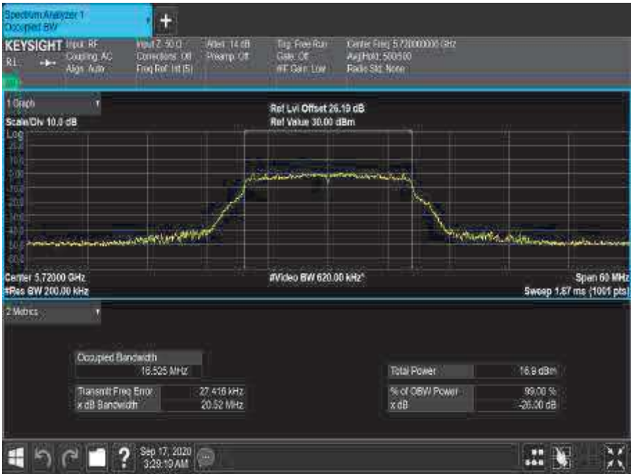
Figure 278 - 5720 MHz - 99% Occupied Bandwidth
