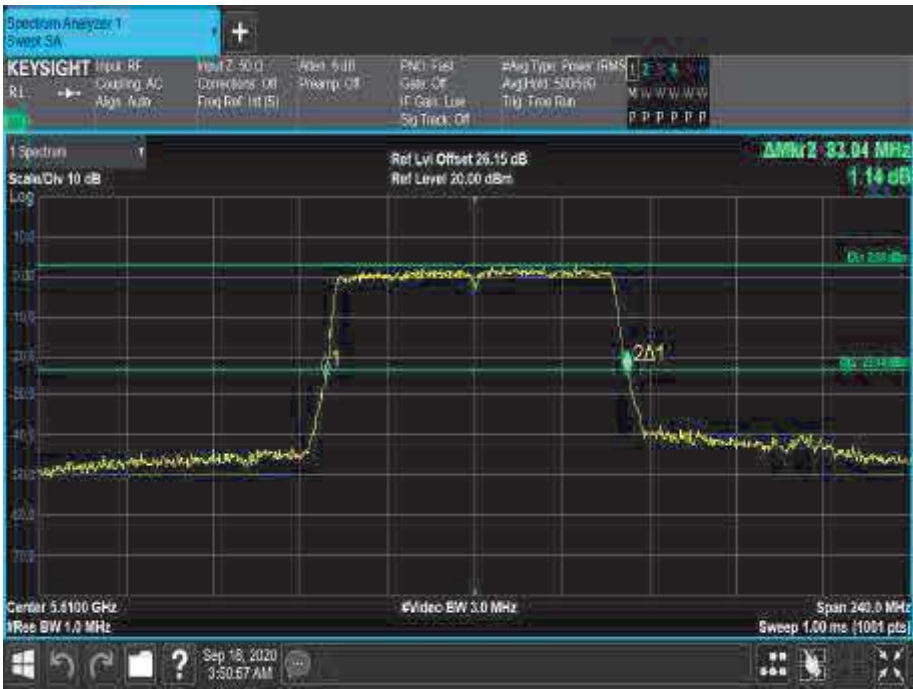
Figure 399 - 5610 MHz - 26 dB Emission Bandwidth
