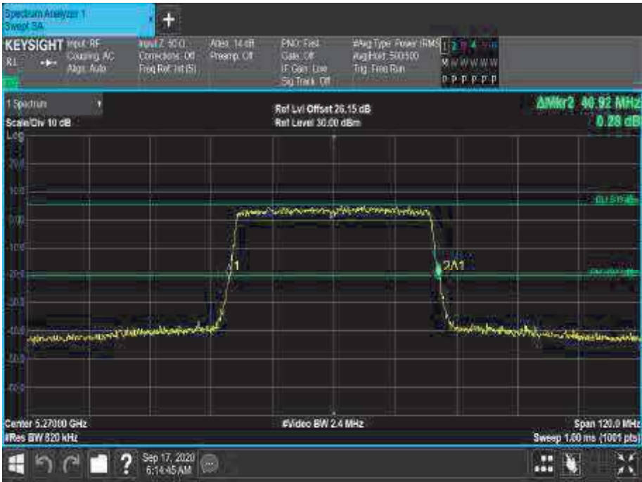
Figure 245 - 5270 MHz - 26 dB Emission Bandwidth
