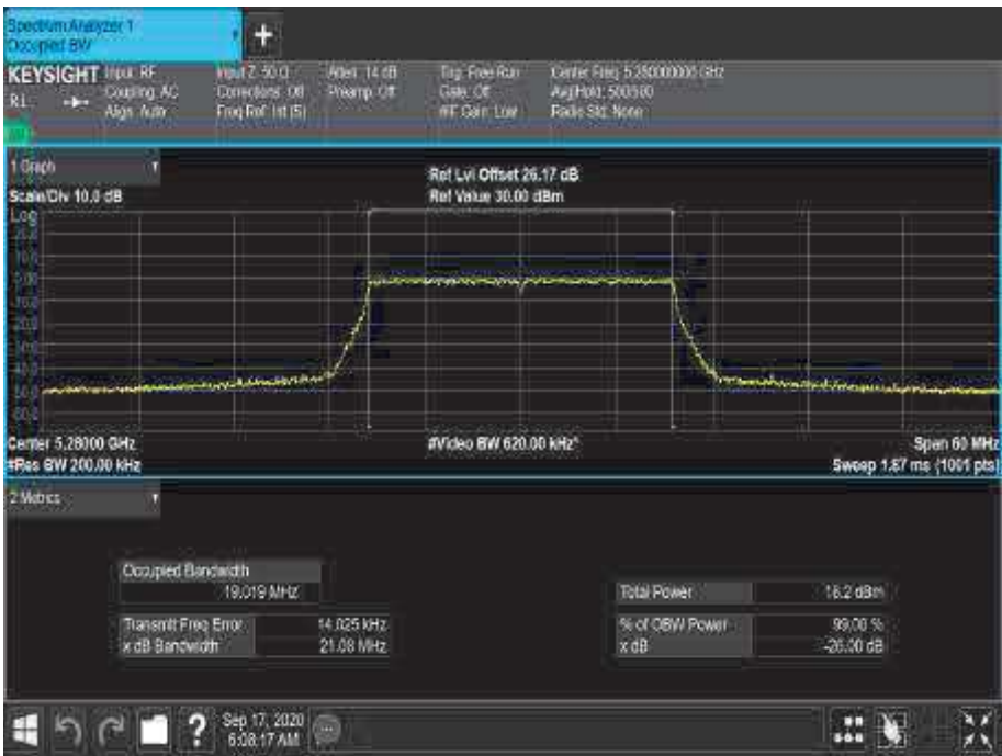
Figure 226 - 5280 MHz - 99% Occupied Bandwidth
