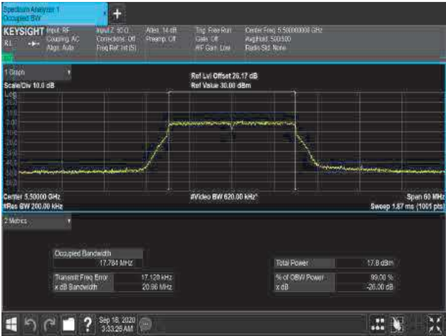
Figure 288 - 5500 MHz - 99% Occupied Bandwidth
