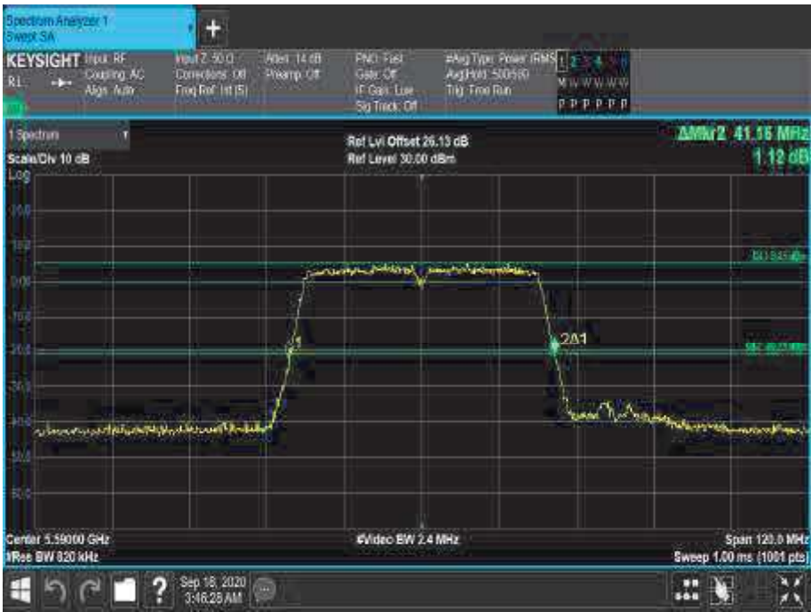
Figure 353 - 5590 MHz - 26 dB Emission Bandwidth
