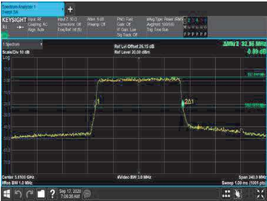
Figure 417 - 5610 MHz - 26 dB Emission Bandwidth
