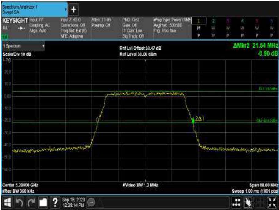
Figure 51 - 5200 MHz - 26 dB Emission Bandwidth
