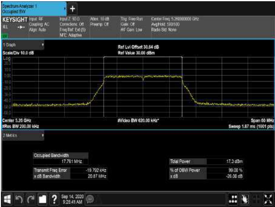
Figure 194 - 5260 MHz - 99% Occupied Bandwidth
