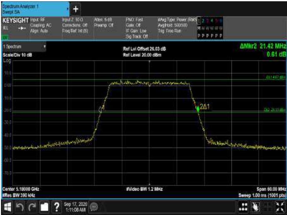
Figure 13 - 5180 MHz - 26 dB Emission Bandwidth
