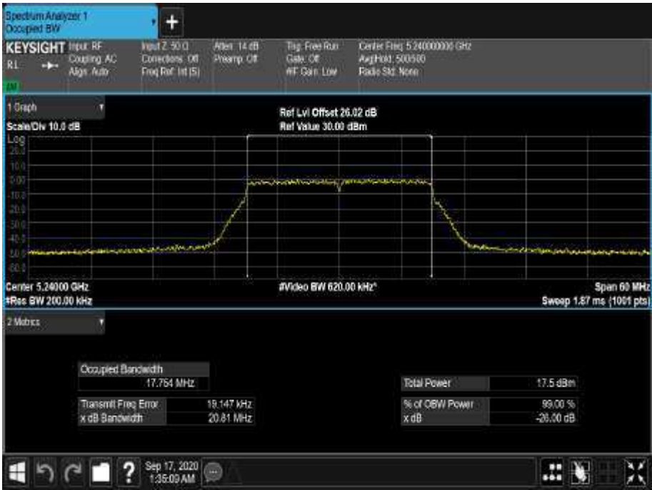
Figure 18 - 5240 MHz - 99% Occupied Bandwidth
