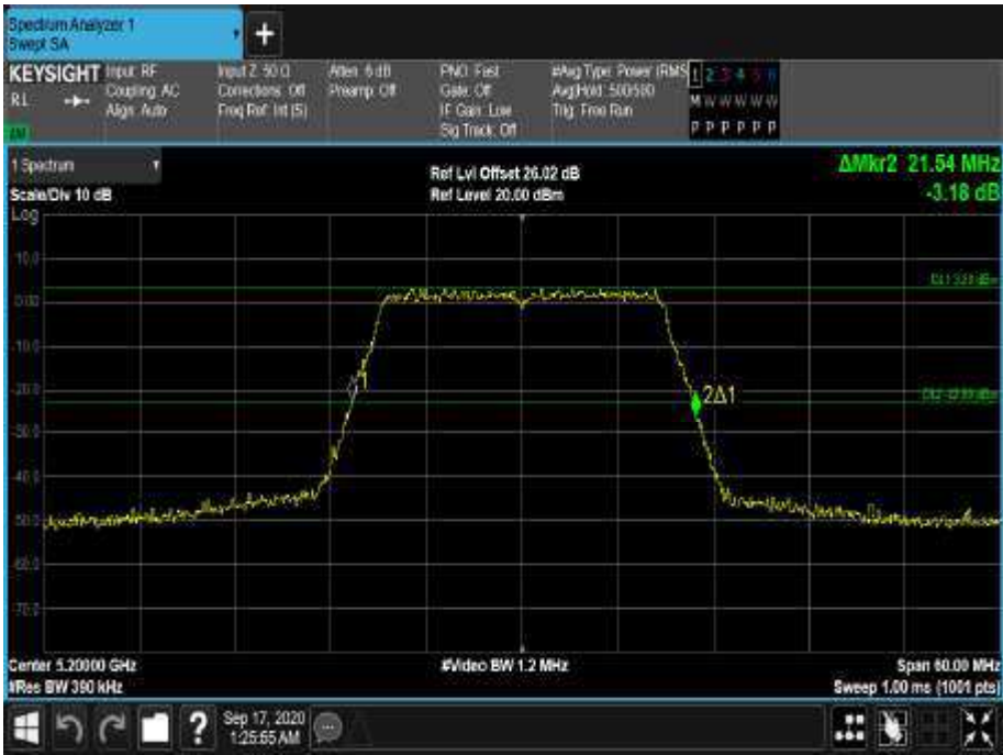
Figure 39 - 5200 MHz - 26 dB Emission Bandwidth
