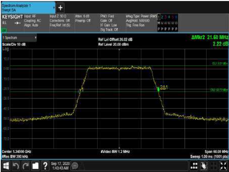
Figure 47 - 5240 MHz - 26 dB Emission Bandwidth
