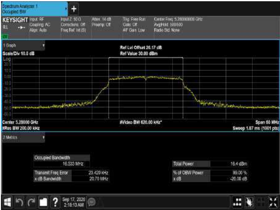
Figure 184 - 5280 MHz - 99% Occupied Bandwidth
