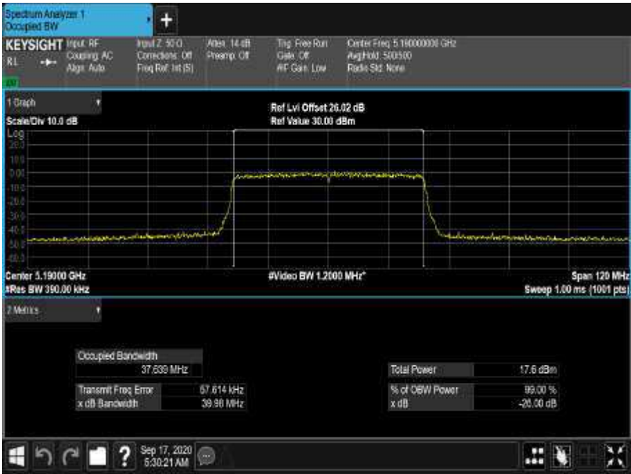
Figure 130 - 5190 MHz - 99% Occupied Bandwidth
