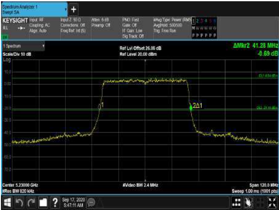
Figure 151 - 5230 MHz - 26 dB Emission Bandwidth
