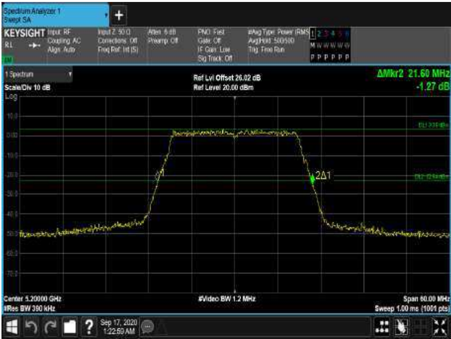
Figure 15 - 5200 MHz - 26 dB Emission Bandwidth
