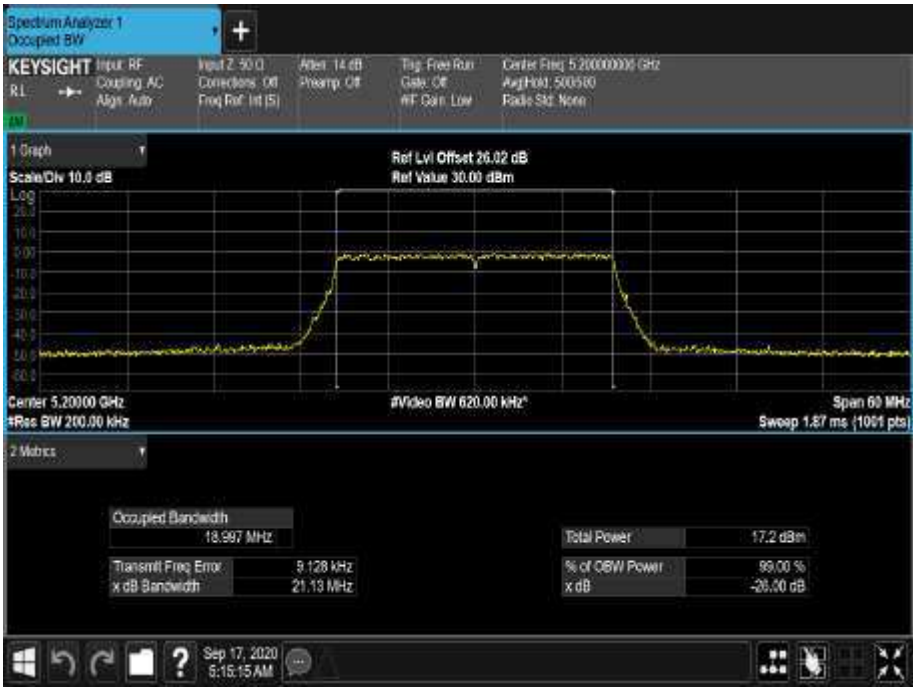
Figure 70 - 5200 MHz - 99% Occupied Bandwidth
