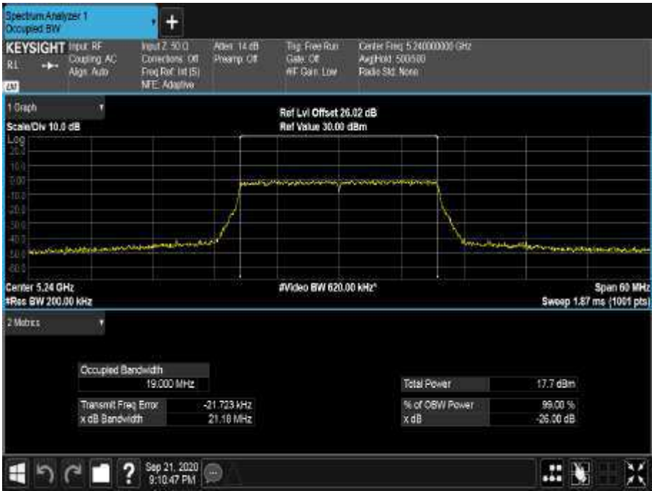
Figure 78 - 5240 MHz - 99% O ccupied Bandwidth h
