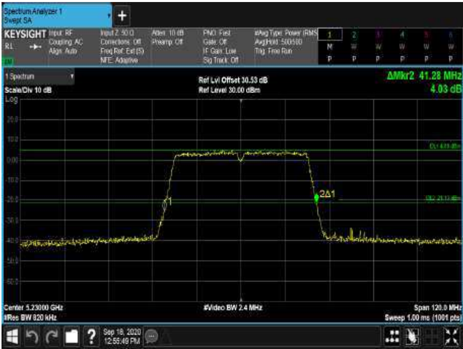
Figure 123 - 5230 MHz - 26 dB Emission Bandwidth
