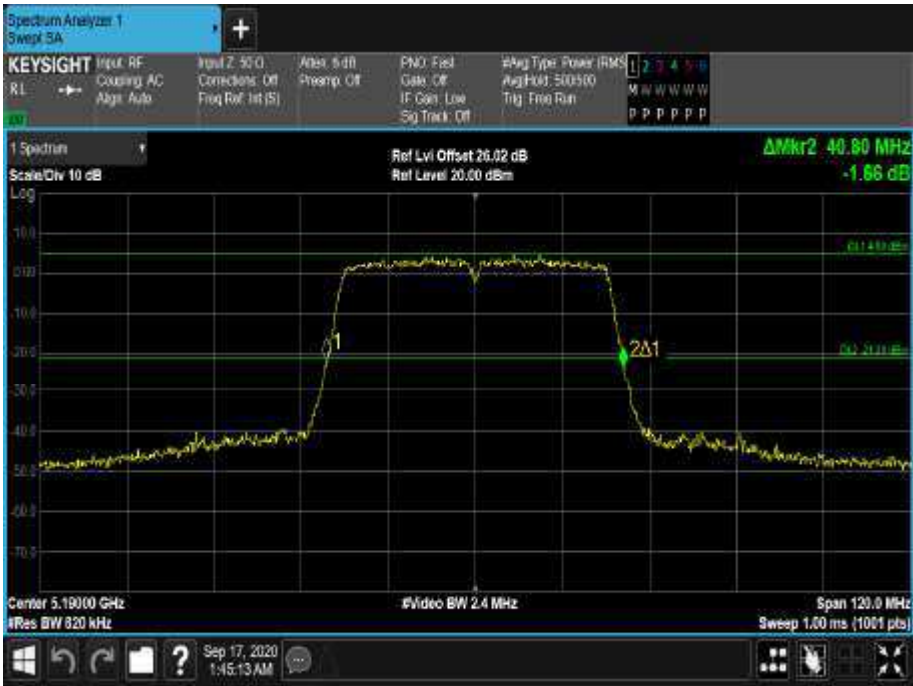
Figure 97 - 5190 MHz - 26 dB Emission Bandwidth
