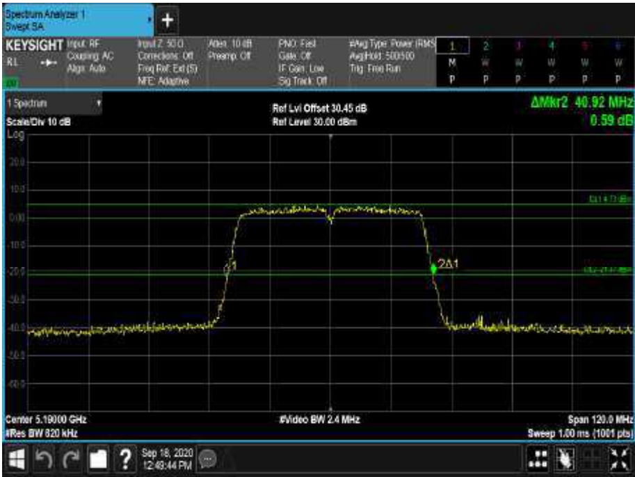
Figure 121 - 5190 MHz - 26 dB Emission Bandwidth
