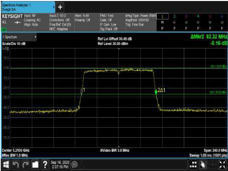
Figure 165 - 5210 MHz - 26 dB Emission Bandwidth
