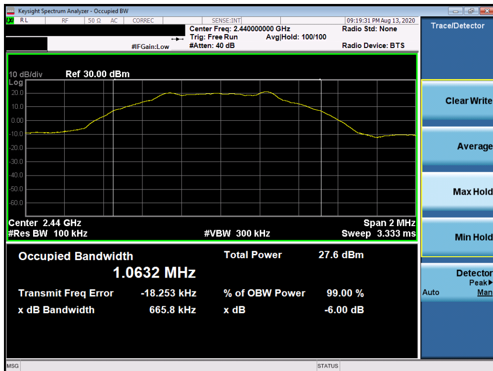
Plot 7-8. 6dB Bandwidth Plot Antenna 1a (Bluetooth (LE), 1Mbps, ePA – Ch. 19)
