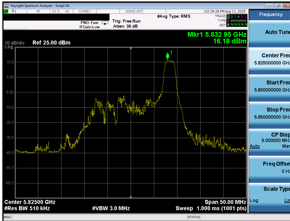
Plot 7-1143. Power Spectral Density Plot CDD Diversity Antenna 2b (20MHz BW 802.11ax Index 8 – RU26 (UNII Band 3) – Ch. 165)
