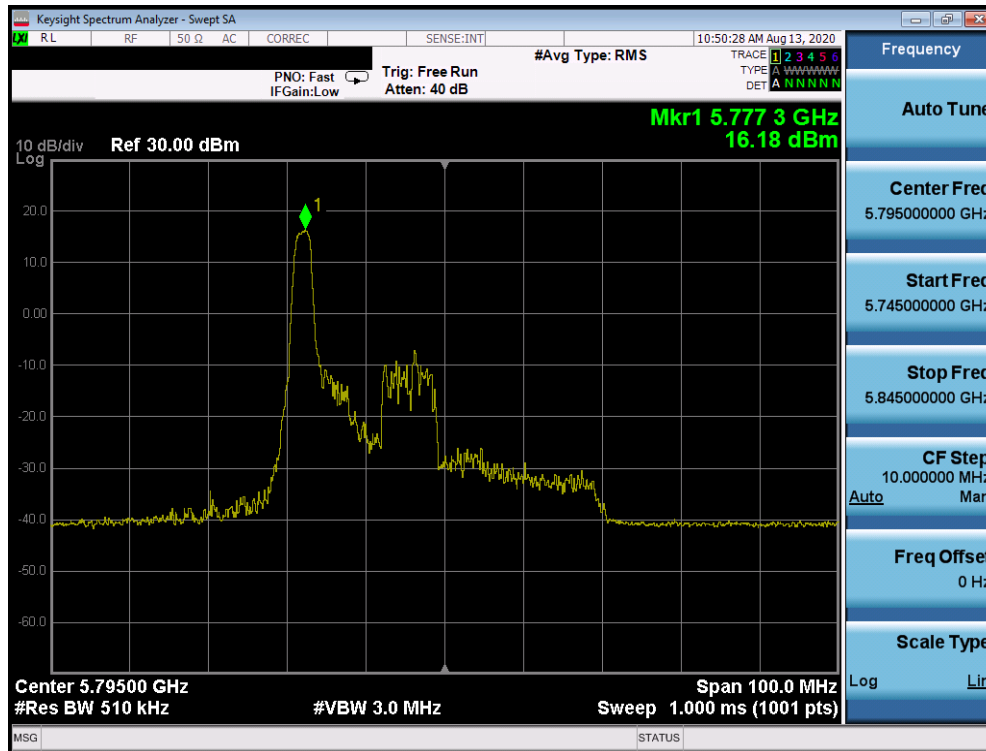
Plot 7-1157. Power Spectral Density Plot CDD Diversity Antenna 2b (40MHz BW 802.11ax Index 0 – RU26 (UNII Band 3) – Ch. 159)
