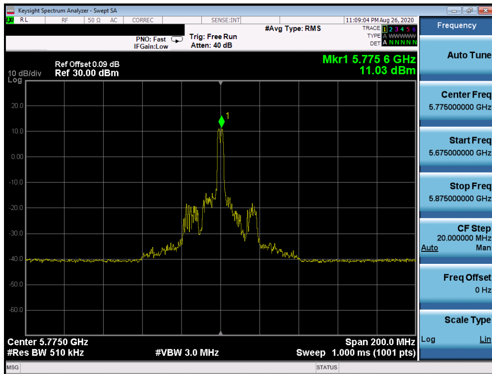
Plot 7-1170. Power Spectral Density Plot CDD Diversity Antenna 1b (80MHz BW 802.11ax Index 18 – RU26 (UNII Band 3) – Ch. 155)
