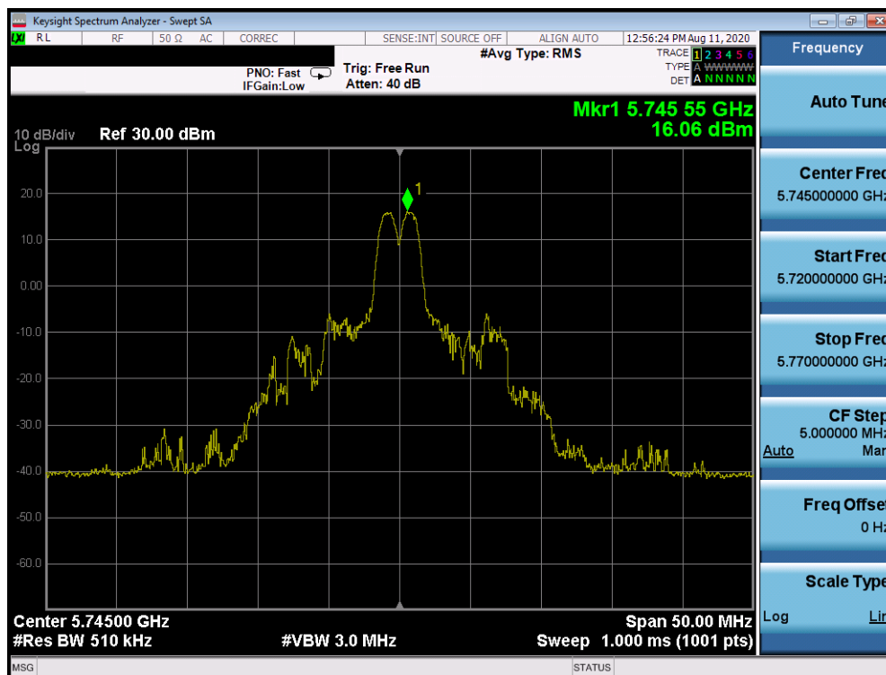
Plot 7-1130. Power Spectral Density Plot CDD Diversity Antenna 1b (20MHz BW 802.11ax Index 4 – RU26 (UNII Band 3) – Ch. 149)
