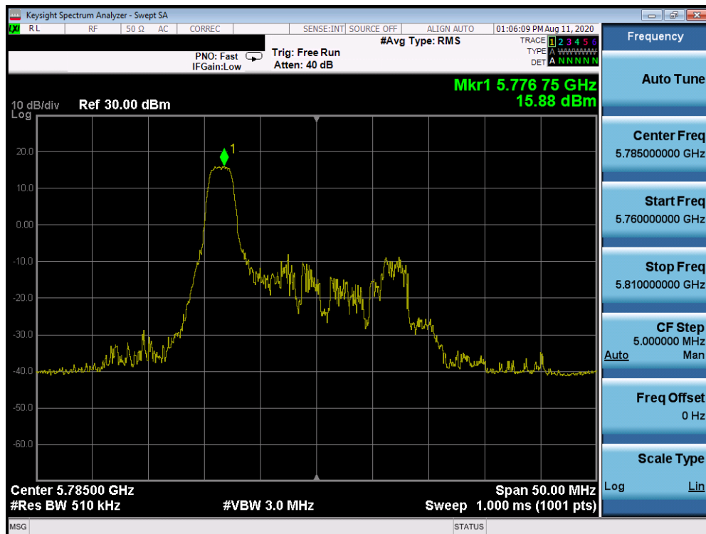
Plot 7-1134. Power Spectral Density Plot CDD Diversity Antenna 1b (20MHz BW 802.11ax Index 0 – RU26 (UNII Band 3) – Ch. 157)
