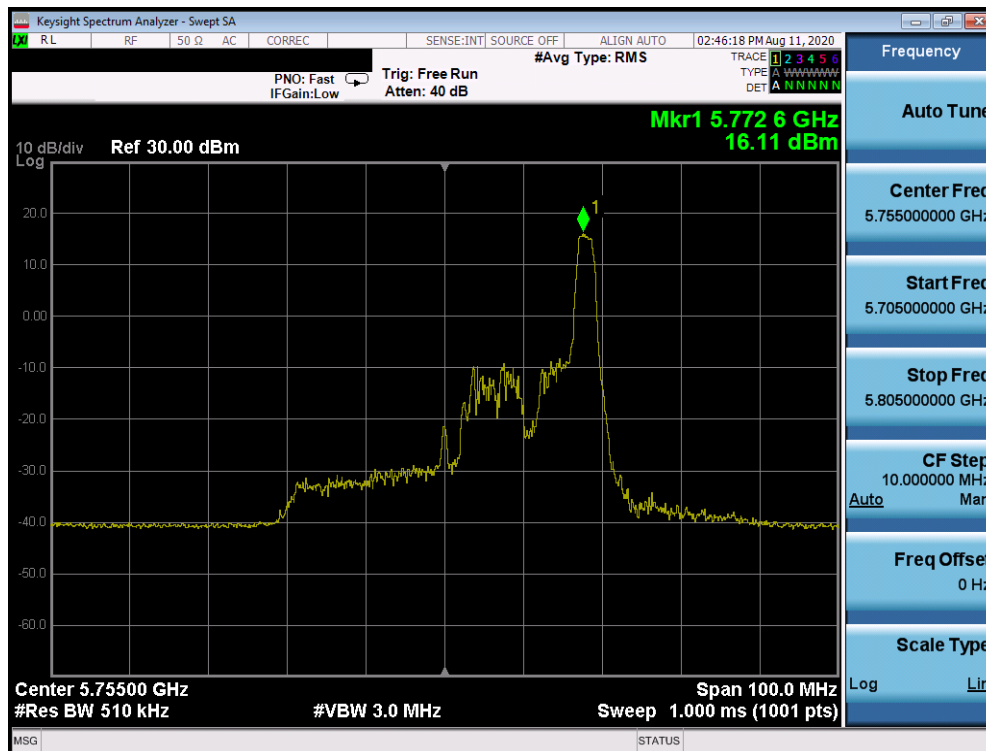
Plot 7-1156. Power Spectral Density Plot CDD Diversity Antenna 1b (40MHz BW 802.11ax Index 17 – RU26 (UNII Band 3) – Ch. 151)
