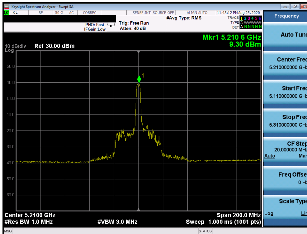
Plot 7-594. Power Spectral Density Plot Antenna 1b (80MHz BW 802.11ax Index 18 – RU26 (UNII Band 1) – Ch. 42)
