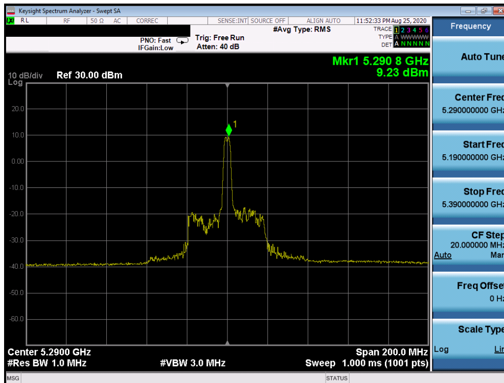
Plot 7-618. Power Spectral Density Plot Antenna 1b (80MHz BW 802.11ax Index 18 – RU26 (UNII Band 2A) – Ch. 58)
