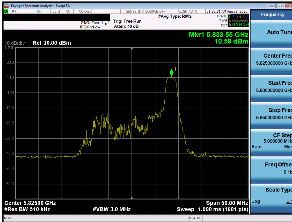
Plot 7-533. Power Spectral Density Plot Antenna 2a (20MHz BW 802.11ax Index 8 – RU26 (UNII Band 3) – Ch. 165)
