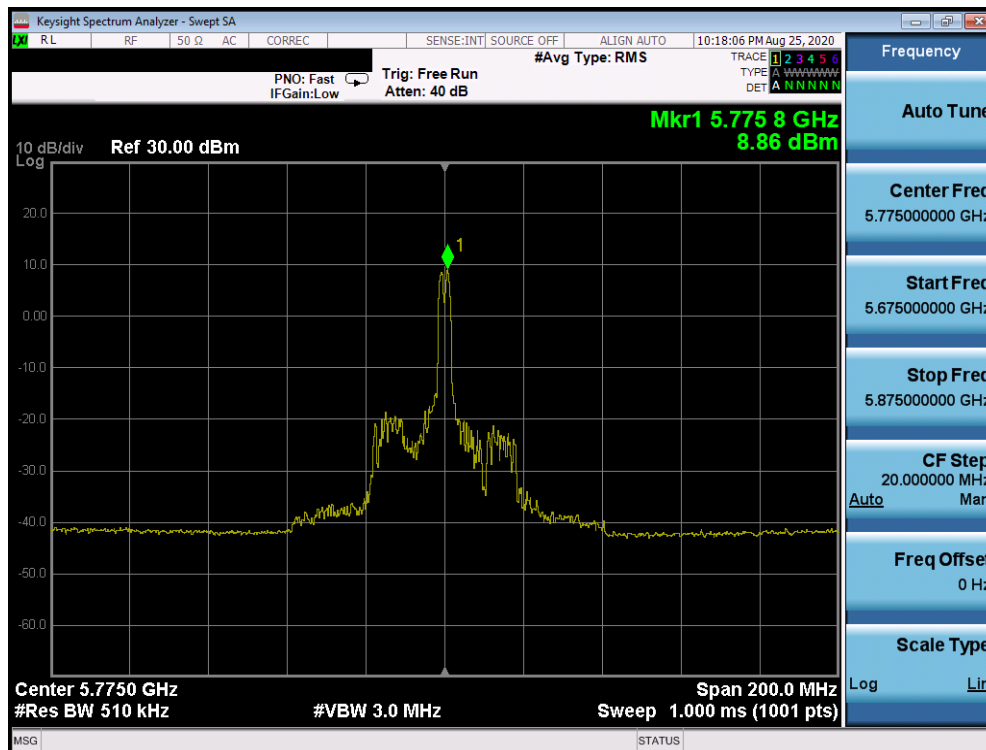
Plot 7-546. Power Spectral Density Plot Antenna 2a (80MHz BW 802.11ax Index 18 – RU26 (UNII Band 3) – Ch. 155)
