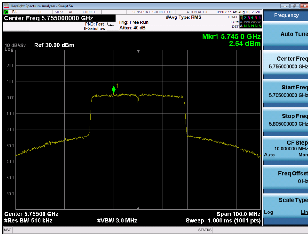
Plot 7-543. Power Spectral Density Plot Antenna 2a (40MHz BW 802.11ax – RU484 (UNII Band 3) – Ch. 151)
