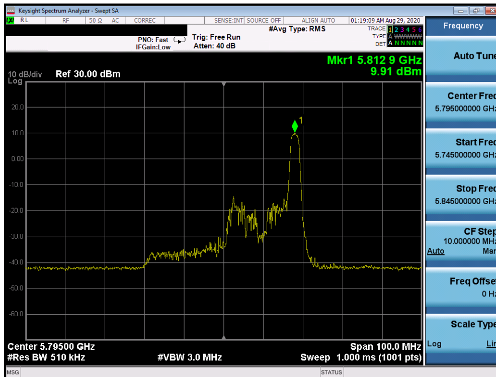
Plot 7-542. Power Spectral Density Plot Antenna 2a (40MHz BW 802.11ax Index 17 – RU26 (UNII Band 3) – Ch. 159)
