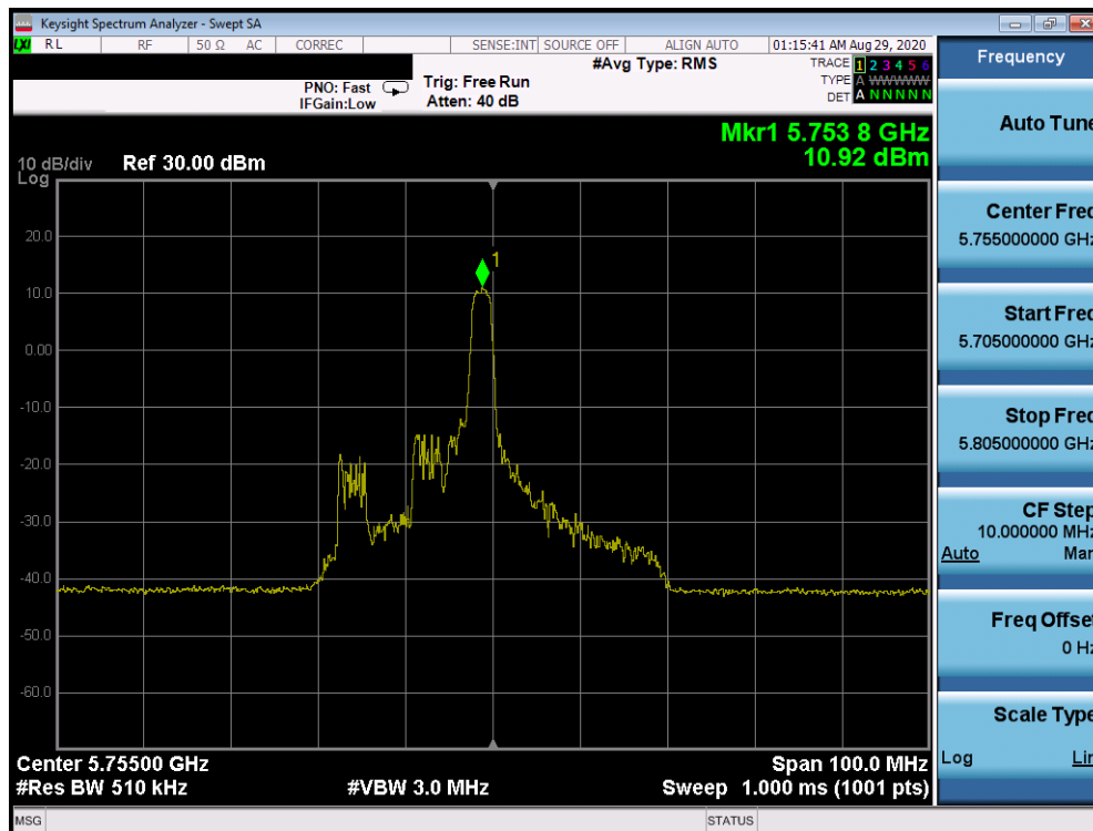
Plot 7-538. Power Spectral Density Plot Antenna 2a (40MHz BW 802.11ax Index 8 – RU26 (UNII Band 3) – Ch. 151)
