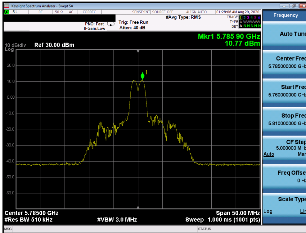
Plot 7-529. Power Spectral Density Plot Antenna 2a (20MHz BW 802.11ax Index 4 – RU26 (UNII Band 3) – Ch. 157)
