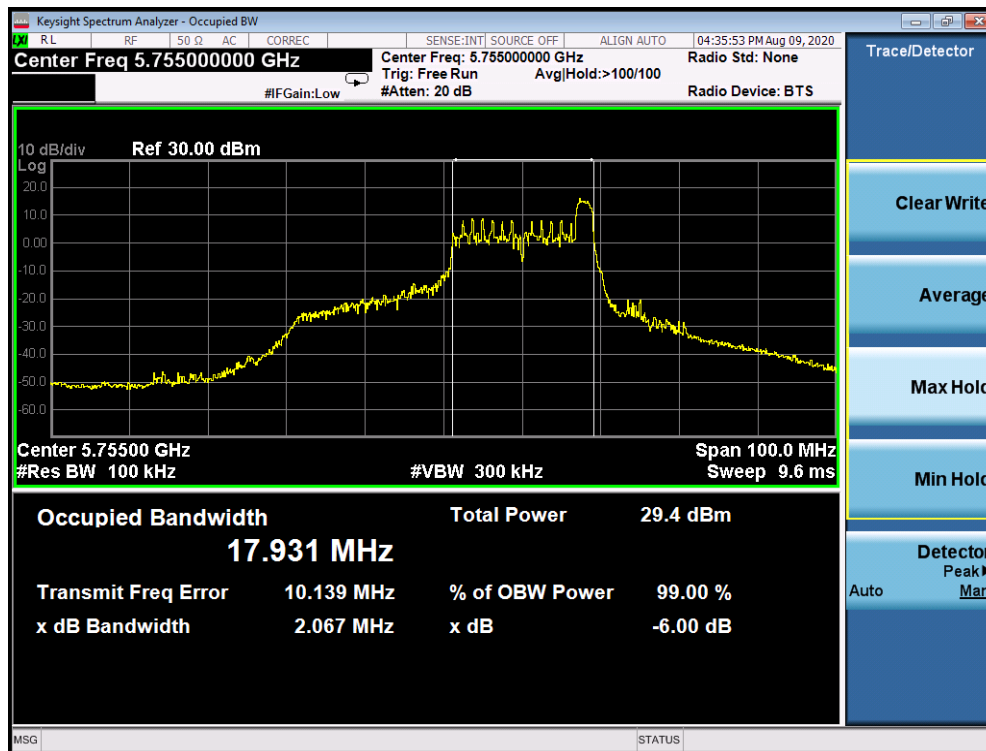
Plot 7-303. 6dB Bandwidth Plot Antenna 1b (40MHz BW 802.11ax Index 17 – RU26 (UNII Band 3) – Ch. 151)
