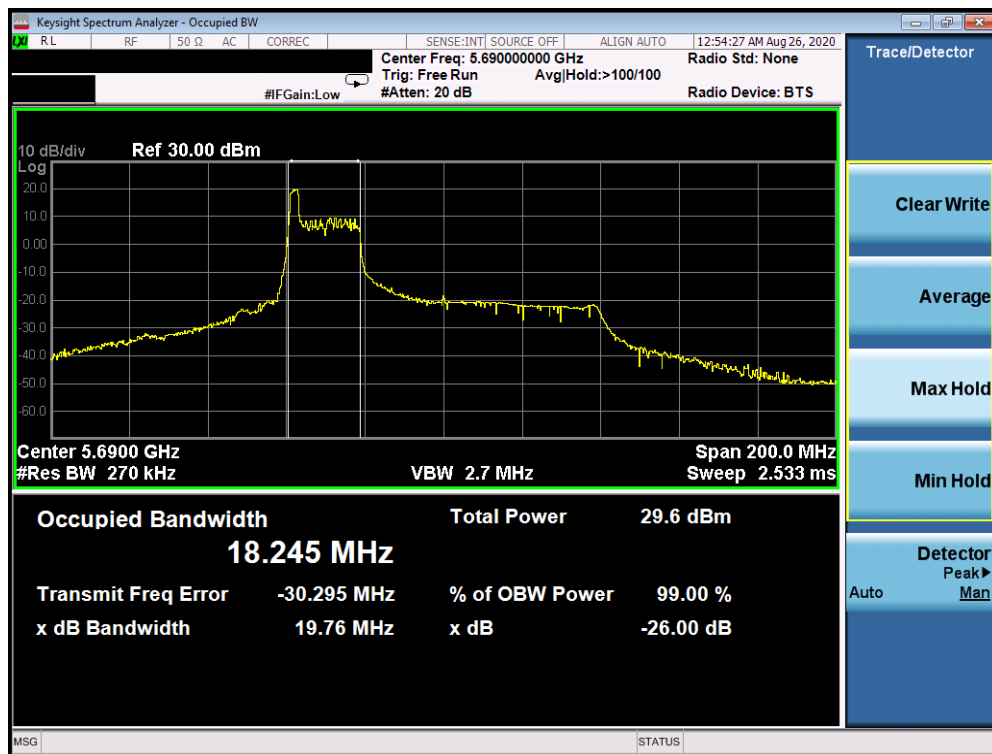
Plot 7-236. 26dB Bandwidth Plot Antenna 1b (80MHz BW 802.11ax Index 0 – RU26 (UNII Band 2C) – Ch. 138)
