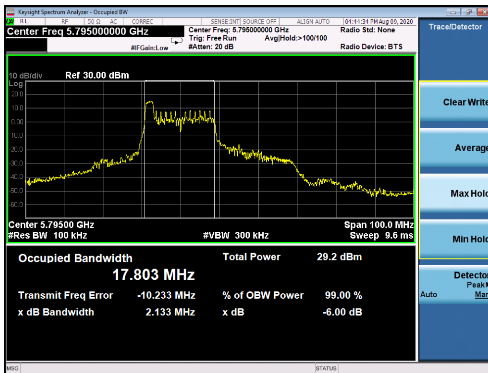
Plot 7-304. 6dB Bandwidth Plot Antenna 1b (40MHz BW 802.11ax Index 0 – RU26 (UNII Band 3) – Ch. 159)
