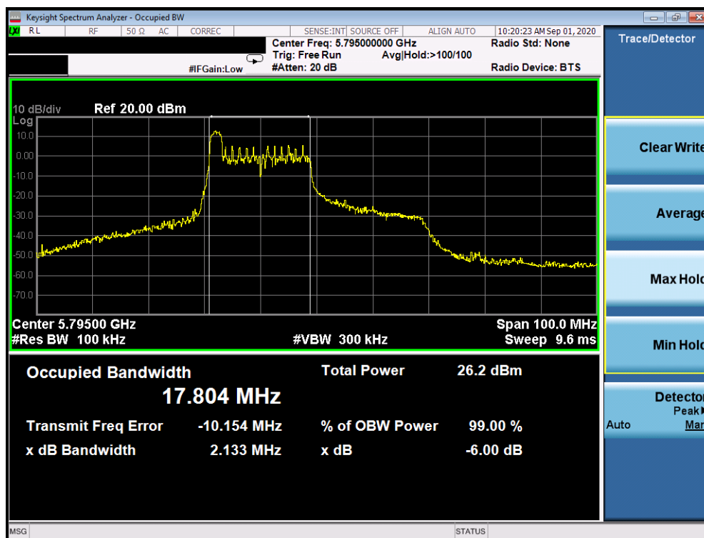
Plot 7-280. 6dB Bandwidth Plot Antenna 2a (40MHz BW 802.11ax Index 0 – RU26 (UNII Band 3) – Ch. 159)
