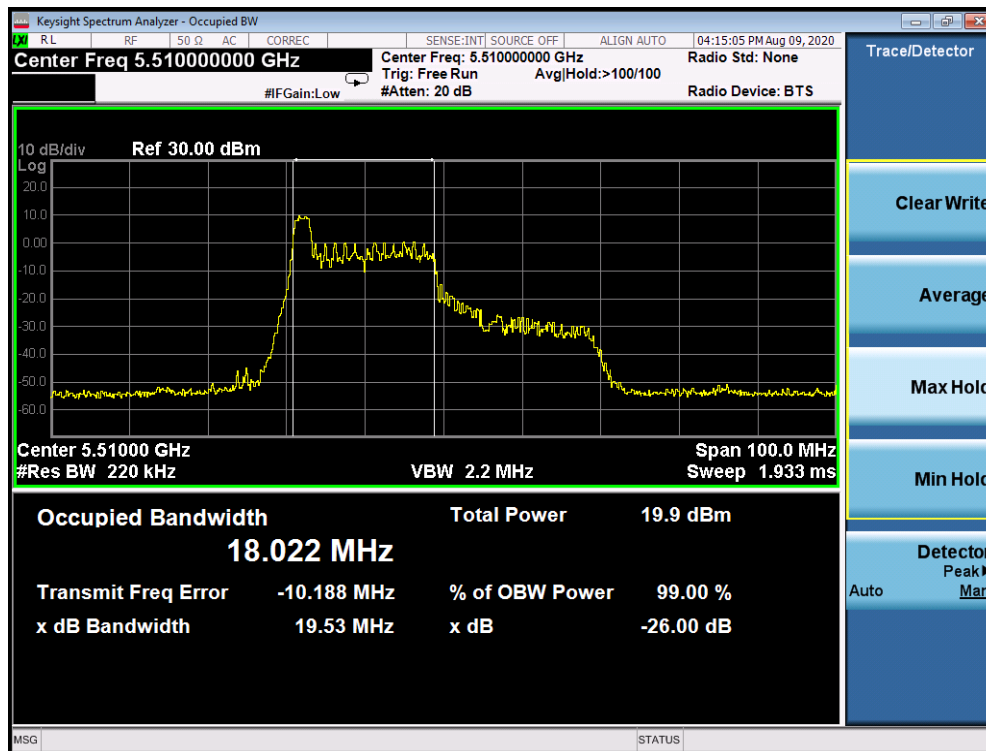
Plot 7-221. 26dB Bandwidth Plot Antenna 1b (40MHz BW 802.11ax Index 0 – RU26 (UNII Band 2C) – Ch. 102)
