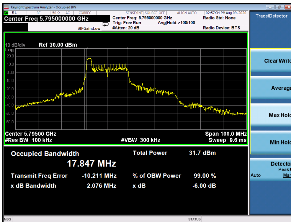
Plot 7-256. 6dB Bandwidth Plot Antenna 2b (40MHz BW 802.11ax Index 0 – RU26 (UNII Band 3) – Ch. 159)
