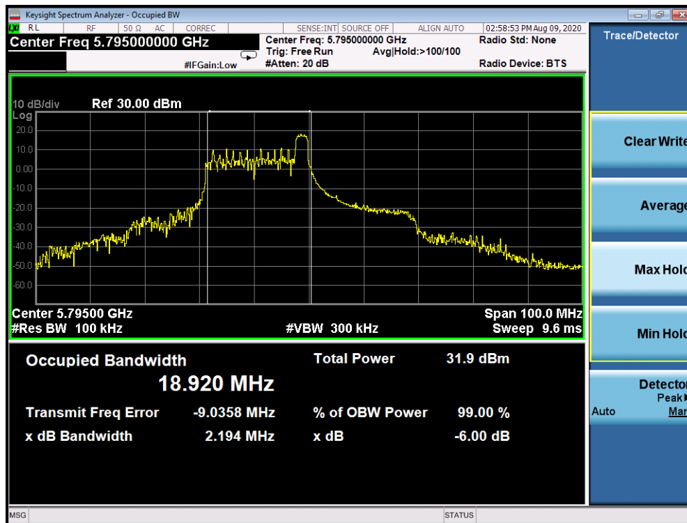
Plot 7-257. 6dB Bandwidth Plot Antenna 2b (40MHz BW 802.11ax Index 8 – RU26 (UNII Band 3) – Ch. 159)
