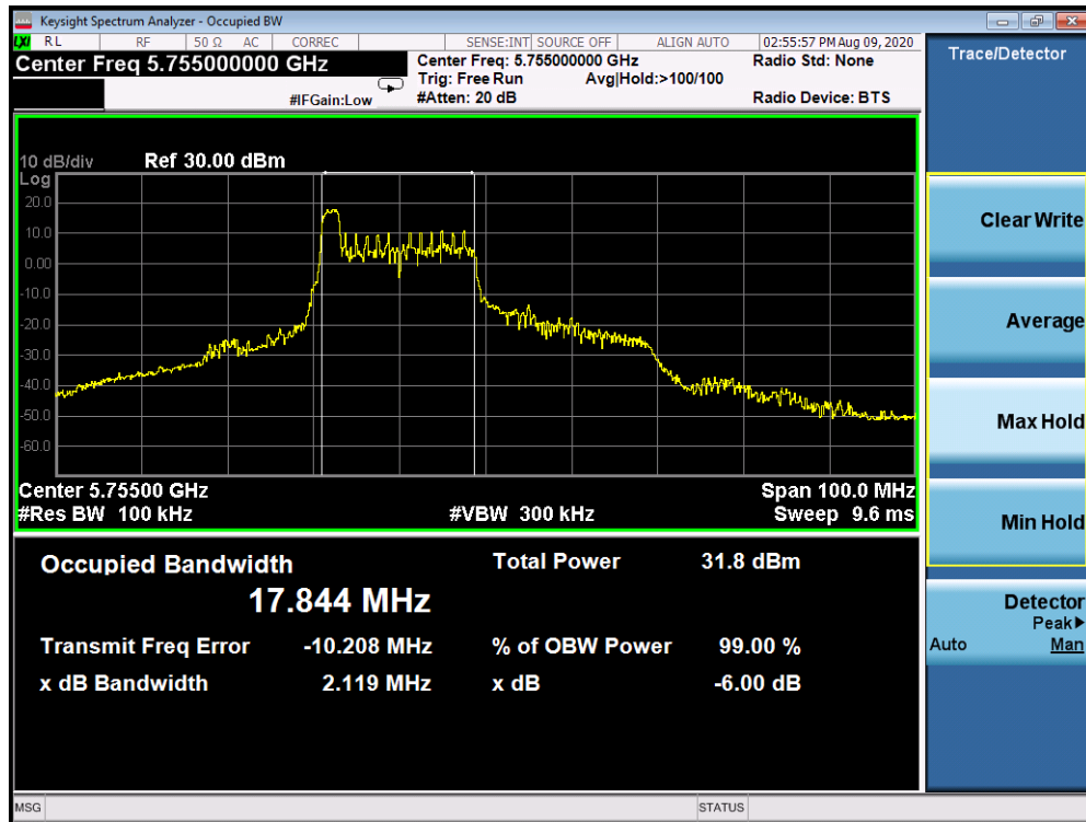
Plot 7-253. 6dB Bandwidth Plot Antenna 2b (40MHz BW 802.11ax Index 0 – RU26 (UNII Band 3) – Ch. 151)
