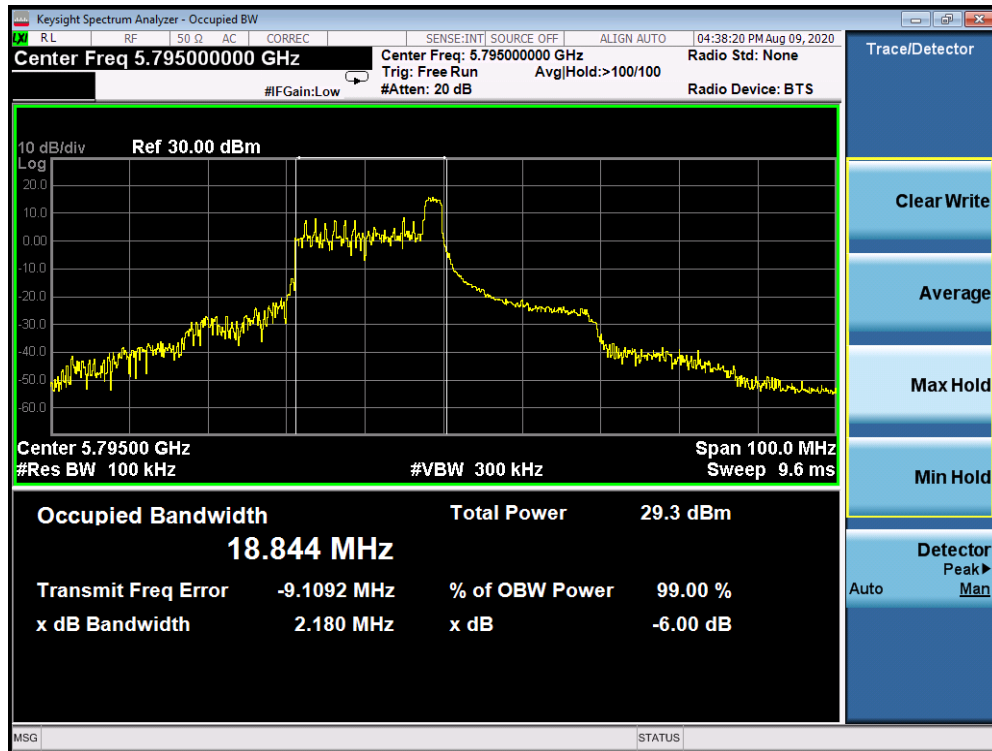
Plot 7-305. 6dB Bandwidth Plot Antenna 1b (40MHz BW 802.11ax Index 8 – RU26 (UNII Band 3) – Ch. 159)
