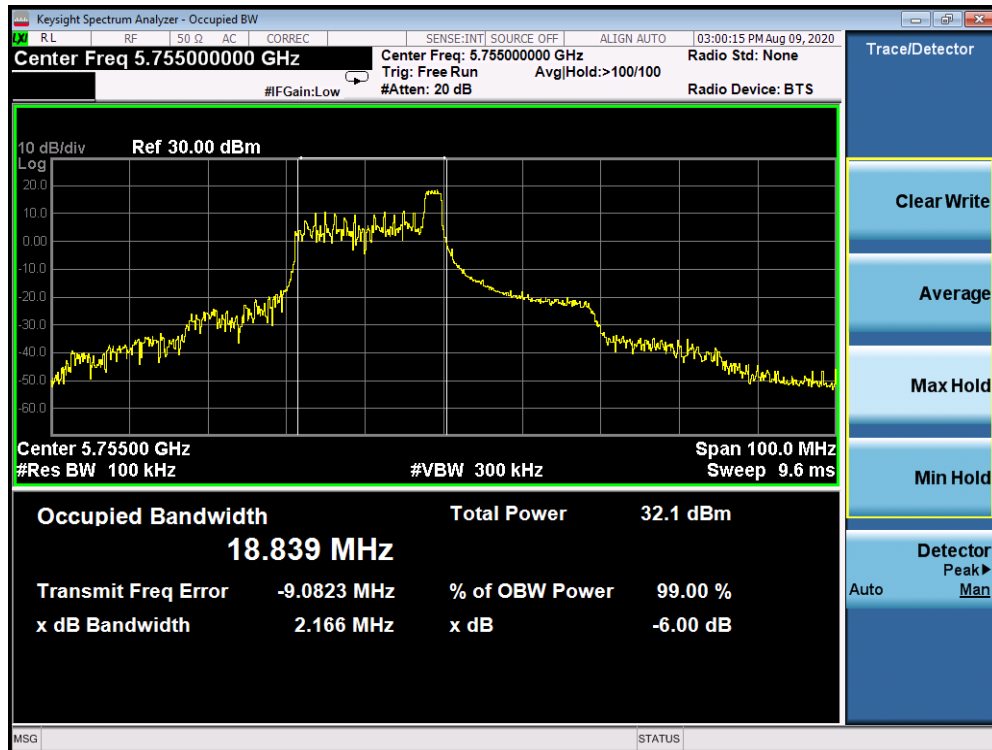
Plot 7-254. 6dB Bandwidth Plot Antenna 2b (40MHz BW 802.11ax Index 8 – RU26 (UNII Band 3) – Ch. 151)
