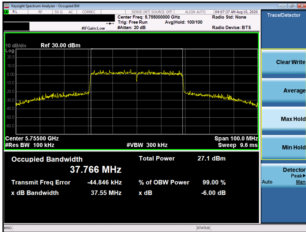
Plot 7-283. 6dB Bandwidth Plot Antenna 2a (40MHz BW 802.11ax – RU484 (UNII Band 3) – Ch. 151)
