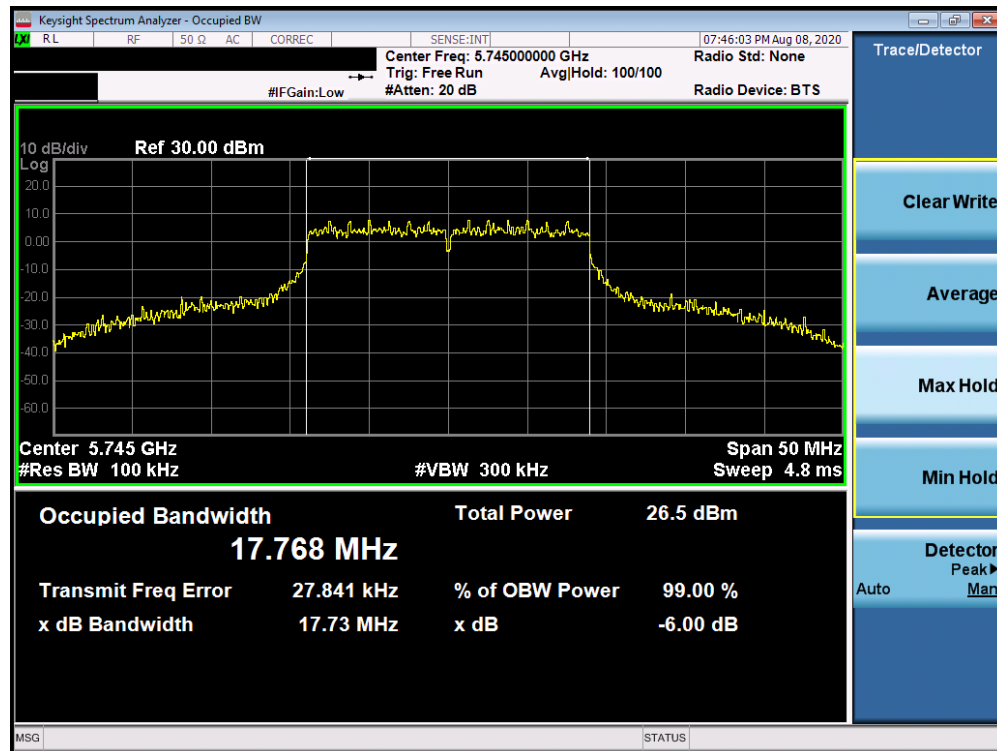
Plot 7-67. 6dB Bandwidth Plot Antenna 2a (20MHz BW 802.11n (UNII Band 3) – Ch. 149)
