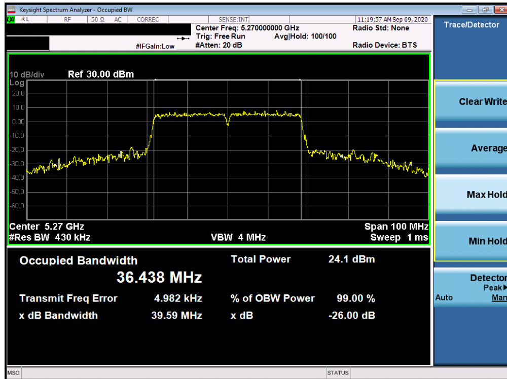
Plot 7-10. 26dB Bandwidth Plot Antenna 2b (40MHz BW 802.11n (UNII Band 2A) – Ch. 54)
