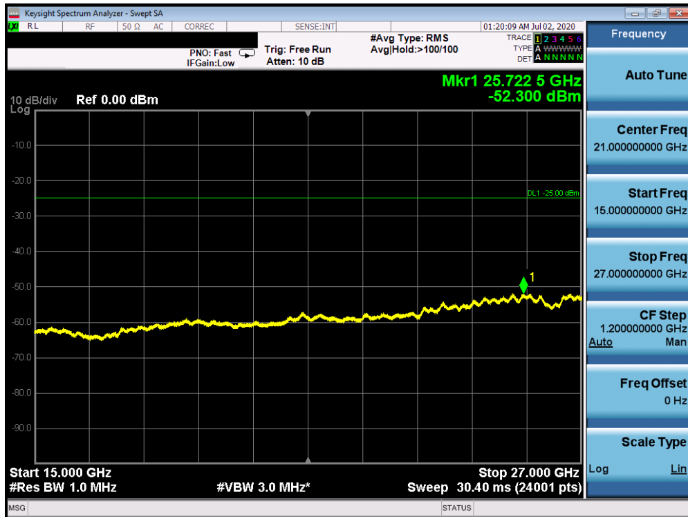
Plot 7-427. Conducted Spurious Plot (Band 7 – 20.0MHz QPSK – PCC 1/99 SCC 1/0 – Mid Channel)
