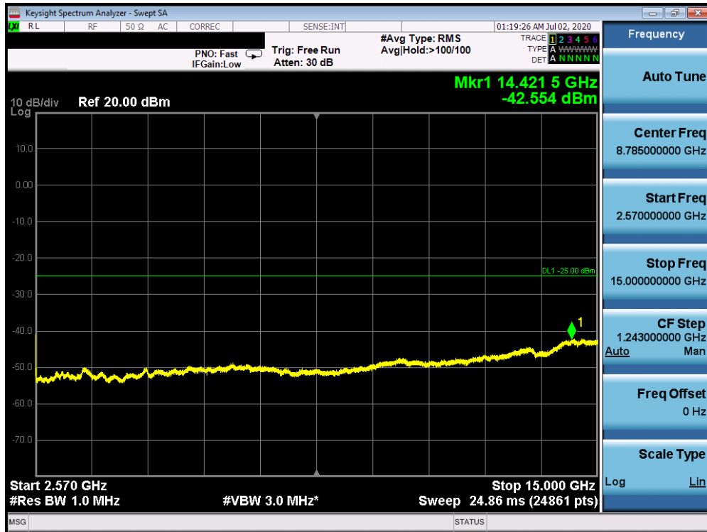
Plot 7-426. Conducted Spurious Plot (Band 7 – 20.0MHz QPSK – PCC 1/99 SCC 1/0 – Mid Channel)
