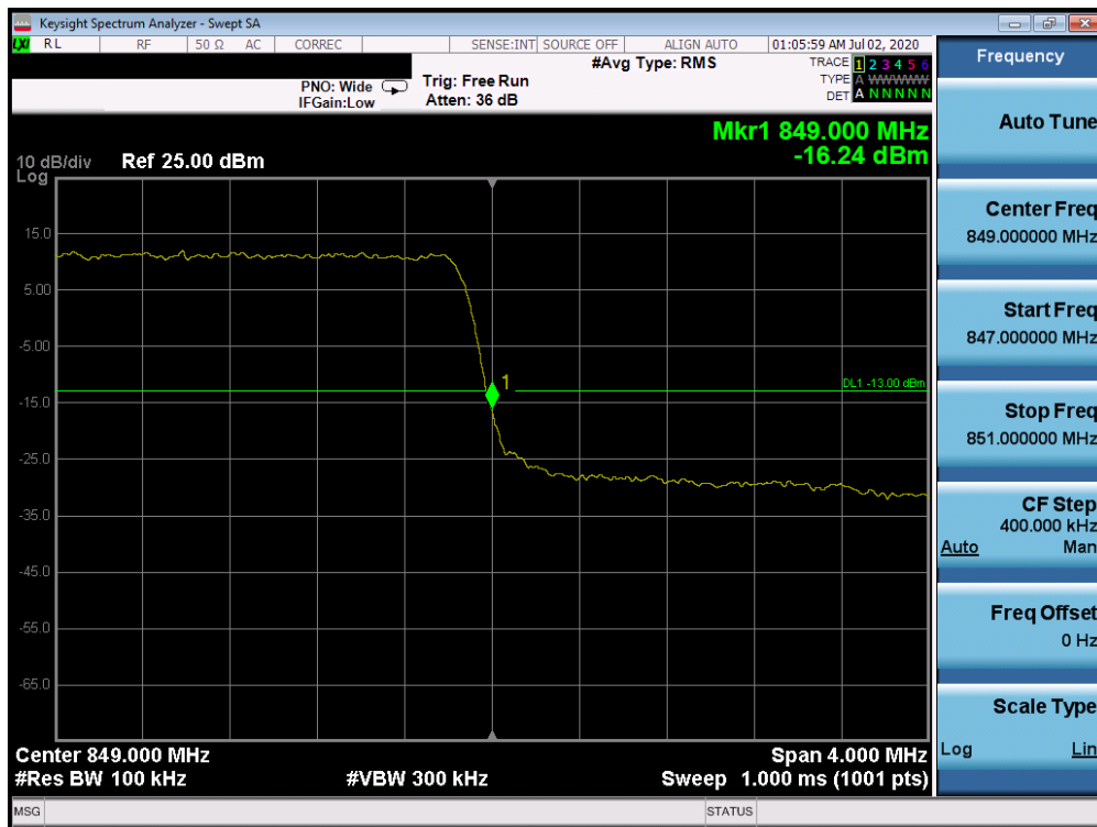
Plot 7-221. Upper Band Edge Plot (Band 26 - 3.0MHz QPSK - Full RB Configuration)
