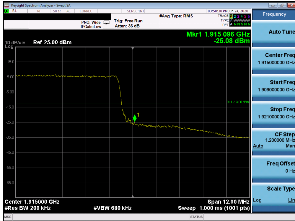
Plot 7-300. Upper Band Edge Plot (Band 25 - 15.0MHz QPSK - Full RB Configuration)
