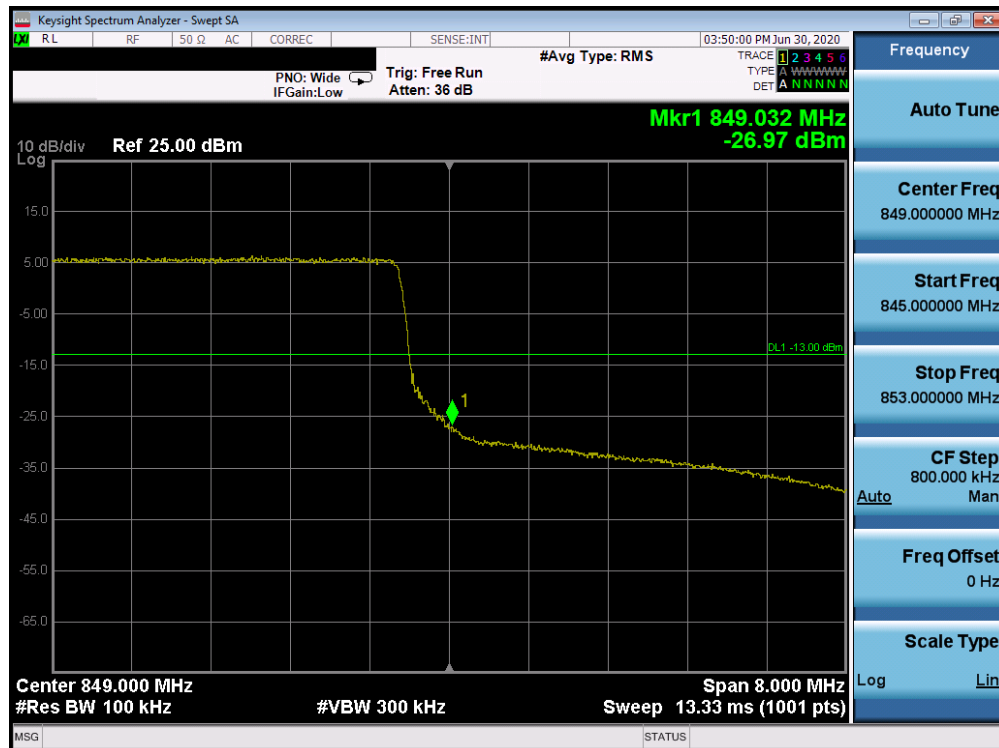
Plot 7-233. Upper Band Edge Plot (Band 5 - 10.0MHz QPSK - Full RB Configuration)
