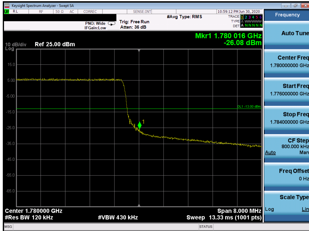
Plot 7-248. Upper Band Edge Plot (Band 66 - 10.0MHz QPSK - Full RB Configuration)
