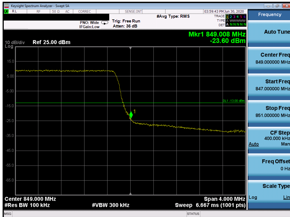
Plot 7-231. Upper Band Edge Plot (Band 5 - 5.0MHz QPSK - Full RB Configuration)
