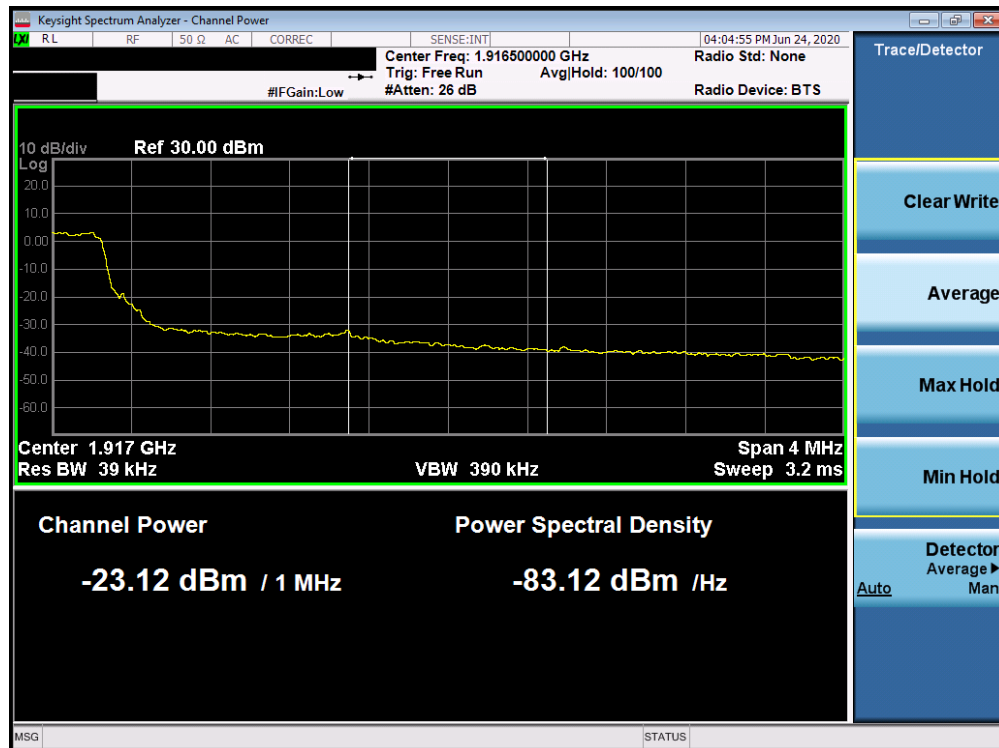
Plot 7-293. Upper Extended Band Edge Plot (Band 25 - 5.0MHz QPSK - Full RB Configuration)
