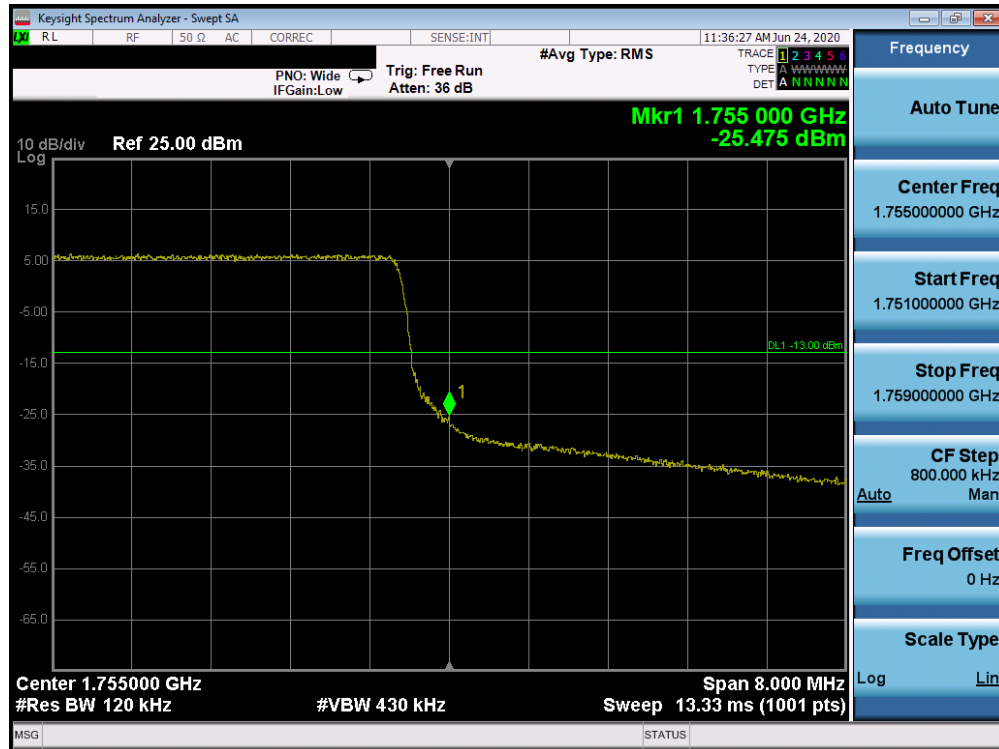
Plot 7-272. Upper Band Edge Plot (Band 4 - 10.0MHz QPSK - Full RB Configuration)
