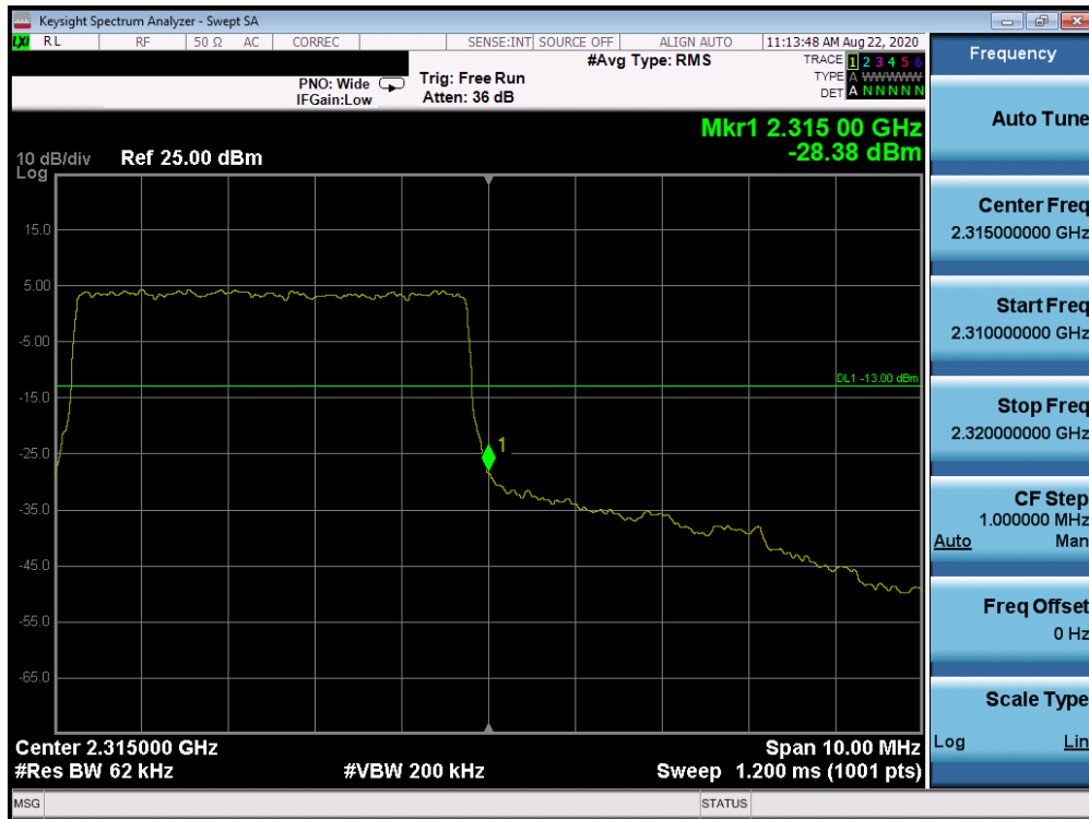
Plot 7-332. Upper Band Edge Plot (Band 30 - 5.0MHz QPSK - Full RB Configuration)
