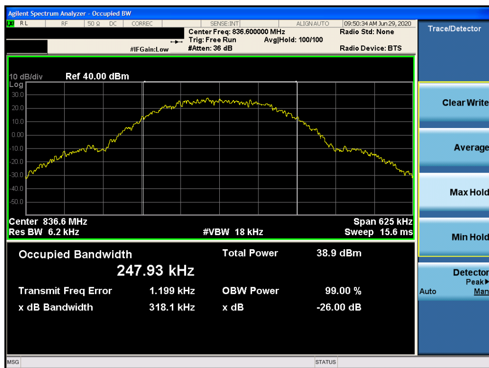
Plot 7-1. Occupied Bandwidth Plot (Cellular GPRS Mode)
