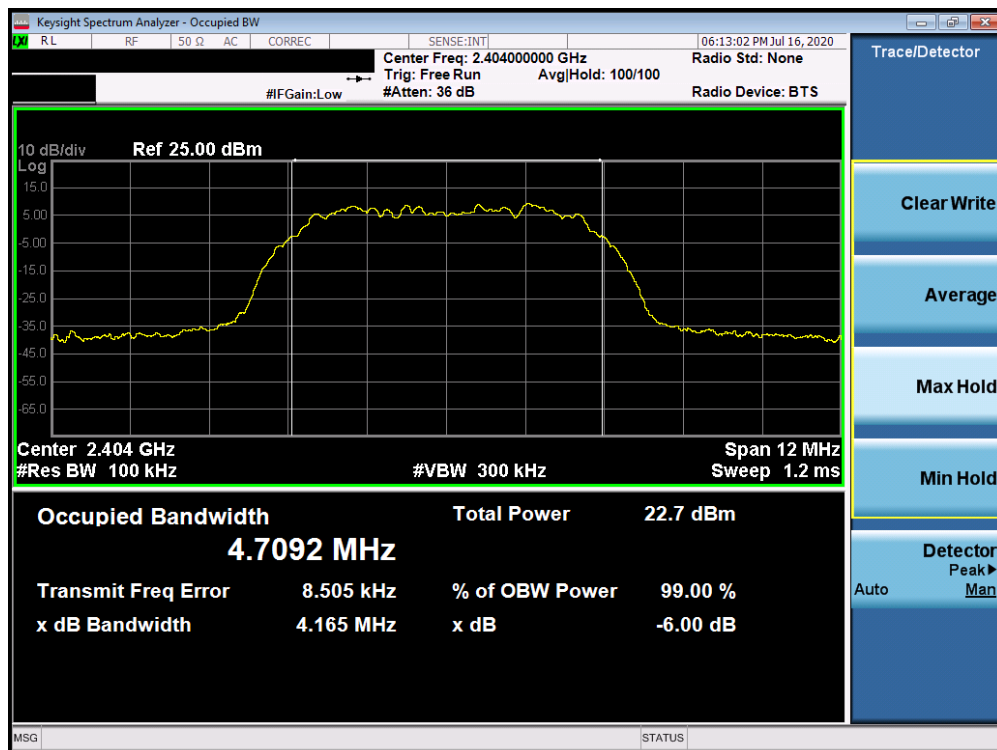
Plot 7-4. 6dB Bandwidth Plot Antenna WF8 (Bluetooth (HDR8), 8Mbps, ePA – Ch. 1)
