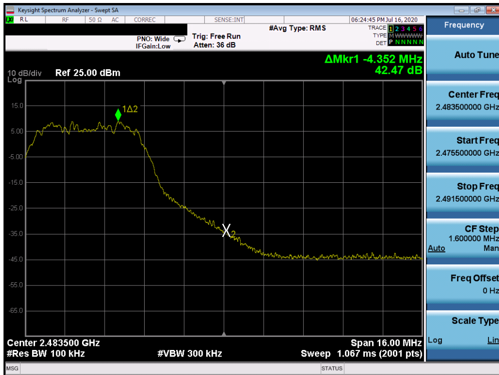
Plot 7-64. Band Edge Plot Antenna WF8 (Bluetooth (HDR8), ePA – Ch. 75)
