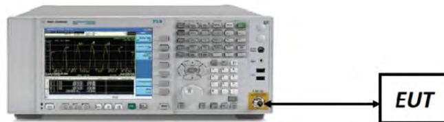
Figure 7-1. Test Instrument & Measurement Setup
