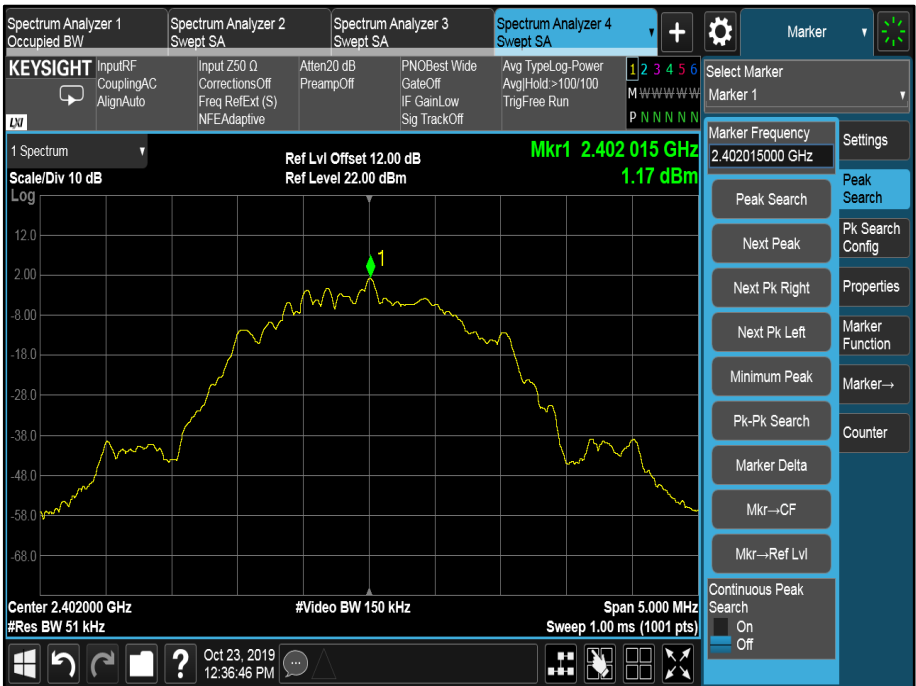
Figure 25 - 2402 MHz, Power Spectral Density
