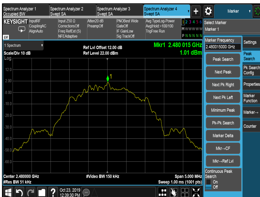
Figure 27 - 2480 MHz, Power Spectral Density
