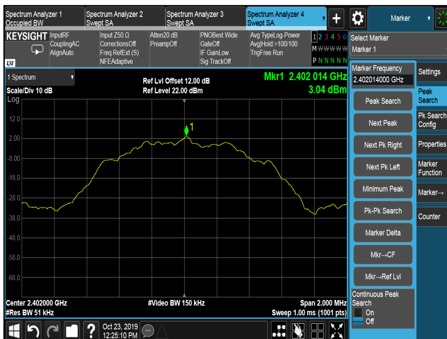
Figure 22 - 2402 MHz, Power Spectral Density
