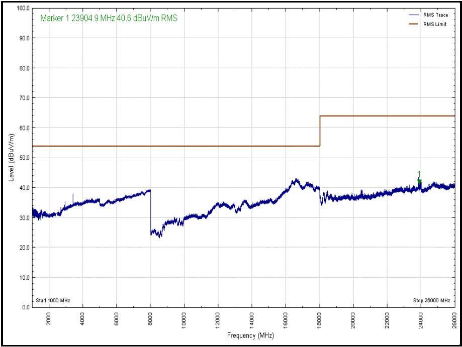
Figure 17 - 2440 MHz - 1 GHz to 26 GHz, Polarisation: Vertical (Average)
