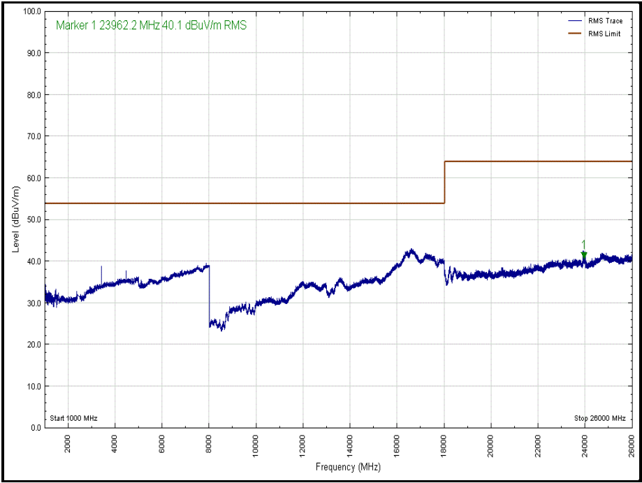
Figure 13 - 2402 MHz - 1 GHz to 26 GHz, Polarisation: Vertical (Average)
