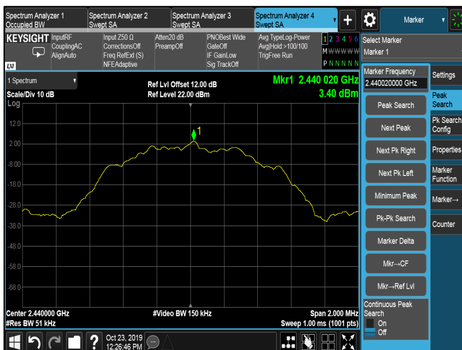
Figure 23 - 2440 MHz, Power Spectral Density
