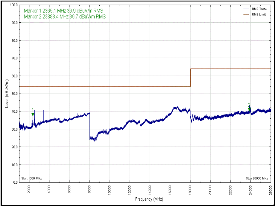
Figure 19 - 2480 MHz - 1 GHz to 26 GHz, Polarisation: Horizontal (Average)
