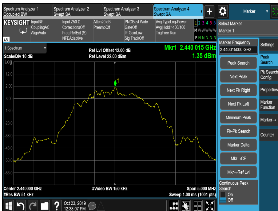
Figure 26 - 2440 MHz, Power Spectral Density
