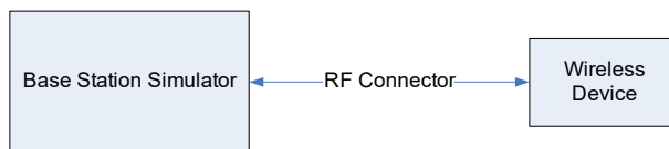
Figure 8-3 Power Measurement Setup
