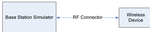
Figure 8-1 Power Measurement Setup
