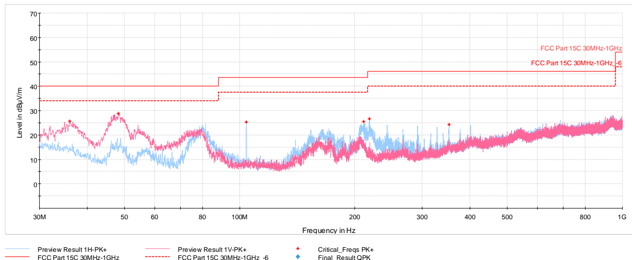
Plot 7-197. Radiated Spurious Emissions below 1GHz CDD Ch.1 (RU26), with AC/DC Adapter
