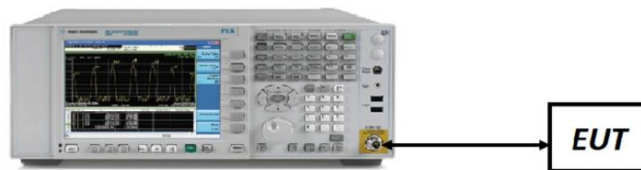
Figure 7-5. Test Instrument & Measurement Setup
