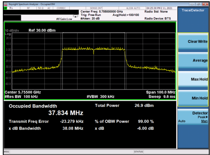
Plot 7-130. 6dB BW & 99% OBW Antenna 4b (40MHz BW 802.11ax(SU) – Ch. 151, MCS0)
