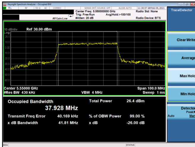
Plot 7-32. 26dB BW & 99% OBW Antenna 5b (40MHz BW 11ax – RU484 – Ch.110)
