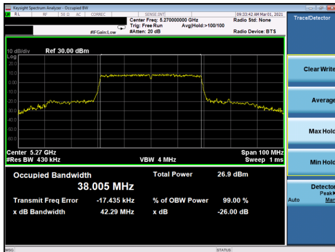
Plot 7-20. 26dB BW & 99% OBW Antenna 5b (40MHz BW 11ax – RU484 – Ch.54)
