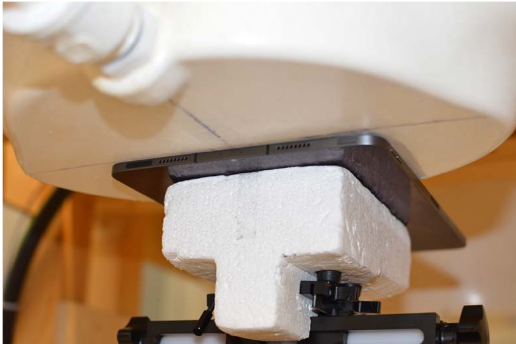
Test Setup Photo 7 – Back Side Antenna 3, 4a, and 4b SAR at 0 mm
