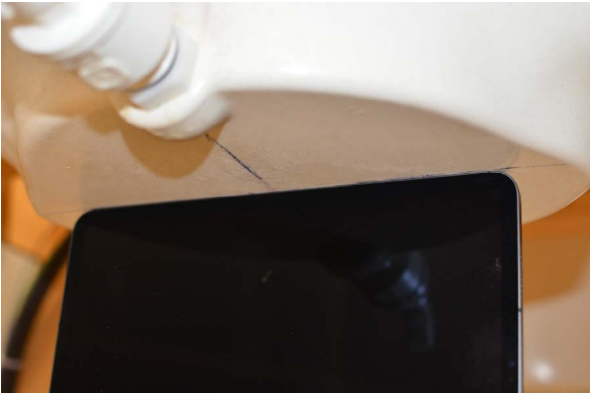
Test Setup Photo 9 – Left Edge SAR at 0 mm
