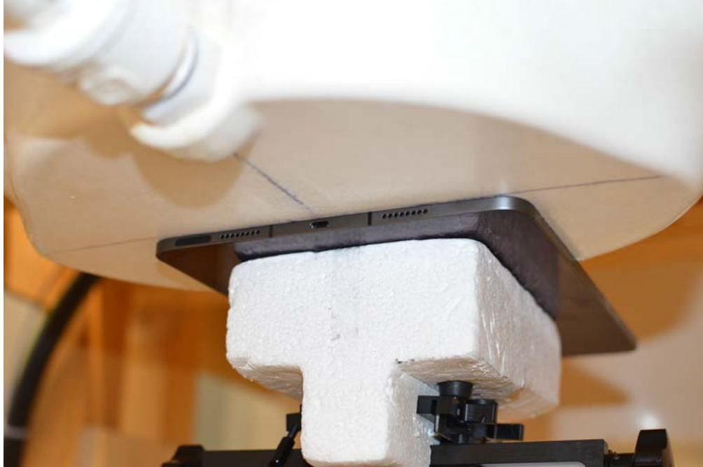
Test Setup Photo 6 – Back Side Antenna 1, 2a, and 2b SAR at 0 mm
