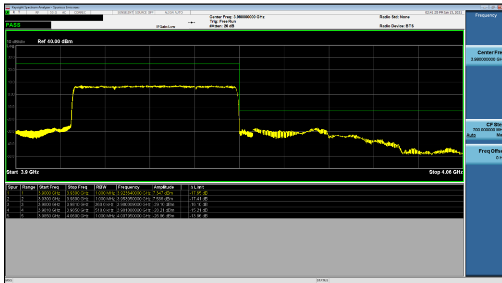
Plot 7-215. Upper ACP Plot (NR Band n77 - 60MHz DFT-s-OFDM \pi/2 BPSK – Full RB Configuration)
