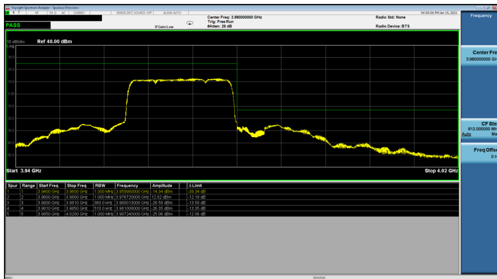
Plot 7-221. Upper ACP Plot (NR Band n77 - 20MHz DFT-s-OFDM \pi/2 BPSK – Full RB Configuration)
