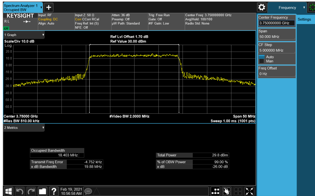
Plot 7-110. Occupied Bandwidth Plot (NR Band n77 - 20MHz CP-OFDM 256-QAM - Full RB Configuration)
