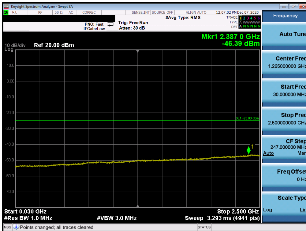
Plot 7-134. CSE (LTE Band 7 - 20MHz QPSK - RB Size 1, RB Offset 0 - High Channel)
