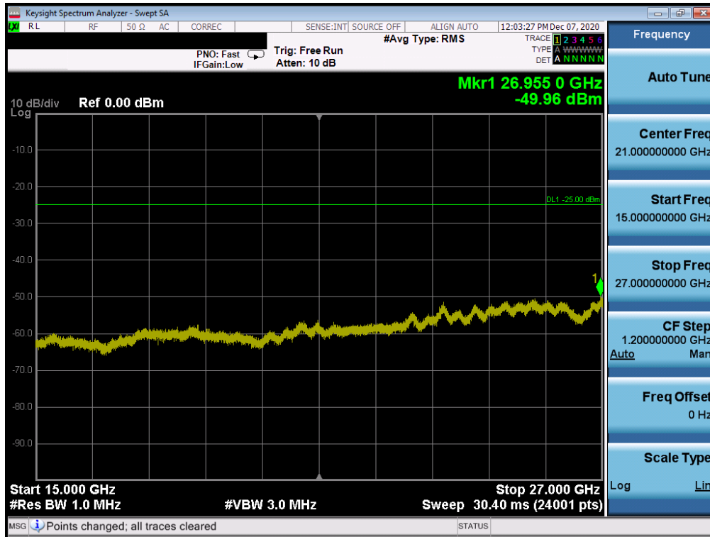
Plot 7-130. CSE (LTE Band 7 - 20MHz QPSK - RB Size 1, RB Offset 0 - Low Channel)
