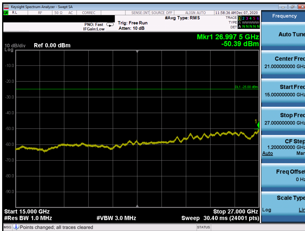
Plot 7-133. CSE (LTE Band 7 - 20MHz QPSK - RB Size 1, RB Offset 0 - Mid Channel)
