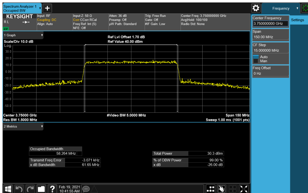
Plot 7-95. Occupied Bandwidth Plot (NR Band n77 - 60MHz CP-OFDM 256-QAM - Full RB Configuration)
