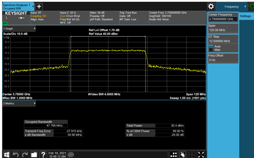
Plot 7-100. Occupied Bandwidth Plot (NR Band n77 - 50MHz CP-OFDM 256-QAM - Full RB Configuration)
