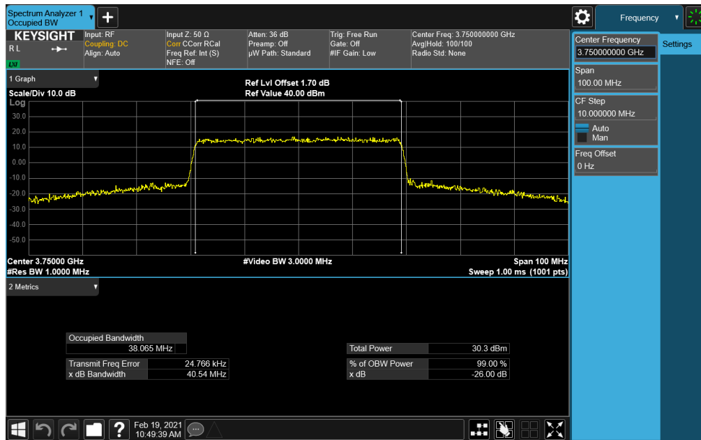
Plot 7-105. Occupied Bandwidth Plot (NR Band n77 - 40MHz CP-OFDM 256-QAM - Full RB Configuration)
