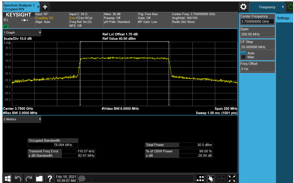
Plot 7-90. Occupied Bandwidth Plot (NR Band n77 - 80MHz CP-OFDM 256-QAM - Full RB Configuration)
