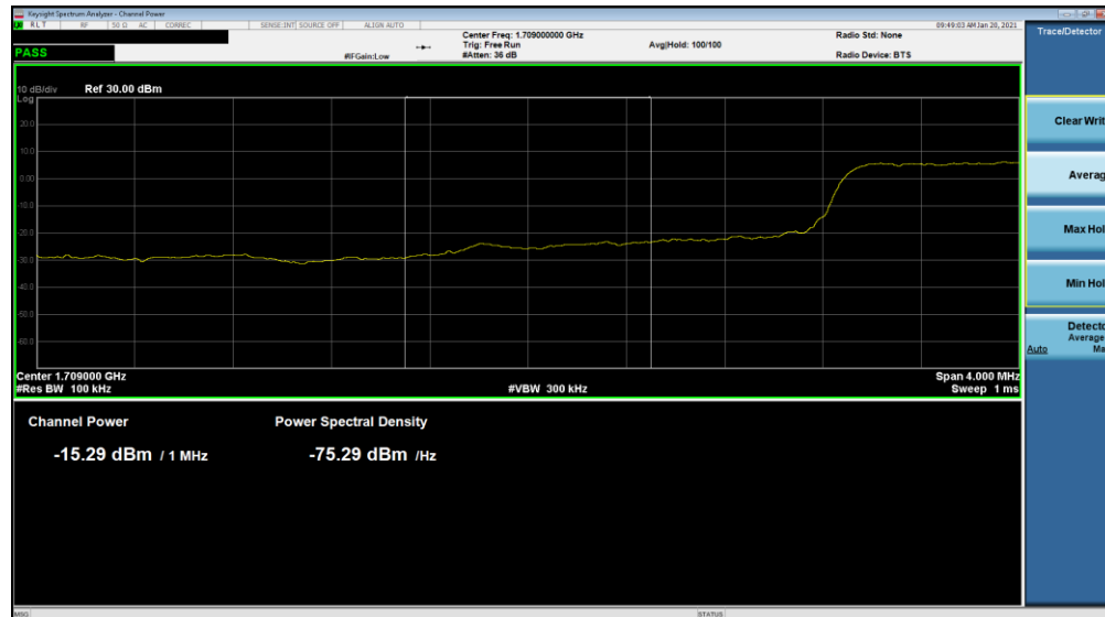
Plot 7-272. Lower Extended Band Edge Plot (NR Band n66 - 10.0MHz DFT-s OFDM \pi/2 BPSK - Full RB Configuration)
