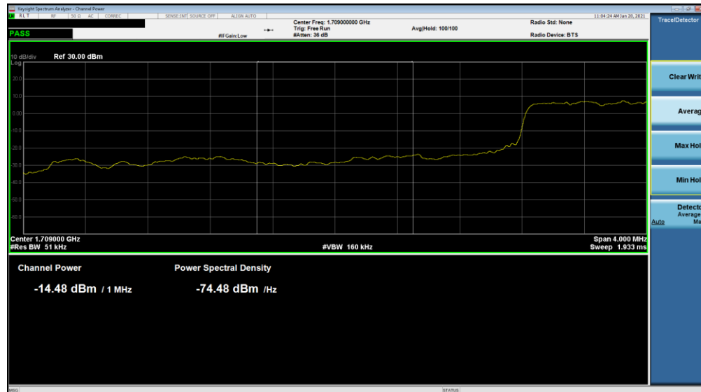
Plot 7-276. Lower Extended Band Edge Plot (NR Band n66 - 5.0MHz DFT-s OFDM \pi/2 BPSK - Full RB Configuration)
