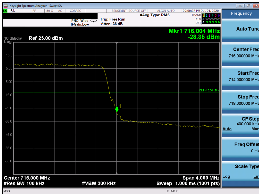
Plot 7-238. Upper Band Edge Plot (Band 12 - 5.0MHz QPSK - Full RB Configuration)
