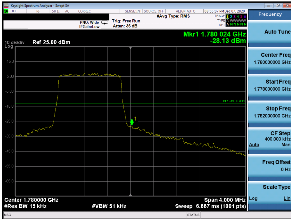
Plot 7-233. Upper Band Edge Plot (Band 66 - 1.4MHz QPSK - Full RB Configuration)
