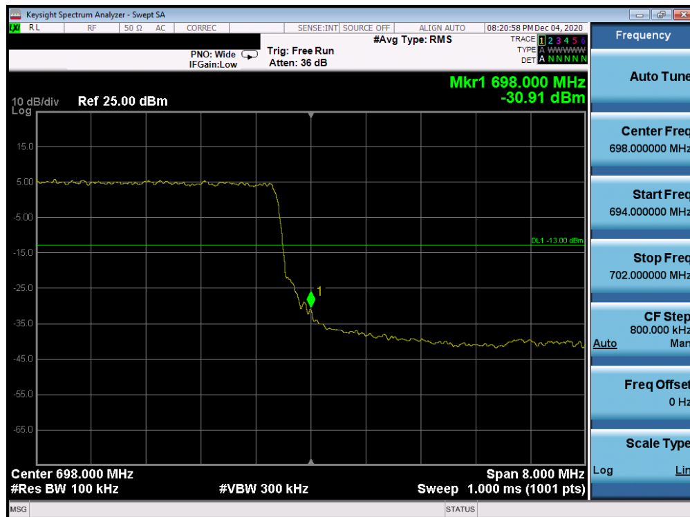
Plot 7-260. Upper Band Edge Plot (Band 71 - 10.0MHz QPSK - Full RB Configuration)
