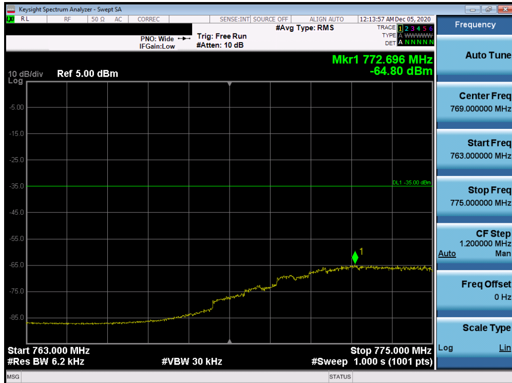
Plot 7-248. Lower Emission Mask Edge Plot (Band 13 - 10.0MHz QPSK - Full RB Configuration)
