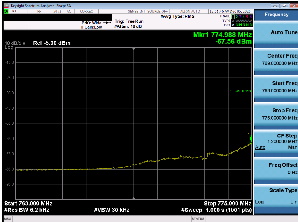
Plot 7-252. Lower Emission Mask Edge Plot (Band 13 - 5.0MHz QPSK - Full RB Configuration)
