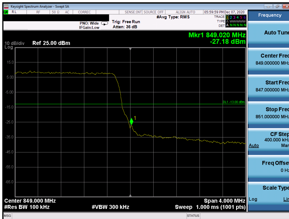
Plot 7-97. Upper Band Edge Plot (LTE Band 26 - 5MHz QPSK – Full RB Configuration)
