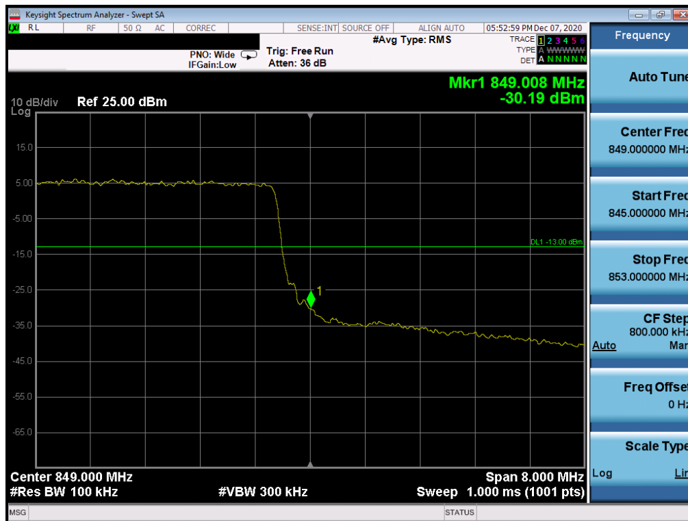
Plot 7-95. Upper Band Edge Plot (LTE Band 26 - 10MHz QPSK – Full RB Configuration)
