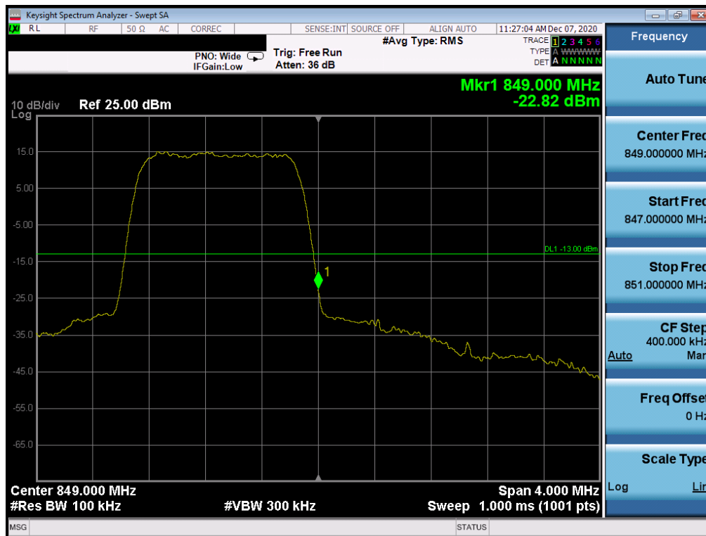
Plot 7-93. Upper Band Edge Plot (LTE Band 5 – 1.4MHz QPSK – Full RB Configuration)
