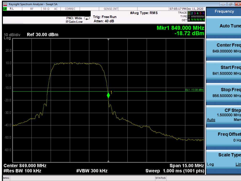
Plot 7-115. Upper Band Edge Plot (WCDMA Cell – Ch. 4233)
