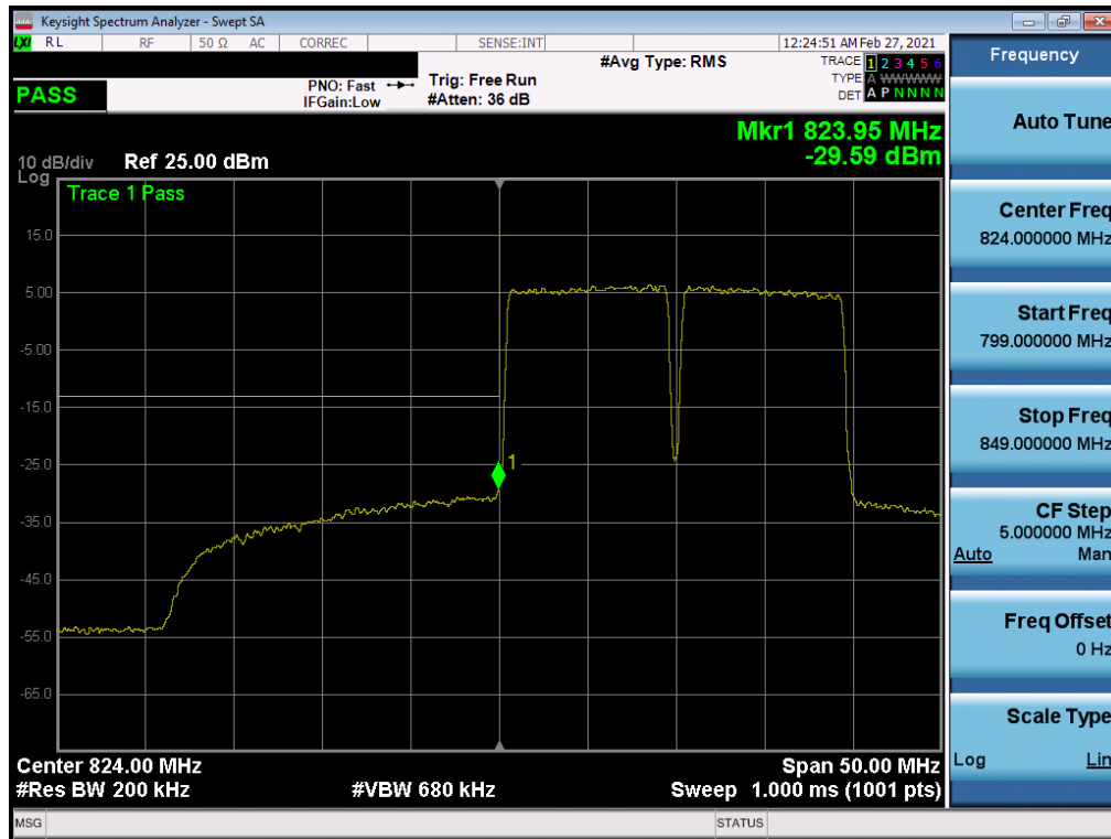
Plot 7-110. Lower BE Plot (ULCA LTE Band 5 - (10 + 10)MHz QPSK – Full RB Configuration)
