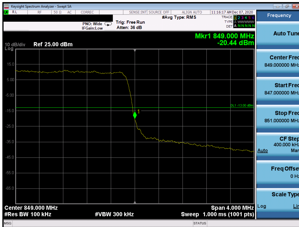
Plot 7-91. Upper Band Edge Plot (LTE Band 5 - 3MHz QPSK – Full RB Configuration)
