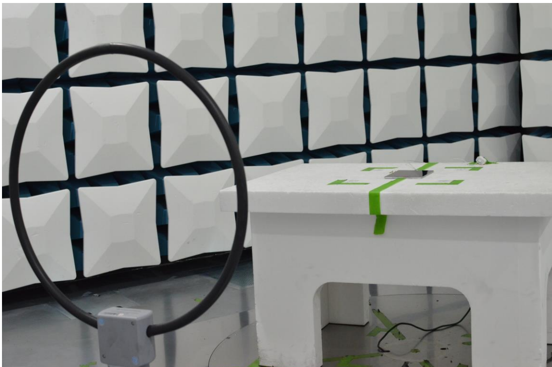
Figure 24: 9kHz-30MHz Test Setup (Front View)
