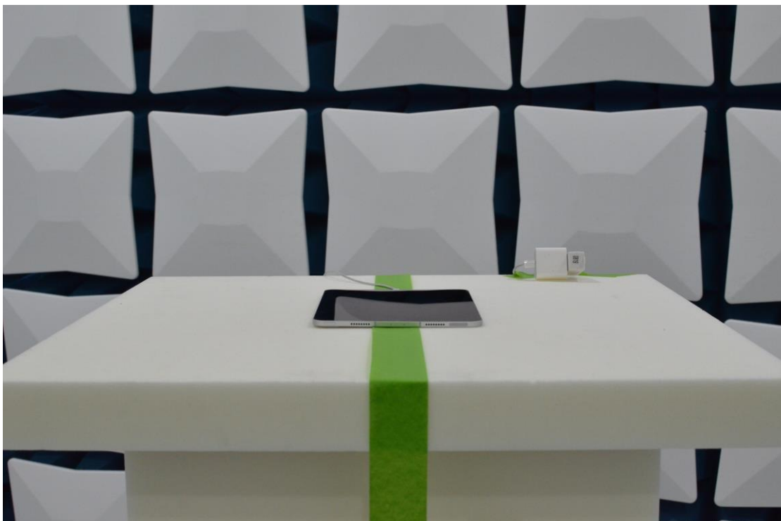
Figure 6: 1-18GHz Test Setup (Front View)
