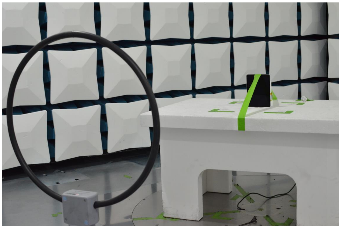
Figure 26: 9kHz-30MHz Test Setup (Front View)
