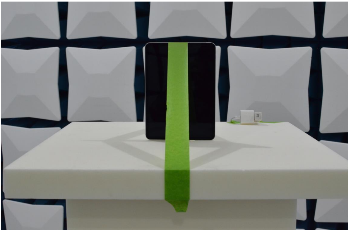
Figure 10: 1-18GHz Test Setup (Front View)
