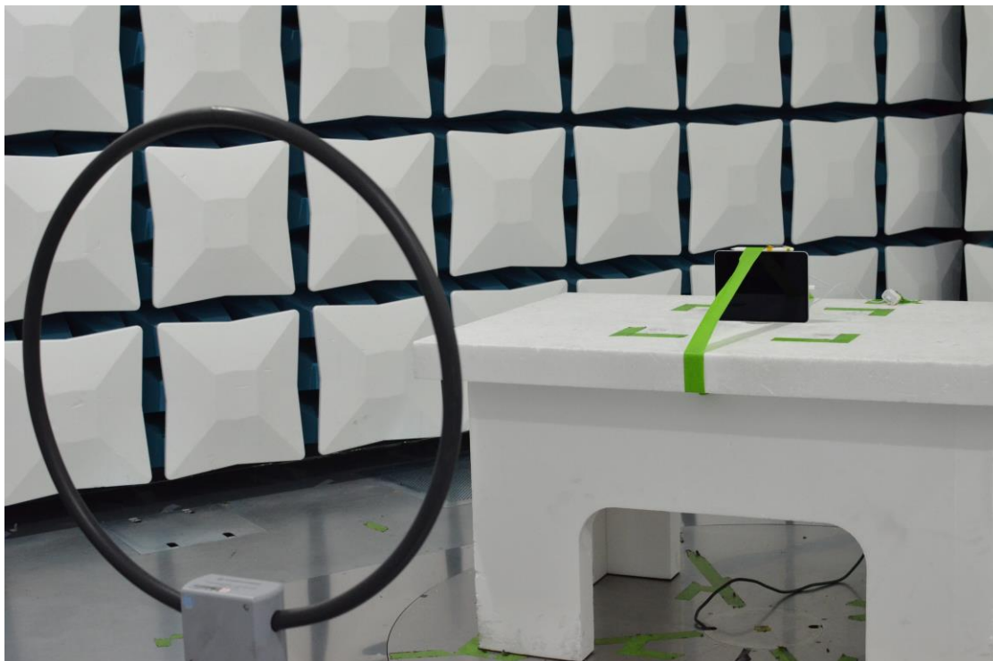
Figure 25: 9kHz-30MHz Test Setup (Front View)
