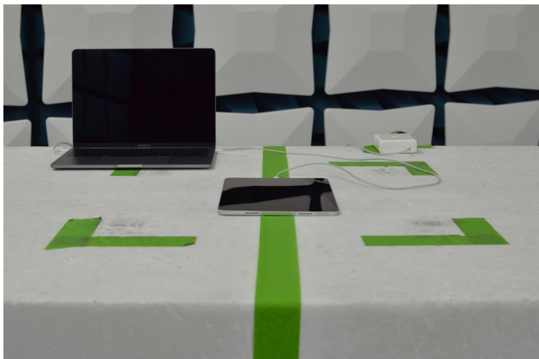
Figure 18: 30MHz-1GHz Test Setup (Front View)
