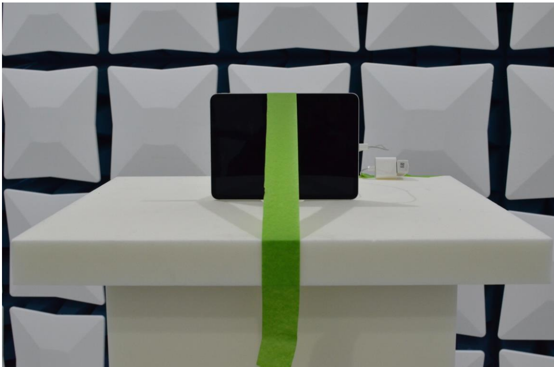
Figure 8: 1-18GHz Test Setup (Front View)
