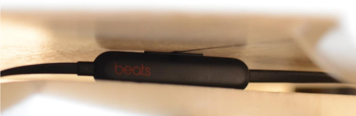
SAR Test Setup Photo 4: Extremity Exposure condition Edge 1 (Button touching)
