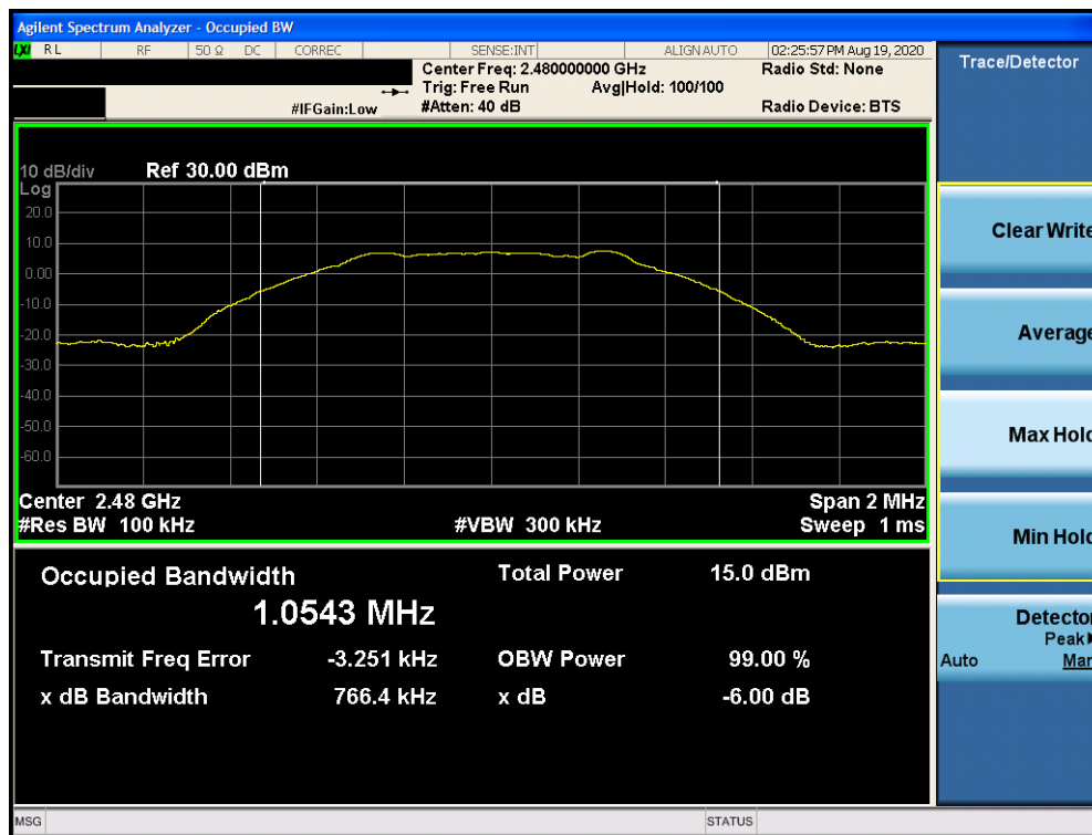
Plot 7-3. 6dB Bandwidth Plot (Bluetooth (LE), 1Mbps, iPA – Ch. 39)
