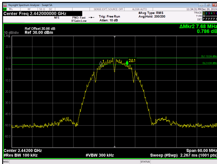
Figure 9 - 2442 MHz - 6 dB DTS Bandwidth
