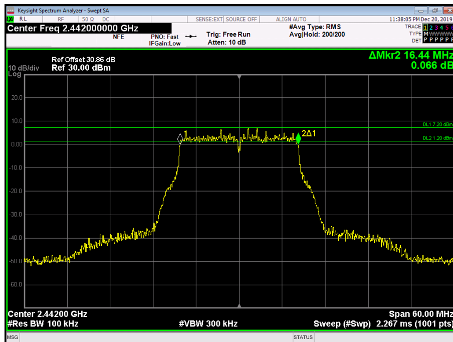
Figure 21 - 2442 MHz - 6 dB DTS Bandwidth
