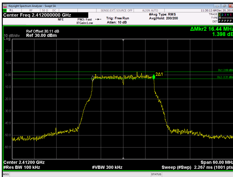
Figure 19 - 2412 MHz - 6 dB DTS Bandwidth
