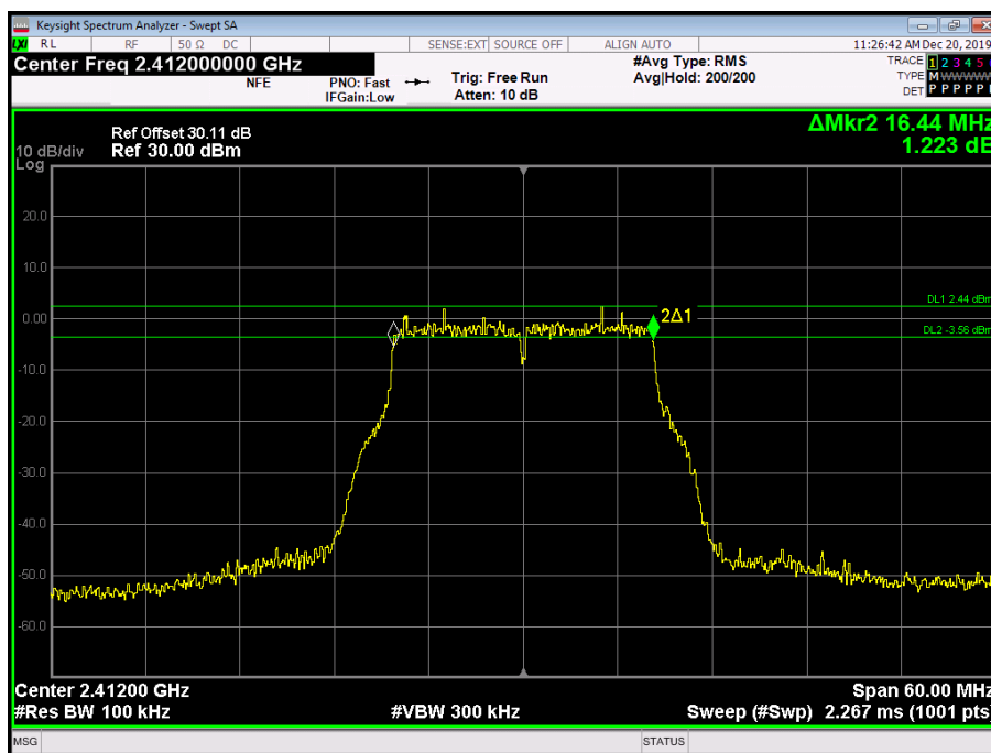
Figure 13 - 2412 MHz - 6 dB DTS Bandwidth
