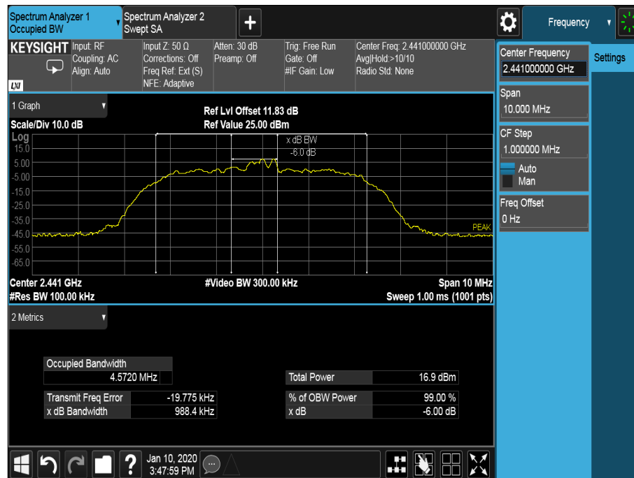
Figure 35 – 2441 MHz – Emission Bandwidth
