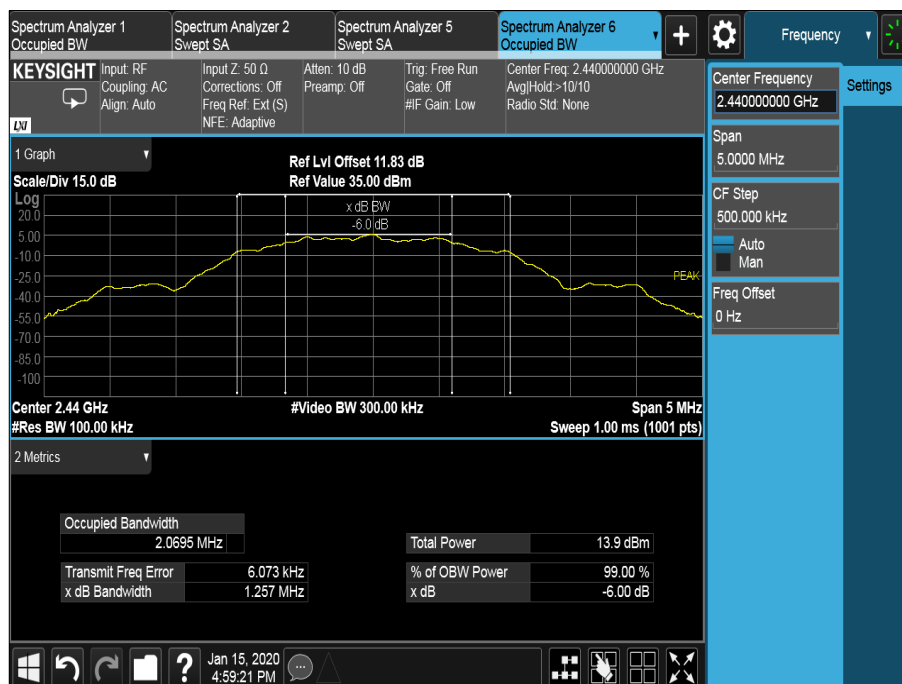
Figure 23 - 2440 MHz – Emission Bandwidth
