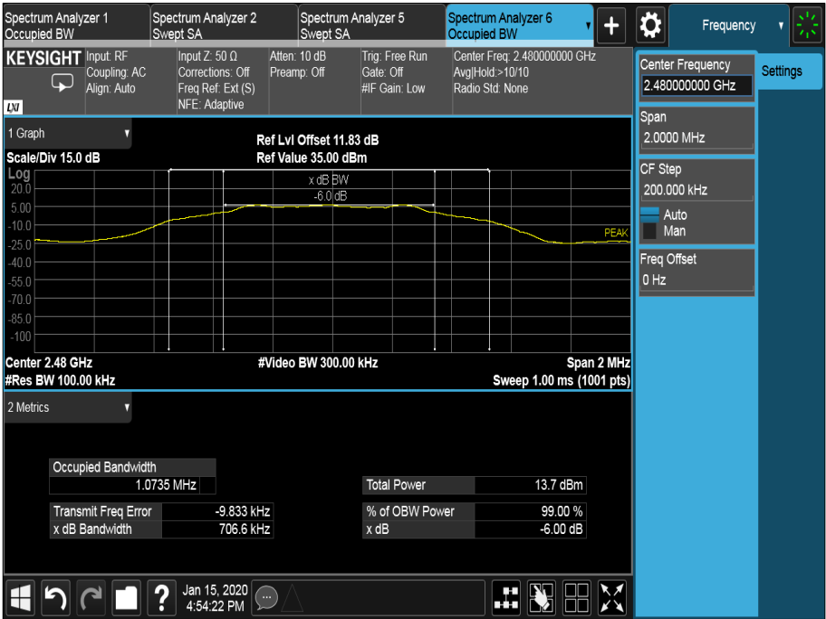
Figure 21 - 2480 MHz – Emission Bandwidth
