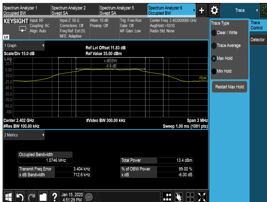
Figure 19 - 2402 MHz – Emission Bandwidth
