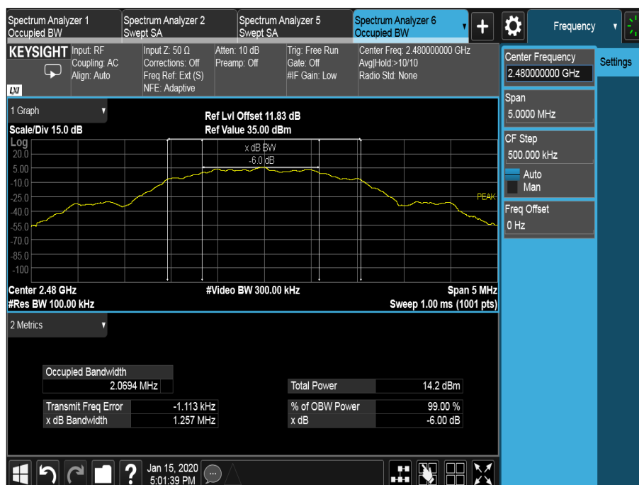
Figure 24 - 2480 MHz – Emission Bandwidth
