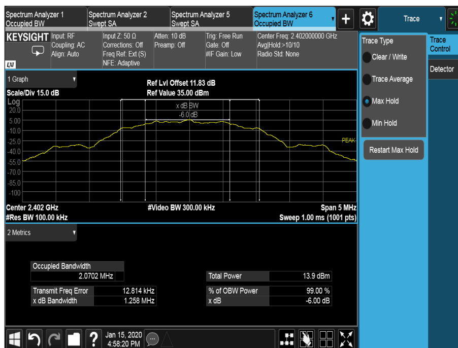
Figure 22 - 2402 MHz – Emission Bandwidth
