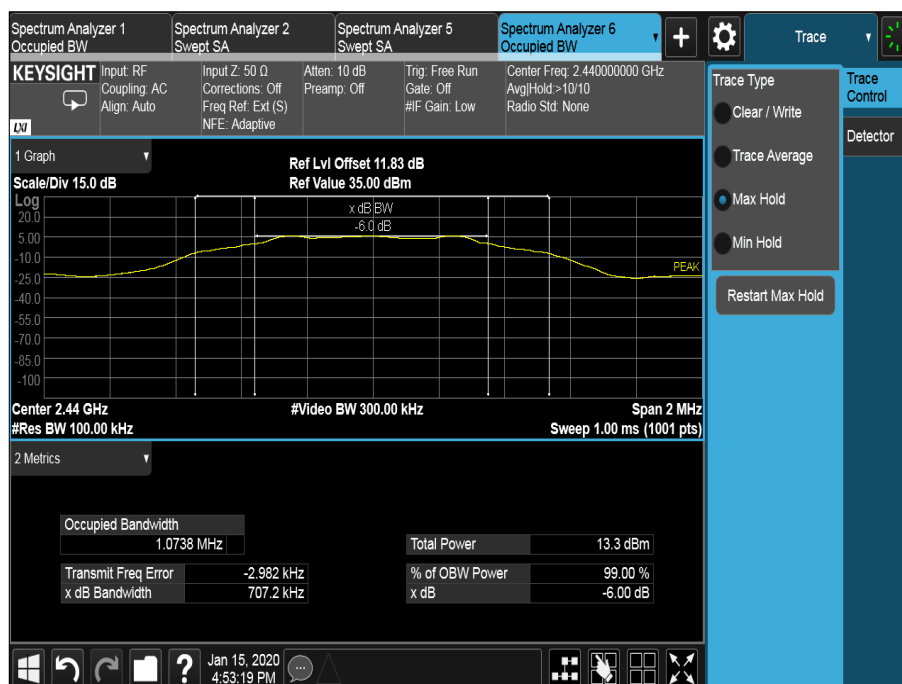
Figure 20 - 2440 MHz – Emission Bandwidth
