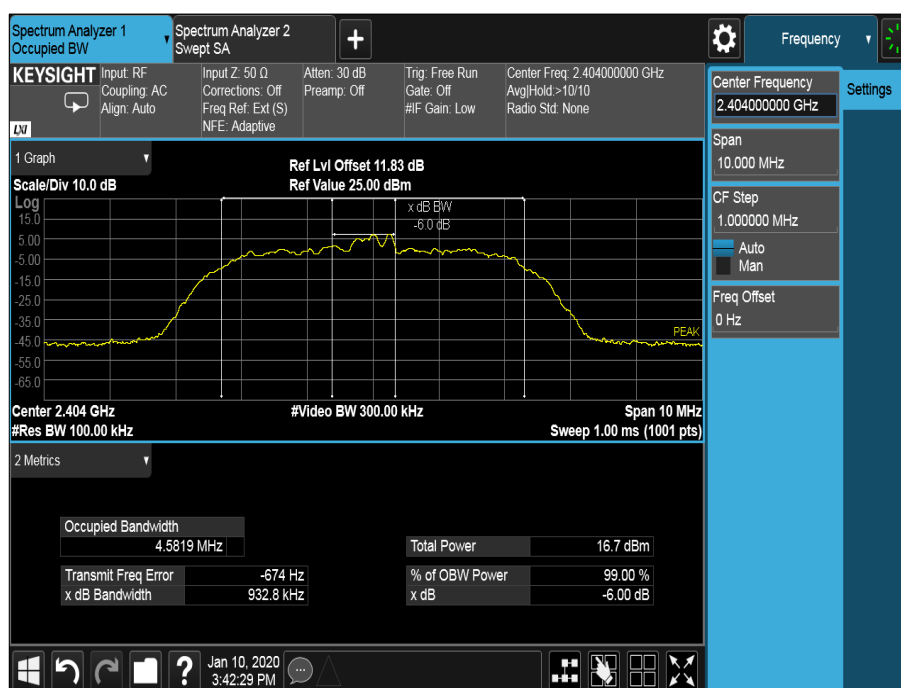
Figure 34 - 2404 MHz – Emission Bandwidth
