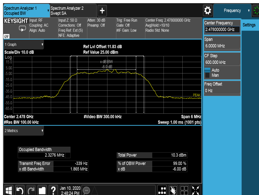
Figure 27 - 2478 MHz – Emission Bandwidth
